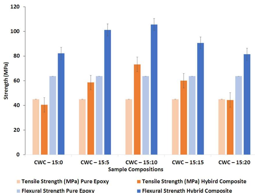
Fig. 5 Tensile and flexural strength ratings for hybrid bio-composites and produced pure epoxy samples.
