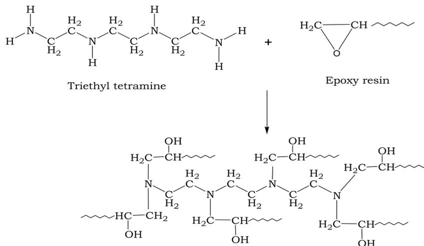
Scheme 1 Interaction between triethylenetetramine and epoxy resin.
