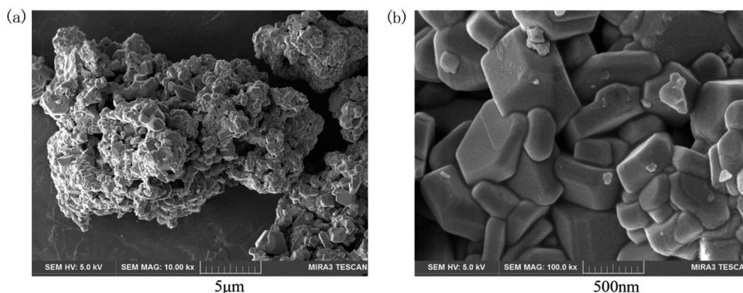
Fig. 2 SEM images of KGP:Bi<sup>3+</sup>,Sm<sup>3+</sup> phosphor.
