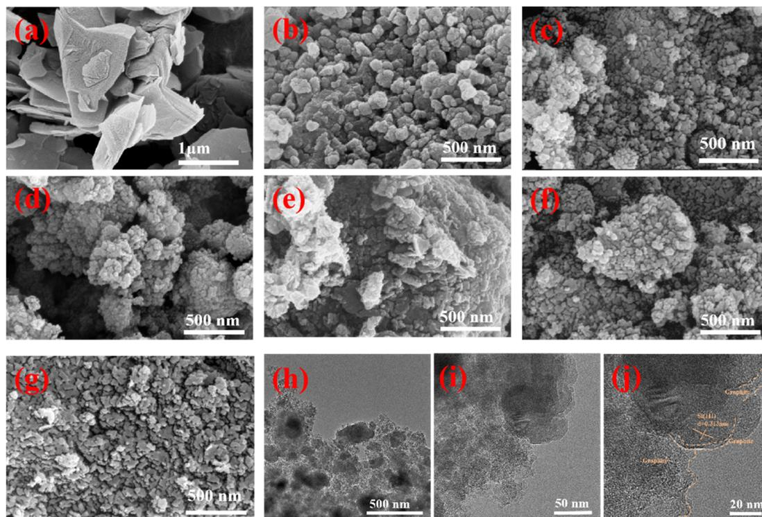
Fig. 3 SEM morphology of (a) graphite, (b) Si, (c) Si<sub>50</sub>G<sub>50</sub>, (d) Si<sub>40</sub>G<sub>60</sub>, (e) Si<sub>30</sub>G<sub>70</sub>, (f) Si<sub>20</sub>G<sub>80</sub>, and (g) Si<sub>10</sub>G<sub>90</sub>. TEM (h and i) and HRTEM (j) images of Si<sub>20</sub>G<sub>80</sub> composites.
