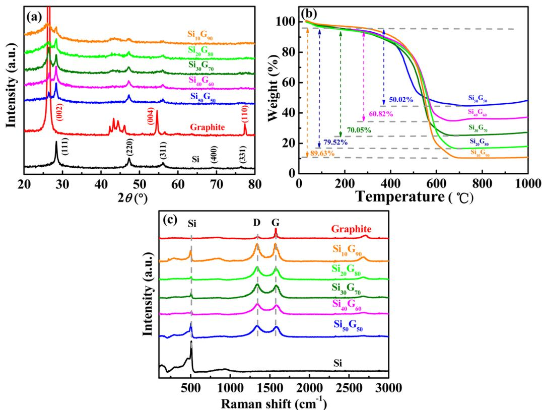
Fig. 2 (a) XRD spectra, (b) TG curves, and (c) Raman spectrum of Si/graphite composites with different mass ratios.
