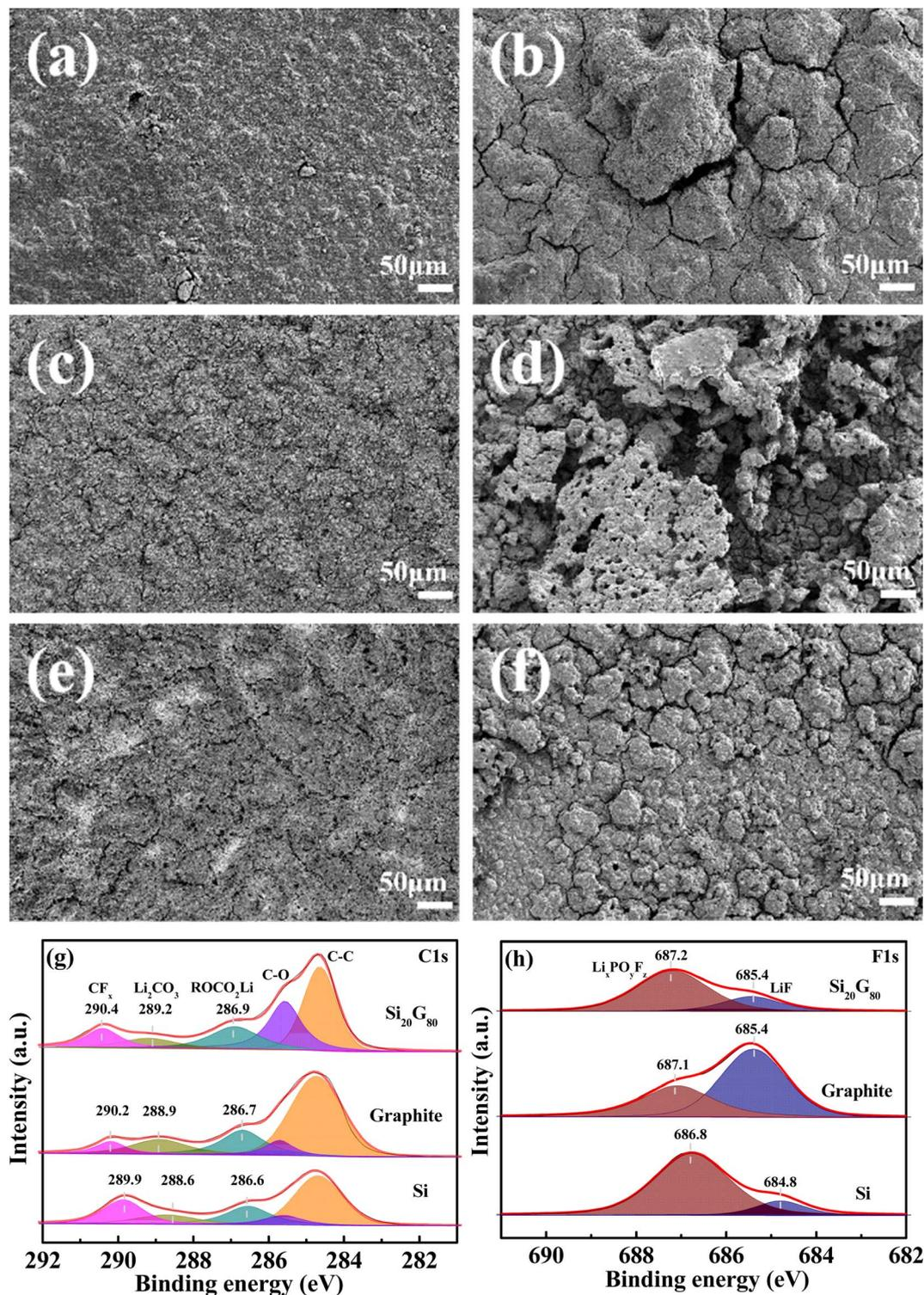
Fig. 6 SEM images of graphite, Si and Si<sub>20</sub>G<sub>80</sub> electrodes before (a, c and e) and after 250 cycles (b, d, and f) at 1C; XPS C 1s (g) and F 1s (h) spectra of the posted cycled electrodes.
