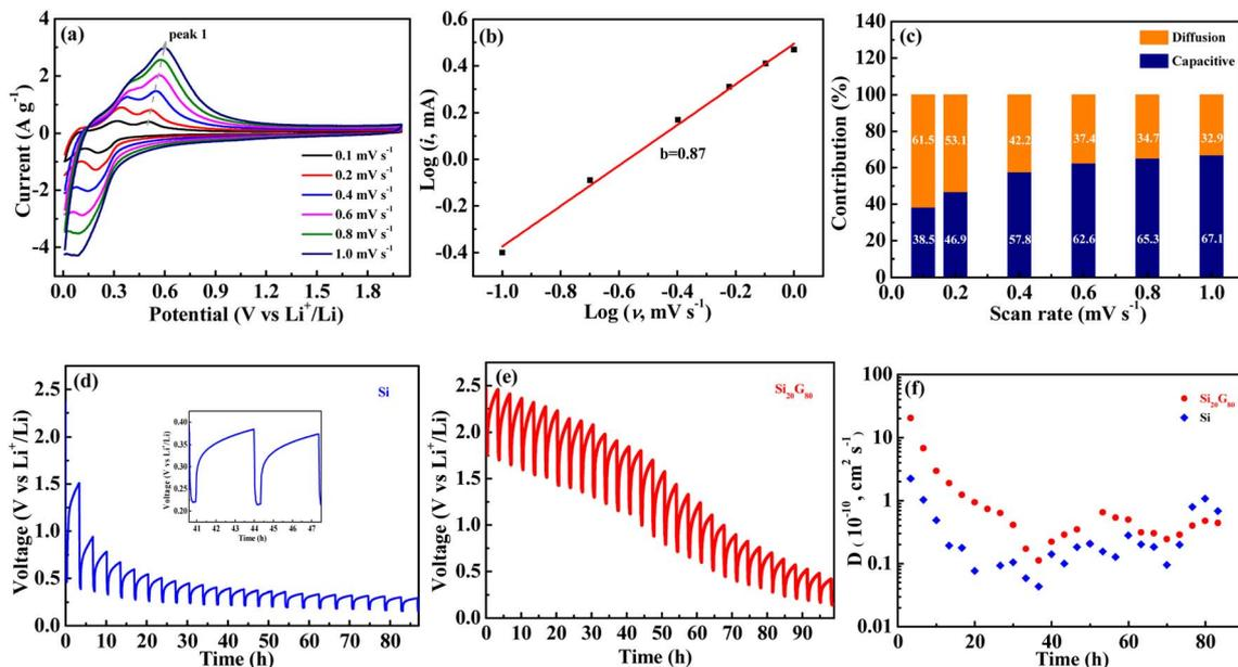
Fig. 5 (a) Cyclic voltammograms (CV), (b)  $\log(i)/\log(v)$  plots, and (c) capacitance and diffusion-controlled contributions at different scan rates of  $\text{Si}_{20}\text{G}_{80}$  electrodes. GITT curves of (d) Si and (e)  $\text{Si}_{20}\text{G}_{80}$  at the discharge state and (f) corresponding diffusion coefficients.
