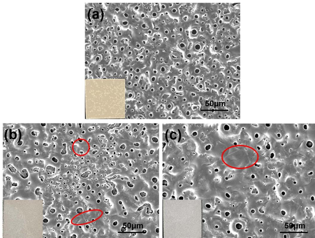
Fig. 3 Surface image of the MAO coating obtained in different electrolytes, (a) base electrolyte, (b) with  $1 \text{ g L}^{-1}$  Cu nanoparticles, (c) with  $2 \text{ g L}^{-1}$  Cu nanoparticles.
