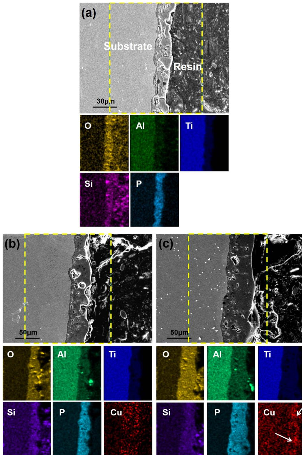
Fig. 4 Cross-section and EDS morphologies of the MAO coating obtained in electrolytes with different contents of Cu nanoparticles, (a) base electrolyte, (b) with  $1 \text{ g L}^{-1}$  Cu nanoparticles, (c) with  $2 \text{ g L}^{-1}$  Cu nanoparticles.
