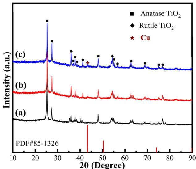
Fig. 6 XRD patterns of the MAO coatings obtained in the electrolytes with different contents of Cu nanoparticles, (a) base electrolyte, (b) with  $1 \text{ g L}^{-1}$  Cu nanoparticles, (c) with  $2 \text{ g L}^{-1}$  Cu nanoparticles.
