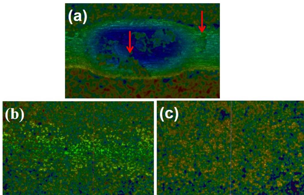
Fig. 9 Friction wear traces of the MAO coatings obtained in electrolytes with different contents of Cu nanoparticles, (a) base electrolyte, (b) with  $1 \text{ g L}^{-1}$  Cu nanoparticles, (c) with  $2 \text{ g L}^{-1}$  Cu nanoparticles.
