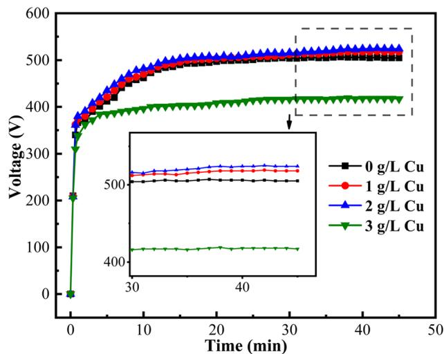
Fig. 1 Voltage variation with time in the electrolyte with different concentrations of Cu nanoparticles.
