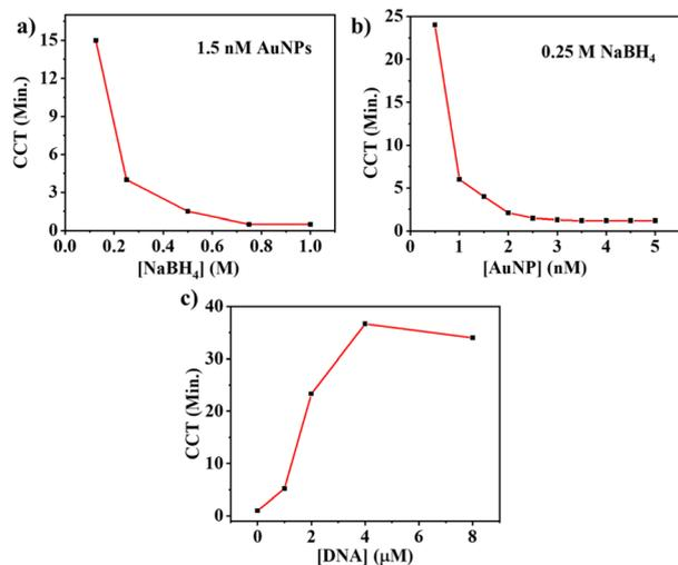
Fig. 3 (a) CCT with varying concentrations of NaBH<sub>4</sub> with 0.01 M 4-NP and 1.5 nM AuNPs. (b) CCT with varying concentrations of AuNPs with 0.01 M 4-NP and 0.25 M NaBH<sub>4</sub>. (c) CCT with varying concentrations of DNA aptamer with 0.25 M NaBH<sub>4</sub>, 1.5 nM AuNPs and 0.01 M 4-NP.
