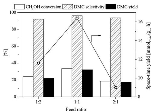
Fig. 10 Effect of feed ratio (CH<sub>3</sub>OH : CO<sub>2</sub>) on CH<sub>3</sub>OH conversion, DMC selectivity, and DMC yield of the flower-like CeO<sub>2</sub> catalyst using 2-CP as dehydrating agent (10 bar, 120 °C).
