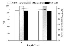
Fig. 13 Recycling of the flower-like CeO<sub>2</sub> catalyst for the DMC synthesis using 2-CP as dehydrating agent (30 bar, 120 °C, CH<sub>3</sub>OH:  $CO_2 = 1:1$ ).
