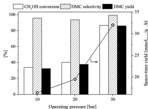
Fig. 12 Effect of operating pressure on CH<sub>3</sub>OH conversion, DMC selectivity, and DMC yield of the flower-like CeO<sub>2</sub> catalyst using 2-CP as dehydrating agent (120 °C, CH<sub>3</sub>OH : CO<sub>2</sub> = 1 : 1).
