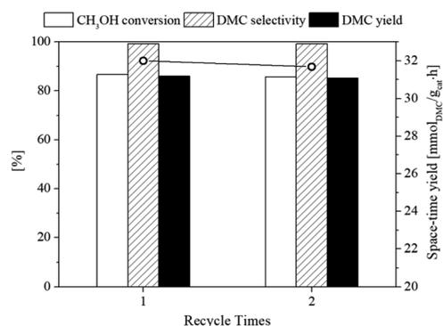
**Fig. 13** Recycling of the flower-like CeO<sub>2</sub> catalyst for the DMC synthesis using 2-CP as dehydrating agent (30 bar, 120 °C, CH<sub>3</sub>OH : CO<sub>2</sub> = 1 : 1).
