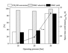
Fig. 12 Effect of operating pressure on CH<sub>3</sub>OH conversion, DMC selectivity, and DMC yield of the flower-like CeO<sub>2</sub> catalyst using 2-CP as dehydrating agent (120 °C, CH<sub>3</sub>OH:  $CO_2 = 1:1$ ).
