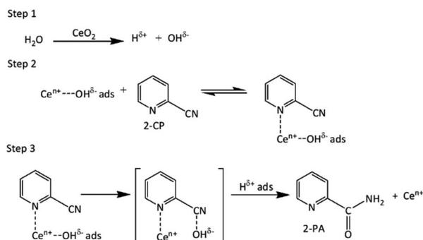
**Scheme 1** Proposed reaction mechanism for the 2-cyanopyridine (2-CP) hydrolysis to form 2-picolinamide (2-PA) over the  $\text{CeO}_2$  catalyst during the DMC synthesis from  $\text{CH}_3\text{OH}$  and  $\text{CO}_2$ .<sup>13</sup>
