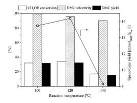
Effect of reaction temperature on CH<sub>3</sub>OH conversion, DMC selectivity, and DMC yield of the flower-like CeO2 catalyst using 2-CP as dehydrating agent (10 bar,  $CH_3OH : CO_2 = 1 : 1$ )
