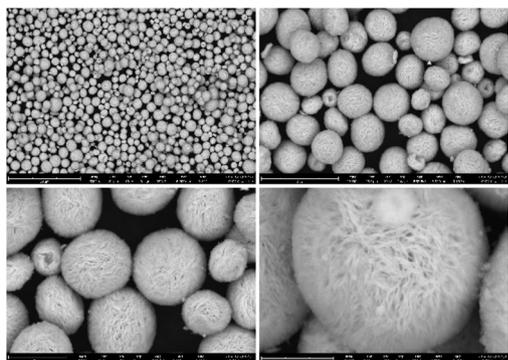
Fig. 3 SEM image of the synthesized flower-like CeO<sub>2</sub> catalyst (before reaction).
