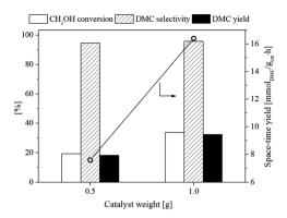
Fig. 11 Effect of catalyst contents on CH<sub>3</sub>OH conversion, DMC selectivity, and DMC yield of the flower-like  $CeO_2$  catalyst using 2-CP as dehydrating agent (10 bar, 120 °C, CH<sub>3</sub>OH:  $CO_2 = 1:1$ ).
