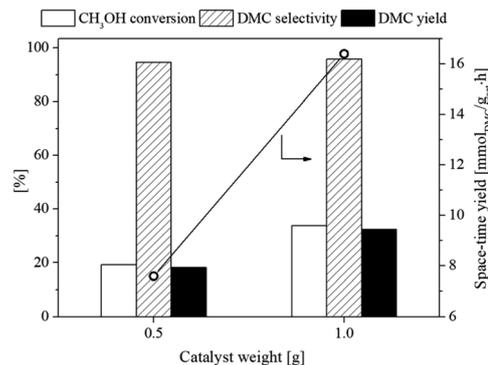
Fig. 11 Effect of catalyst contents on CH<sub>3</sub>OH conversion, DMC selectivity, and DMC yield of the flower-like CeO<sub>2</sub> catalyst using 2-CP as dehydrating agent (10 bar, 120 °C, CH<sub>3</sub>OH : CO<sub>2</sub> = 1 : 1).
