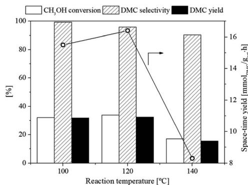
**Fig. 9** Effect of reaction temperature on  $\text{CH}_3\text{OH}$  conversion, DMC selectivity, and DMC yield of the flower-like  $\text{CeO}_2$  catalyst using 2-CP as dehydrating agent (10 bar,  $\text{CH}_3\text{OH}:\text{CO}_2 = 1:1$ ).
