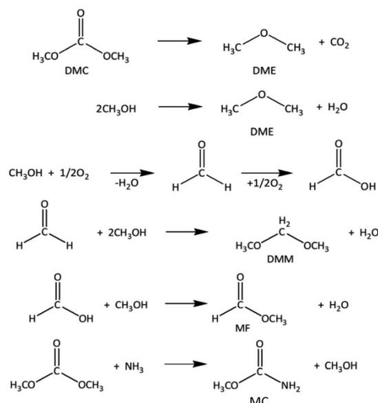
**Scheme 2** Reaction of possible by-products formation during the direct synthesis of DMC from  $\text{CH}_3\text{OH}$  and  $\text{CO}_2$  at high temperatures.<sup>14,53,54</sup>
