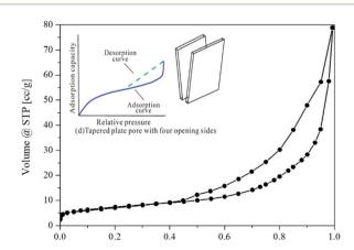
Fig. 5  $N_2$  adsorption-desorption isotherm of the flower-like  $CeO_2$  catalyst and isotherm for tapered plate pore with four opening sides (inset).<sup>49</sup>
