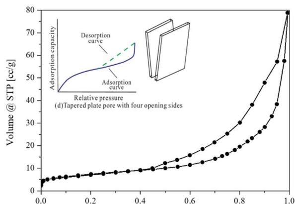
Fig. 5 N<sub>2</sub> adsorption–desorption isotherm of the flower-like CeO<sub>2</sub> catalyst and isotherm for tapered plate pore with four opening sides (inset).<sup>49</sup>
