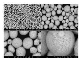
Fig. 3 SEM image of the synthesized flower-like  $CeO_2$  catalyst (before reaction).
