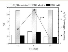
Fig. 10 Effect of feed ratio  $(CH_3OH:CO_2)$  on  $CH_3OH$  conversion, DMC selectivity, and DMC yield of the flower-like  $CeO_2$  catalyst using 2-CP as dehydrating agent (10 bar, 120 °C).
