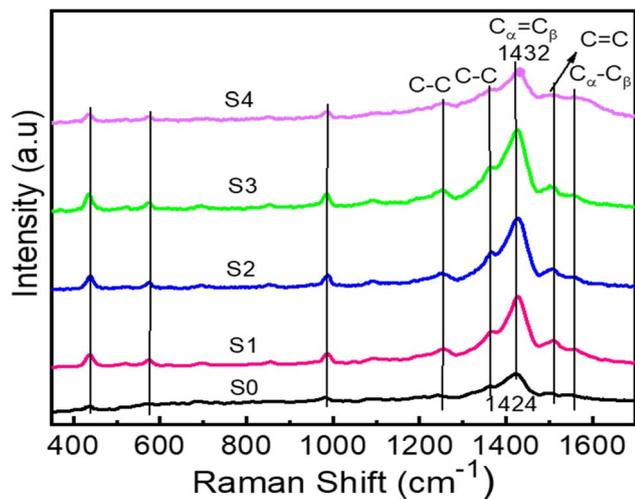
Fig. 4 Raman spectra of S0 (PEDOT:PSS), S1 (PEDOT:PSS/Bi<sub>2</sub>Te<sub>3</sub>), and S2, S3, and S4 (PEDOT:PSS/Bi<sub>2</sub>Te<sub>3</sub>/rGO) composite films. The shifting of the C=C symmetric stretching vibrational mode peak at 1424 cm<sup>-1</sup> to higher wavenumber is attributed to the  $\pi$ - $\pi$  interaction between the electron-rich rGO and the aromatic structures of PEDOT.
