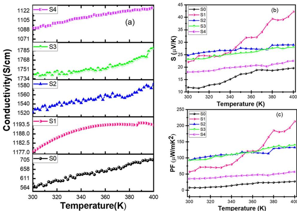
Fig. 6 (a) Measured electrical conductivity, (b) Seebeck coefficient, and (c) power factor of PEDOT:PSS (S0), PEDOT:PSS/0.4%  $\text{Bi}_2\text{Te}_3$  (S1) and PEDOT:PSS/0.4%  $\text{Bi}_2\text{Te}_3$ /0.1% rGO (S2) composite films.
