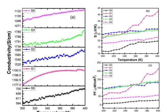
Fig. 6 (a) Measured electrical conductivity, (b) Seebeck coefficient, and (c) power factor of PEDOT:PSS (S0), PEDOT:PSS/0.4% Bi<sub>2</sub>Te<sub>3</sub> (S1) and PEDOT:PSS/0.4% Bi<sub>2</sub>Te<sub>3</sub>/0.1% rGO (S2) composite films.
