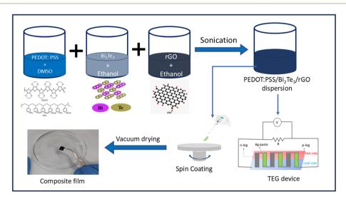
Fig. 1 The schematic illustrates the process flow for preparing the PEDOT:PSS/Bi<sub>2</sub>Te<sub>3</sub>/rGO ternary composite film using the spin coating method.
