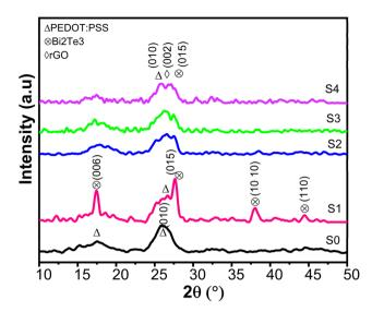
Fig. 2 GIXRD of Raman spectra of S0 (PEDOT:PSS), S1 (PEDOT:PSS/Bi<sub>2</sub>Te<sub>3</sub>), and S2, S3, and S4 (PEDOT:PSS/Bi<sub>2</sub>Te<sub>3</sub>/rGO) composite films.
