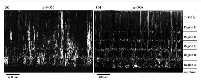
Fig. 9 WB-DF images along  $\langle 2110 \rangle$  zone axis with diffraction vector (a) q = 0-330 and (b) q = 0006.
