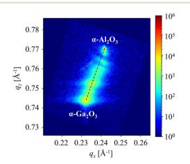
Fig. 5 Reciprocal space mapping around ( $10\bar{1}$ ,10) reflections from compositionally step-graded  $\alpha$ -(Al<sub>x</sub>Ga<sub>1-x</sub>)<sub>2</sub>O<sub>3</sub> layers.
