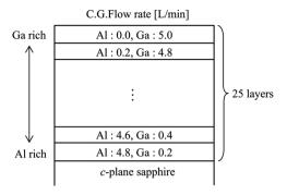
Fig. 4 A schematic diagram of the fabricated compositionally step-graded  $\alpha$ -(Al<sub>x</sub>Ga<sub>1-x</sub>)<sub>2</sub>O<sub>3</sub> layers.
