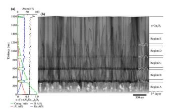
Fig. 8 (a) EDX spectra and (b) cross-sectional BF-STEM image of compositionally step-graded  $\alpha$ -(Al<sub>x</sub>Ga<sub>1-x</sub>)<sub>2</sub>O<sub>3</sub> layers with insertions of  $\alpha$ -Ga<sub>2</sub>O<sub>3</sub> layers.
