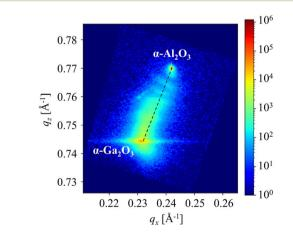
Fig. 7 Reciprocal space mapping around ( $10\overline{1}$ ,10) reflections from compositionally step-graded  $\alpha$ -(Al $_x$ Ga $_{1-x}$ ) $_2$ O $_3$  layers with insertions of  $\alpha$ -Ga $_2$ O $_3$  layers.
