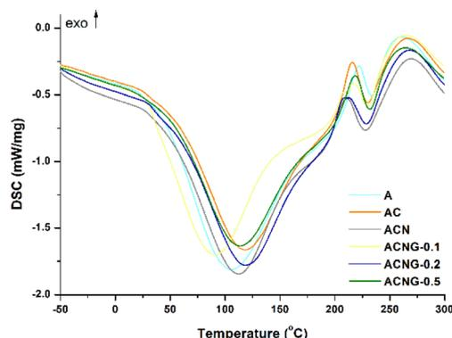
Fig. 7 DSC thermograms of the analyzed materials.
