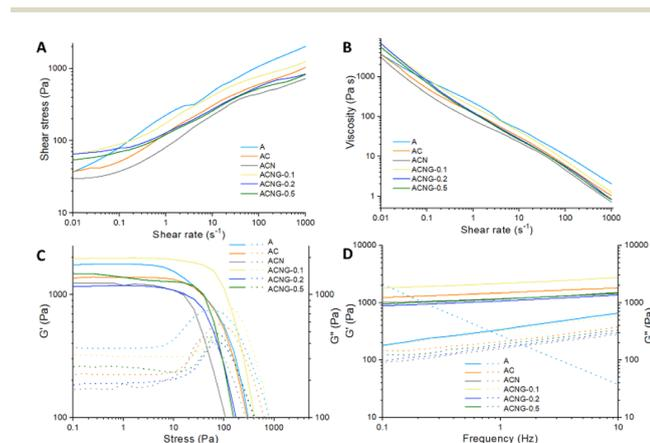
Fig. 1 Rheological results: (A) shear stress and (B) viscosity as a log–log function of shear rates for the formulated inks; elastic and viscous moduli ( $G'$  and  $G''$ ) *versus* (C) stress and (D) frequency for precursor composite inks.
