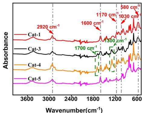
Fig. 1 FTIR spectra of Ti/Mg@s-POP catalysts.
