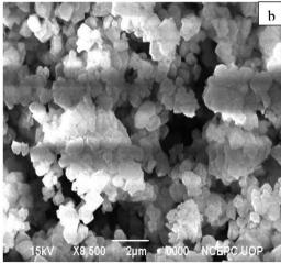
Fig. 2 (a) SEM of zeolite Y, hydrogen (b) SEM of Ni impregnated zeolite Y, hydrogen.
