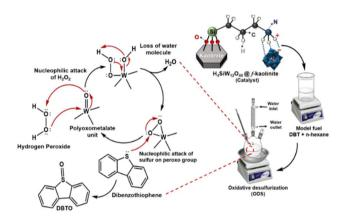
Fig. 9 Proposed mechanism for the conversion of DBT in the oxidative desulfurization process using  $H_aSiW_{12}O_{40}$ @f-kaolinite.
