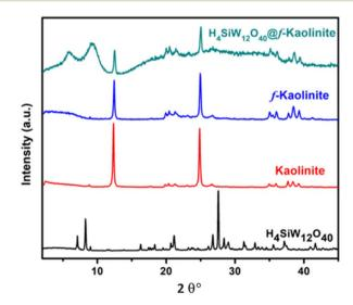
Fig. 4 XRD pattern of  $H_4SiW_{12}O_{40}$ , kaolinite, f-kaolinite, and  $H_4SiW_{12}O_{40}$ @f-kaolinite.
