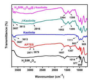
Fig. 1 FTIR spectra of H<sub>4</sub>SiW<sub>12</sub>O<sub>40</sub>, APTES, kaolinite, f-kaolinite, and H<sub>4</sub>SiW<sub>12</sub>O<sub>40</sub>@f-kaolinite.
