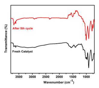
Fig. 11 FT-IR spectra of fresh and recycled catalyst.
