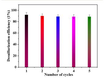
Fig. 10 Recyclability of  $H_4SiW_{12}O_{40}$ @f-kaolinite over five cycles under optimum conditions.
