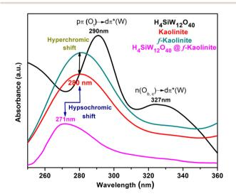
Fig. 3 UV spectra of  $H_4 SiW_{12}O_{40},$  kaolinite, f-kaolinite, and  $H_4 SiW_{12}O_{40}$ @f-kaolinite ( $\approx 3.13\times 10^{-3}$  mM solution).
