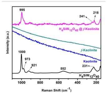
Fig. 2 Raman spectra of H<sub>4</sub>SiW<sub>12</sub>O<sub>40</sub>, kaolinite, f-kaolinite, and H<sub>4</sub>SiW<sub>12</sub>O<sub>40</sub>@f-kaolinite.
