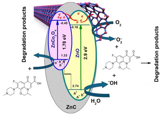
Fig. 8 Proposed photocatalytic mechanism responsible for the degradation of OFL by xCnts@ZnC hydrid.
