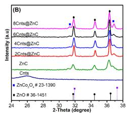
Fig. 1 (A and B) XRD patterns of (a) Cnts, ZnC and xCnt@ZnC (x = 2, 4, 6, 8).
