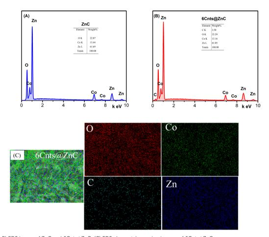
Fig. 5 (A and B) EDS image of ZnC and 6Cnts@ZnC; (C) EDS elemental mapping images of 6Cnts@ZnC
