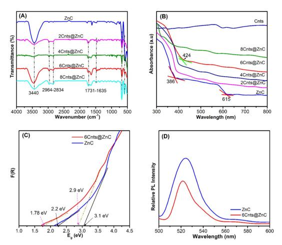
(A) FT-IR and (B) UV-vis DRS patterns of Cnts; ZnC; xCnt@ZnC (x = 2, 4, 6, 8). (C)  $E_a$  of ZnC and 6Cnts@ZnC; (D) PL of ZnC and 6Cnts@ZnC.
