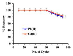
Fig. 8 Reusability of FCM for Pb( $_{\rm II}$ ) and Cd( $_{\rm II}$ ) extraction from aqueous solution (experimental condition: sample volume 100 mL; sample pH 6.0; sorbent amount 500 mg; metal ion concentration 250 ppm; flow rate 8 mL min $^{-1}$ ).
