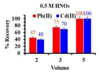
Fig. 7 Effect of different stripping agents (volume and concentration) on the recovery of adsorbed metal ions (experimental condition: sample volume 100 mL; sample pH 6.0; sorbent amount 500 mg; metal ion concentration 250 ppm; sample flow rate 8 mL min<sup>-1</sup>).
