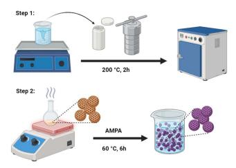
Fig. 1 Schematic illustration of FCM synthesis steps
