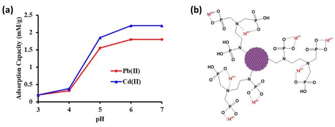
Fig. 5 (a) Effect of solution pH on the adsorption of metal ions (experimental condition: sample volume 100 mL; sorbent amount 500 mg; metal ion concentration 250 ppm; flow rate 8 mL min $^{-1}$ ); (b) possible adsorption mechanism of FCM by metal ion complexation at optimum sample pH.
