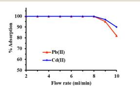
**Fig. 6** Effect of solution flow rate on the adsorption of metal ions (experimental condition: sample volume 100 mL; sample pH 5.0; sorbent amount 500 mg; metal ion concentration 250 ppm).
