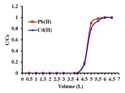
Fig. 9 Breakthrough profile of FCM for Pb(II) and Cd(II) adsorption (experimental condition: sample volume 100 mL; sample pH 6.0; sorbent amount 500 mg; metal ion concentration 250 ppm; flow rate  $8 \text{ mL min}^{-1}$ ).
