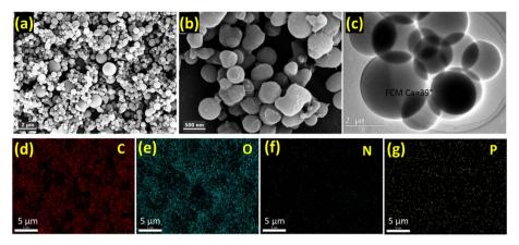
Fig. 3 (a and b) SEM micrographs of FCM at varying magnifications shows physical appearance with smooth surface morphology; (c) TEM micrographs of FCM depicts porous structure of FCM; (d-g) elemental mapping images of FCM depicts uniform distribution of constituent elements.
