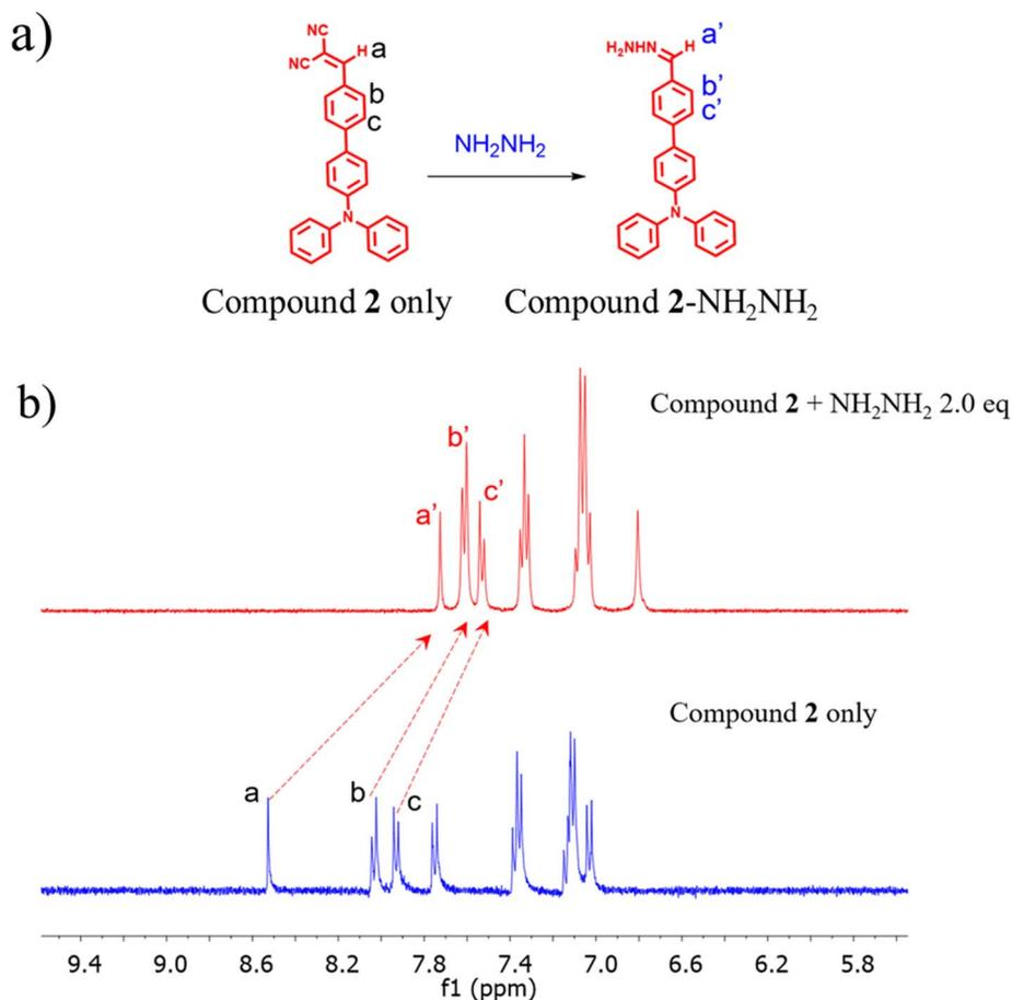
Fig. 7 (a) Chemical structure of the product (compound 2 +  $\text{NH}_2\text{NH}_2$ ) in the presence of hydrazine and (b)  $^1\text{H}$ -NMR titration of compound 2 in the absence and presence of hydrazine in  $\text{DMSO}-d_6$ .
