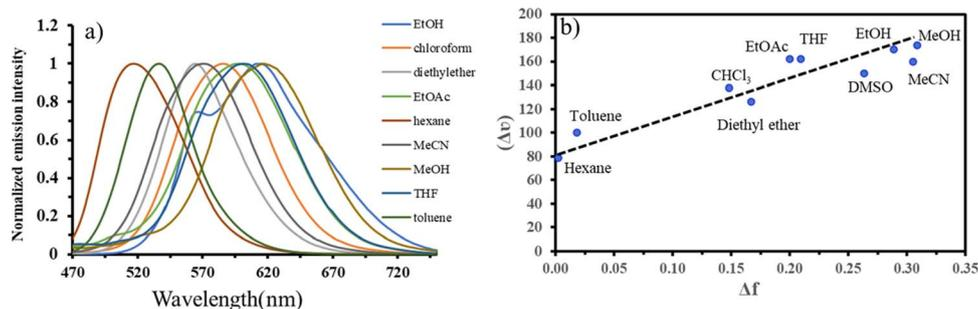
Fig. 1 (a) Normalized fluorescence emission spectra of compound 2 in different solvents at 10  $\mu\text{M}$ , with the excitation wavelength set to the longest absorption wavelength of compound 2. (b) Lippert–Mataga plots illustrating the relationship between the Stokes shift and the orientation polarization of different solvents for compound 2.
