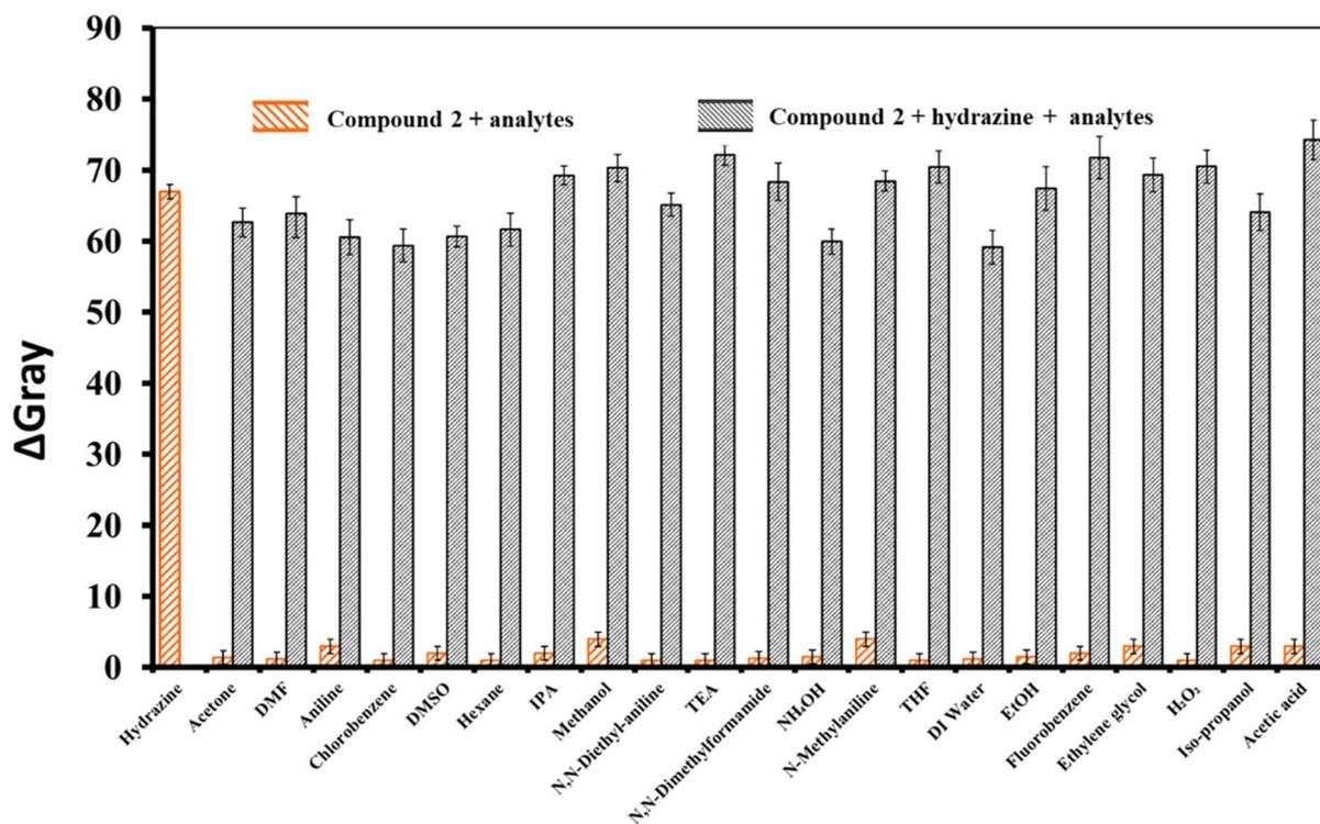
Fig. 5 Differences in the intensities of the fluorescent images ( $\Delta$ Gray) of the nanofibrous sheet of compound 2 exposed for 6 min at r.t. to several analytes (0.08% w/v) (22 compounds) and hydrazine (0.08% w/v).
