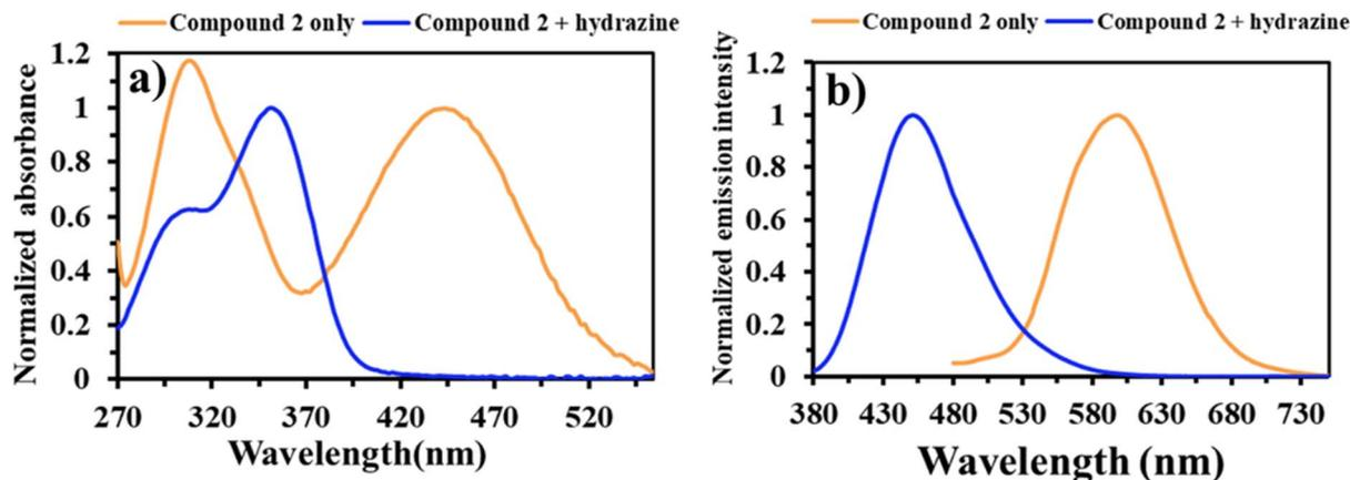
Fig. 2 Changes in the normalized absorption (a) and emission spectra (b) for compound 2 (10  $\mu\text{M}$ ) before (orange line) and after (blue line) the addition of  $\text{N}_2\text{H}_4$  (10  $\mu\text{M}$ ) in DMSO.
