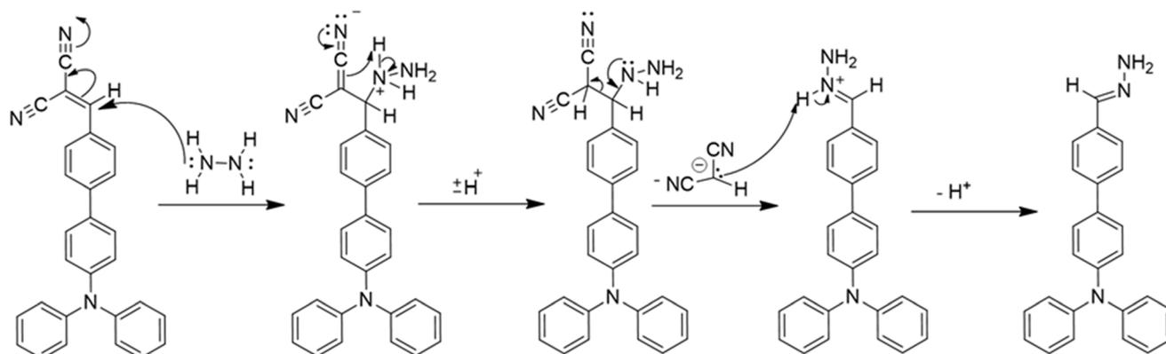
Scheme 2 Detection mechanism of compound 2 for hydrazine.
