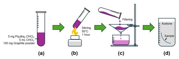
Fig. 2 Illustration of palladium deposition process on carbon surface. (a) A screw cap tube with  $Pd_2dba_3 \cdot CHCl_3$  (5 mg), graphite powder (100 mg), and  $CHCl_3$  (5 mL). (b) Stirring at 50 °C for 1 hour. (c) Filtration to separate the transparent solution from the carbon material. (d) The material is washed with acetone.
