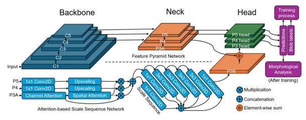
Fig. 1 The structure of employed deep learning-based detector model
