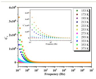
Fig. 16 Frequency-dependent behavior of permittivity in GCO perovskite at various temperatures.
