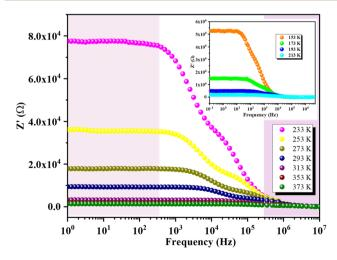
Fig. 10 Frequency-dependent impedance behavior in GCC compound.
