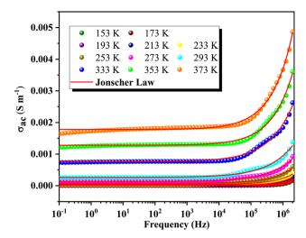
Fig. 6 Temperature-dependent conductivity spectra of GCO chromite.
