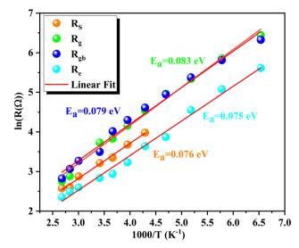
Fig. 13 Logarithmic variation of  $R_{\rm s}$ ,  $R_{\rm g}$ ,  $R_{\rm gb}$  and  $R_{\rm e}$  with inverse temperature.
