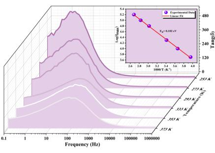
Fig. 19 Dielectric loss characteristics and activation energy analysis of GCO chromite.
