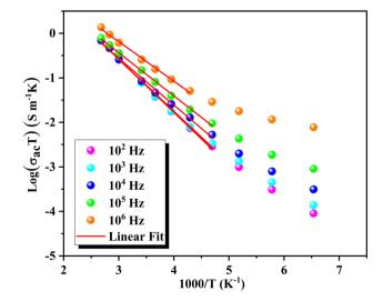
Fig. 9 Temperature dependence of  $\log(\sigma_{ac}T)$  and Arrhenius activation energy for GCO compound across frequencies.
