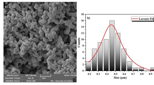
Fig. 3 (a) SEM image and (b) the average grains size histograms of GdCrO<sub>3</sub>.
