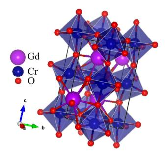
Fig. 2 Orthorhombic unit cell of GCO perovskite material modeled with Vesta Software.
