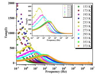
Fig. 18 Frequency-dependent dielectric loss ( $\tan g(\delta)$ ) of GCO chromite across different temperatures.
