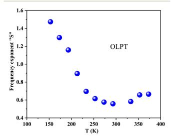
Fig. 7 Thermal variation of  ${\bf s}$  indicating polaronic conduction  ${\it via}$  the OLPT model.
