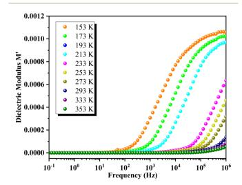
Fig. 14 Frequency dependence of the real part of modulus  $M^\prime$  at different temperatures.
