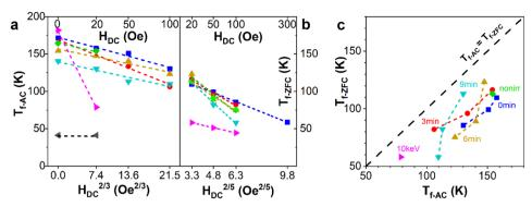
Fig. 5 (a)  $T_f$  vs.  $H_{DC}^{2/3}$  derived from AC magnetometry and (b)  $T_f$  vs.  $H_{DC}^{2/5}$  of the ZFC/FC protocol. The development of  $T_{f-ZFC}$  is shown except for FeAl\_25 keV, where the spin glass transition of the IFM phase is not observed. (c) Correlation of  $T_f$ 's obtained from AC and ZFC curves.
