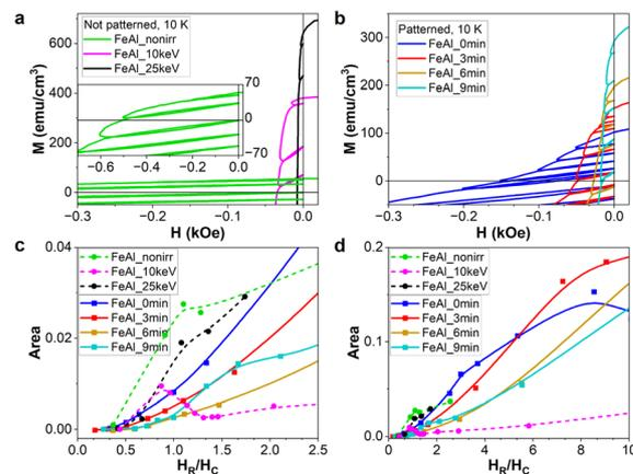
Fig. 3 (a and b) Recoil loops for the non-patterned and patterned samples, respectively. The dependence of the hysteretic area within the recoil loops on the reverse field  $H_R$  relative to  $H_C$  and the preparation conditions are shown in (c and d). The inset in (a) shows the recoil loops for FeAl\_nonirr samples in a larger range of magnetic fields.
