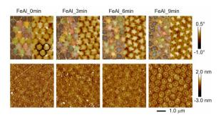
Fig. 1 MFM (top row) and corresponding AFM images of the  $Fe_{60}Al_{40}$  films irradiated through PS nanospheres. The original size of the spheres is indicated by black circles in the upper left figure. The identifiers of the samples indicate the etching time. Color scales for the phase (MFM) and height (AFM) are shown on the right. The MFM images (upper row) are overlaid with the shape/size of the non-irradiated areas (left half of each figure), estimated using.<sup>32</sup>
