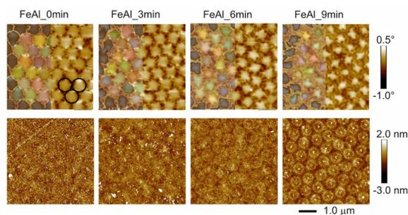
Fig. 1 MFM (top row) and corresponding AFM images of the  $\text{Fe}_{60}\text{Al}_{40}$  films irradiated through PS nanospheres. The original size of the spheres is indicated by black circles in the upper left figure. The identifiers of the samples indicate the etching time. Color scales for the phase (MFM) and height (AFM) are shown on the right. The MFM images (upper row) are overlaid with the shape/size of the non-irradiated areas (left half of each figure), estimated using.<sup>32</sup>
