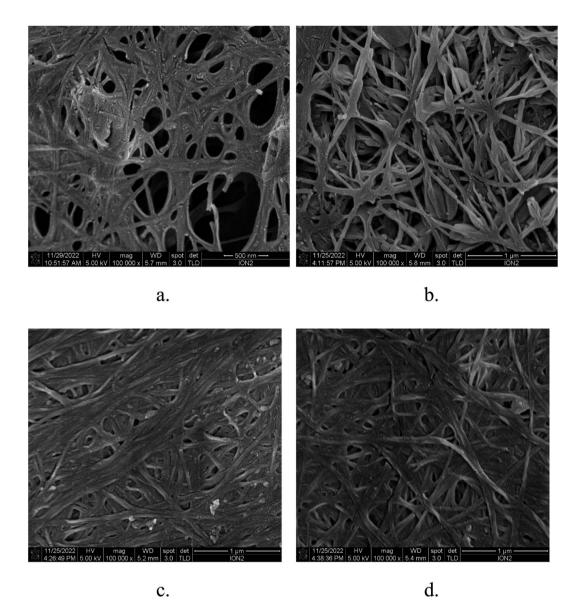
Fig. 1 FESEM morphology of the film surfaces of TNS (a), TS1 (b), TS2 (c), and TS4 (d).
