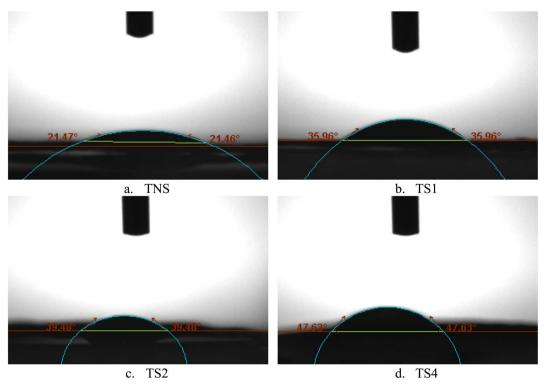
Images of contact angles (θ) of water on different film surfaces of TNS (a), TS1 (b), TS2 (c), TS4 (d) analysed using image software.
