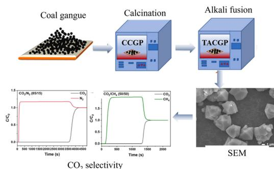
Fig. 7 The process of synthesizing CO<sub>2</sub> adsorbents from coal gangue and their CO<sub>2</sub> adsorption performance.
