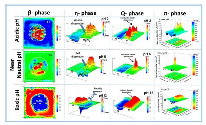
Fig. 17 SVET current density map on typical  $\eta$ -phase (MgZn<sub>2</sub>),  $\beta$ -phase (Al<sub>3</sub>Mg<sub>2</sub>), Q-phase (Al<sub>4</sub>Cu<sub>2</sub>Mg<sub>8</sub>Si<sub>7</sub>), and  $\pi$ -phase (Al<sub>8</sub>Mg<sub>3</sub>FeSi<sub>6</sub>) coupled to aluminum in different pH environments. This figure has been adapted/reproduced from (ref. 8, 73, 103, 131 and 142) with permission from Elsevier, copyright 2024.
