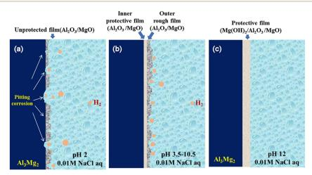
Fig. 14 The schematic of the surface physical models of  $Al_3Mg_2$  after immersion in 0.01 M NaCl solution of (a) pH 2; (b) pH 3.5–10.5 and (c) pH 12.139
