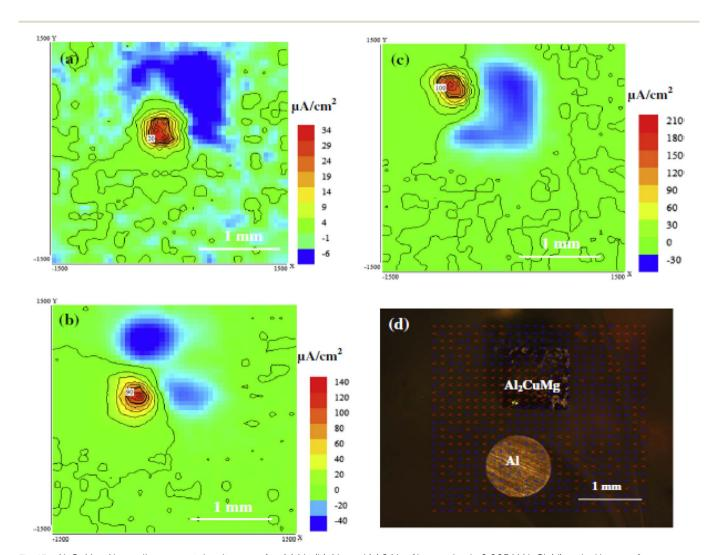
Fig. 13 Al<sub>2</sub>CuMg-Al coupling current density map after (a) 1 h, (b) 4 h, and (c) 24 h of immersion in 0.005 M NaCl, (d) optical image after exposure for 24 h.113 This figure has been adapted/reproduced from (ref. 113) with permission from Elsevier, copyright 2024.
