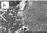
Fig. 12 Surface morphology of Al<sub>2</sub>Cu/Al surface picture without and after immersion (a) 0 h; (b) 96 h of 0.1 M Na<sub>2</sub>SO<sub>4</sub>. This figure has been adapted/reproduced from (ref. 108) with permission from Elsevier, copyright 2024.
