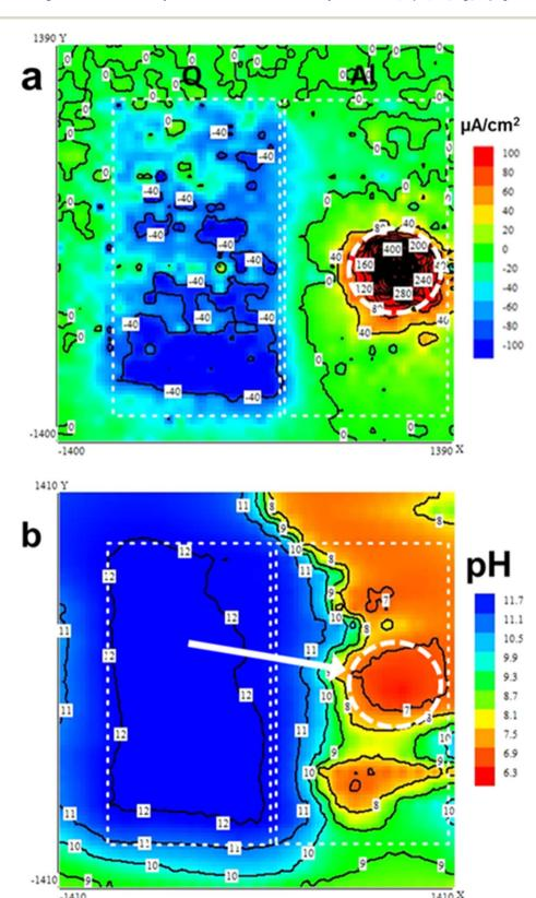
Fig. 9 Successive SIET-SVET scan of the Q-phase/Al couple after an hour in NaCl containing solution at 6 pH value: (a) SVET current density map, and (b) SIET pH map. This figure has been adapted/reproduced from (ref. 8) with permission from ELSEVIER, copyright 2024.
