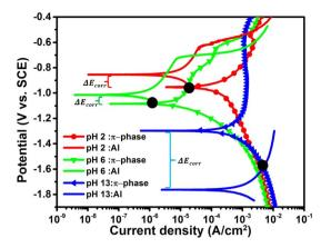
Fig. 10 The  $\pi$ -phase and pure Al potentiodynamic polarization plots in sodium chloride solutions at different pH values. This figure has been adapted/reproduced from (ref. 103) with permission from Elsevier, copyright 2024.
