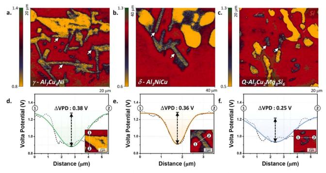
Fig. 5 Volta potential maps (insets) and line profiles of (a, d)  $\gamma$ -Al<sub>7</sub>Cu<sub>4</sub>Ni, (b, e)  $\delta$ -Al<sub>3</sub>NiCu, and (c, f) Q-Al<sub>5</sub>Cu<sub>2</sub>Mg<sub>8</sub>Si<sub>6</sub> phases in T6-treated aluminum alloy. This figure has been adapted/reproduced from (ref. 36) with permission from Elsevier, copyright 2024.
