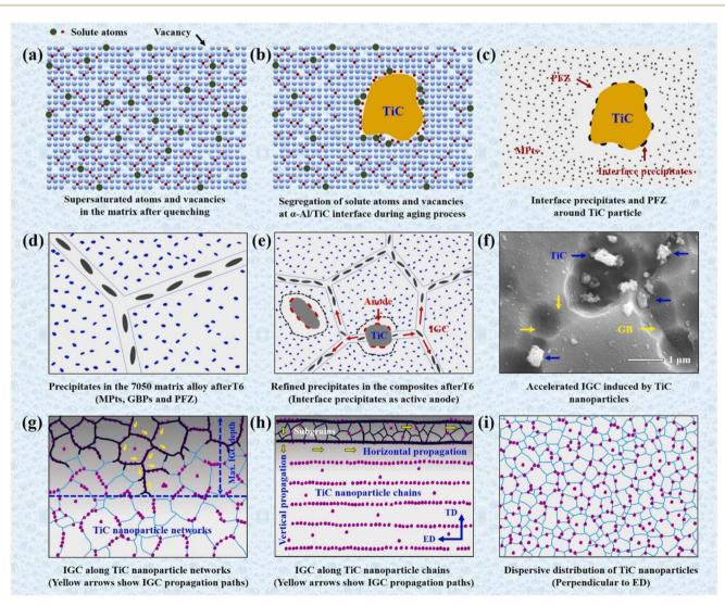
Fig. 4 Schematic of interface precipitation and corrosion mechanisms in Al–Zn–Mg–Cu aluminum alloy composite: (a–c) preferential segregation of precipitates at the  $\alpha$ -Al/TiC interface; (d and e) difference in aging kinetics between alloy and composites; (f) initiation and propagation of IGC in composites (g–i) IGC susceptibility to TiC particles distribution configurations. This figure has been adapted/reproduced from (ref. 34) with permission from Elsevier, copyright 2024.
