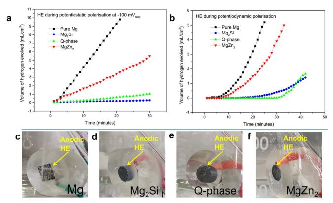
Fig. 18 Hydrogen evolution per surface area on pure Mg, Mg<sub>2</sub>Si, Q-phase, and MgZn<sub>2</sub> electrodes during (a) potentiodynamic polarization, (b) potentiostatic polarization at  $-100 \text{ mV}_{SCE}$  (c), (d), (e), and (f) are photographs showing the evolution of hydrogen on the electrodes at  $-100 \text{ mV}_{SCE}$ . This figure has been adapted/reproduced from (ref. 183) with permission from Springer Nature, copyright 2024.
