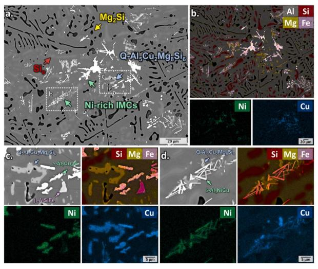
Fig. 6 (a) BSE images and (b) EDS elemental maps of Al single bond Si single bond Mg single bond Cu single bond Ni alloys after T6 treatment. High-magnification BSE images and corresponding EDS elemental maps of (c)  $\gamma$ -Al<sub>7</sub>Cu<sub>4</sub>Ni and (d)  $\delta$ -Al<sub>3</sub>NiCu phases.<sup>36</sup> This figure has been adapted/reproduced from (ref. 36) with permission from Elsevier, copyright 2024.
