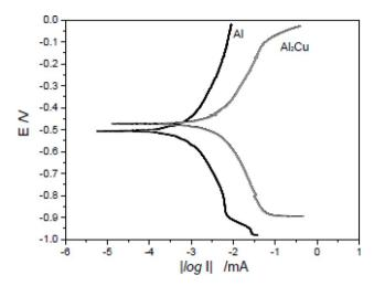
Fig. 11 Potentiodynamic polarization plots for  $Al_2Cu$  and pure Al in  $0.1 \, M \, Na_2SO_4$  solution. This figure has been adapted/reproduced from (ref. 108) with permission from Elsevier, copyright 2024.
