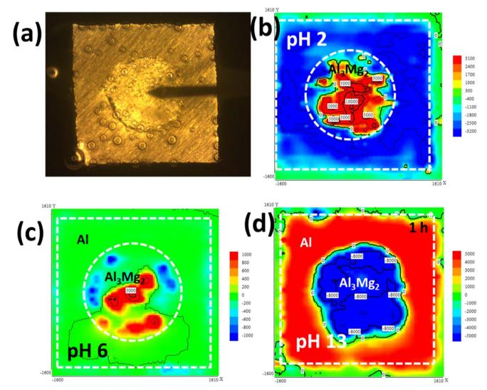
Fig. 15 SVET current density distribution on  $Al_3Mg_2$  embedded in pure Al matrix in 0.1 M NaCl solutions at different pH values (a) microscopic image of sample-probe arrangement (b) pH 2, (c) pH 6 (d) pH 13. This figure has been adapted/reproduced from (ref. 142) with permission from IOP SCIENCE, copyright 2024.
