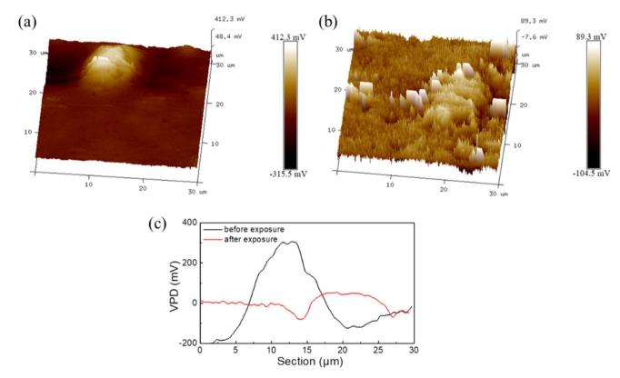
Fig. 3 The VPD of Al-Mn and α-Mg in AM50 (a) before corrosion, (b) after corrosion and (c) corresponding line-profile analysis of relative potential through the secondary phases. This figure has been adapted/reproduced from (ref. 32) with permission from Elsevier, copyright 2024.
