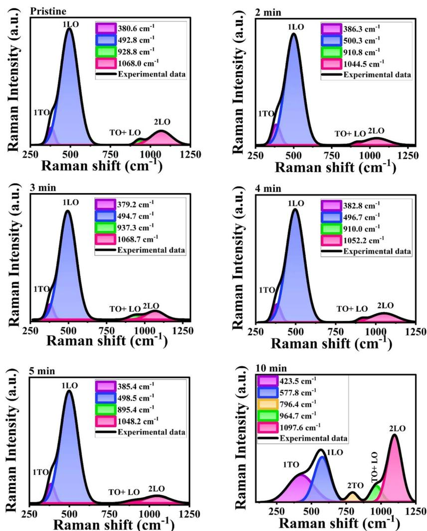
Fig. 7 Deconvoluted Raman spectra of MW irradiated NiO nanostructures films.
