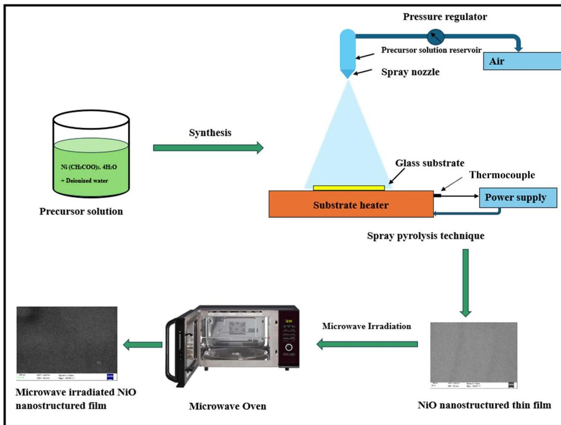
Fig. 2 Schematic representation of process flow for preparation of microwave irradiated NiO nanostructure films.
