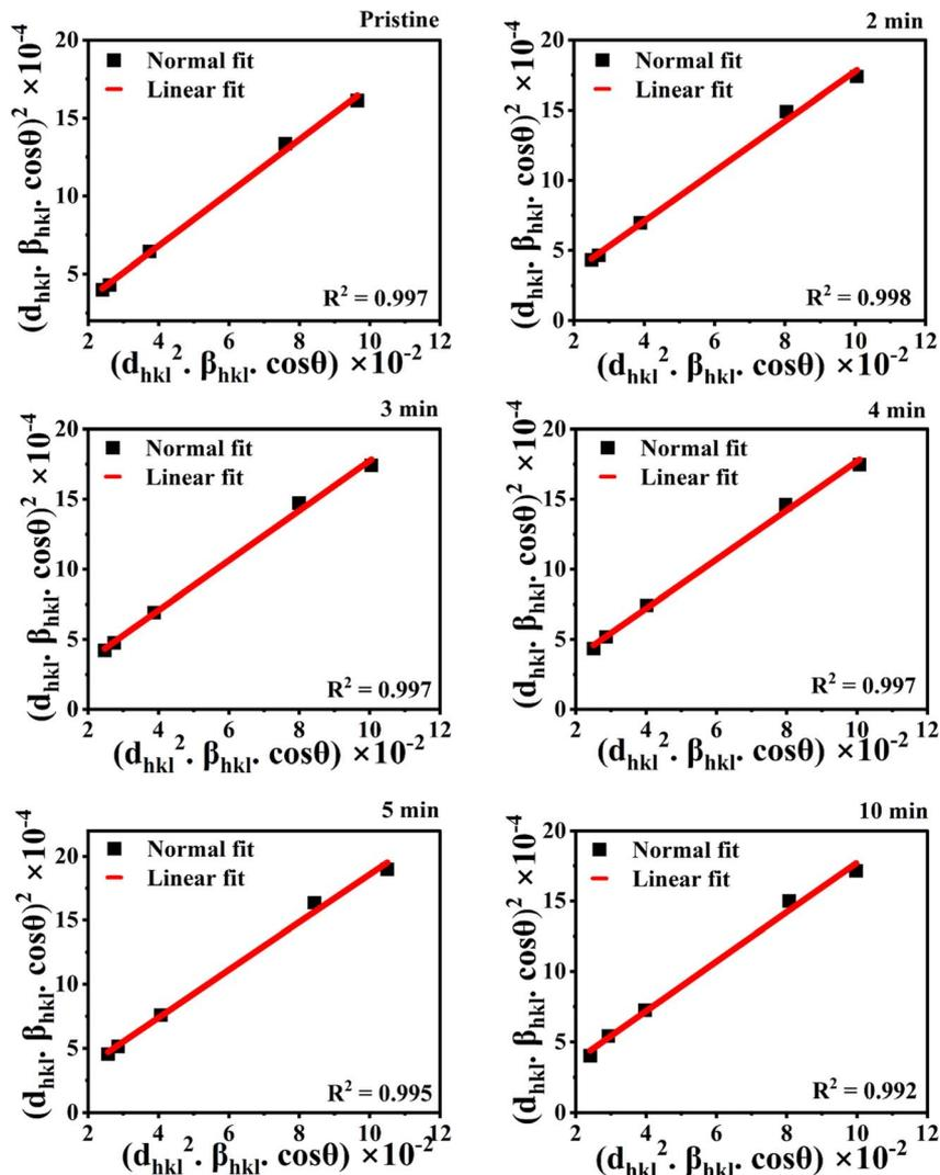
Fig. 6 SSP plot of pristine and MW irradiated NiO nanostructure films.
