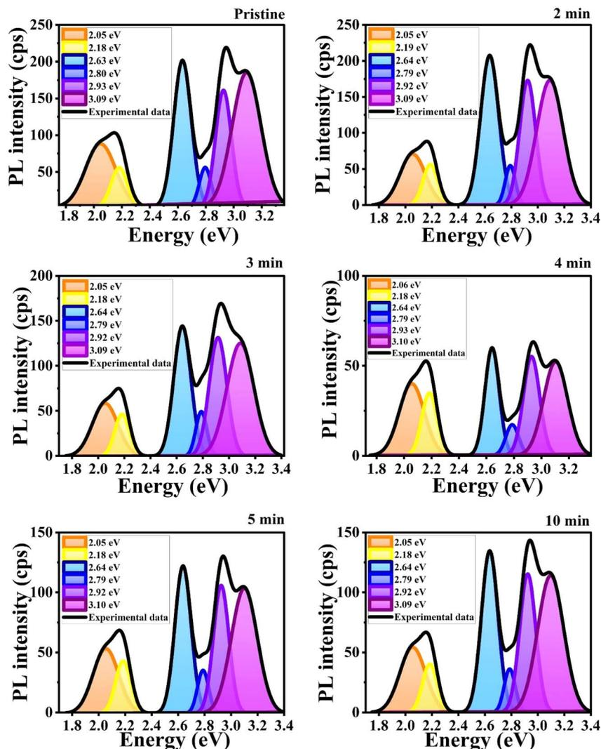
Fig. 15 Gaussian deconvoluted PL emission spectra of MW irradiated NiO nanostructure films.
