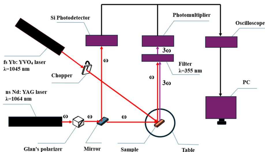
Fig. 4 Experimental setup for laser-induced THG measurement.
