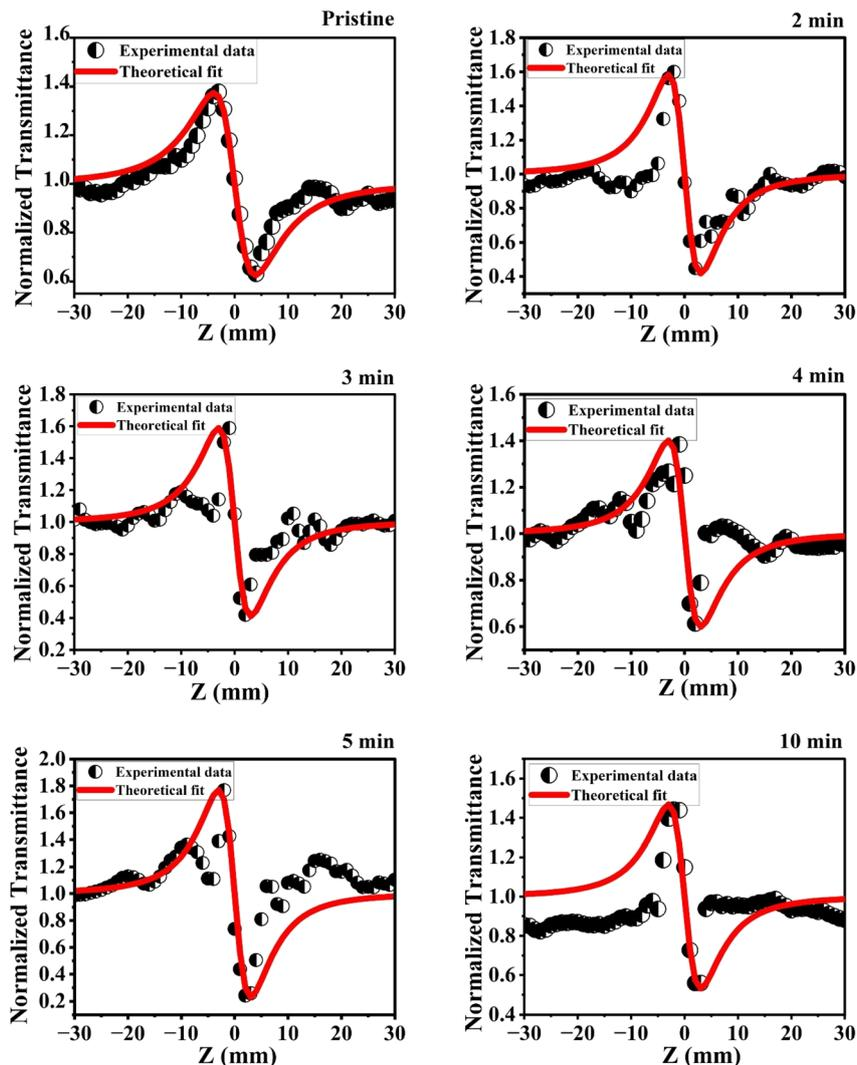
Fig. 18 CA traces of the pristine and MW irradiated NiO nanostructure film.
