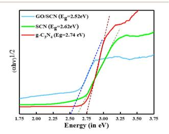
**Fig. 9** Tauc plot representing the bandgap energies of SCN and GO/SCN.
