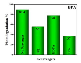
Fig. 18 Influence of radical scavengers for photodegradation of BPA on GO/SCN under visible light irradiation.
