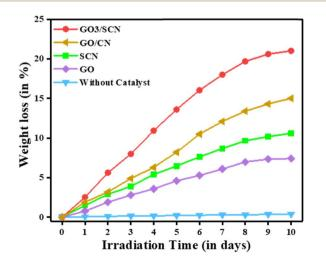
Fig. 12 Weight loss (%) of LDPE films without catalyst, with GO3/SCN, GO/CN, SCN, and GO under visible light irradiation.
