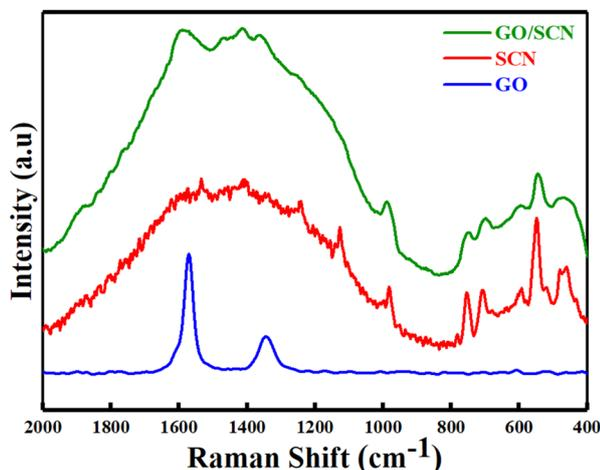
Fig. 4 Raman spectrums of GO, SCN and GO/SCN.
