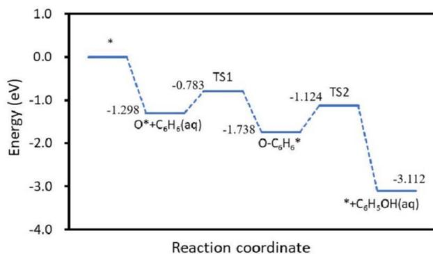
Fig. 15 Benzene catalyzed oxidation reaction path by  $\gamma$ -Al<sub>2</sub>O<sub>3</sub> modified by Cu/Mn/Ce doping.
