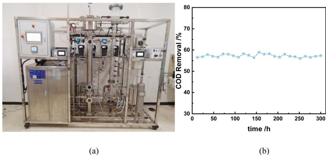
Fig. 17 (a) Catalyst and 20 L h<sup>-1</sup> ozone catalytic oxidation continuous unit; (b) continuous test COD monitoring. (Condition: inlet water flow 10 L h<sup>-1</sup>, O<sub>3</sub> flow 0.4 L min<sup>-1</sup>, O<sub>3</sub> concentration 40 mg L<sup>-1</sup>, retention time 30 min, sampling every 12 h to measure COD.)
