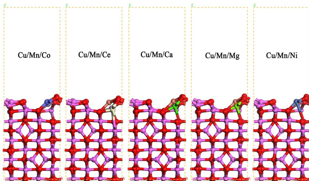
Fig. 1 Surface model of  $\gamma$ -Al<sub>2</sub>O<sub>3</sub> modified by Cu/Mn/Co, Cu/Mn/Ce, Cu/Mn/Ca, Cu/Mn/Mg and Cu/Mn/Ni doping.
