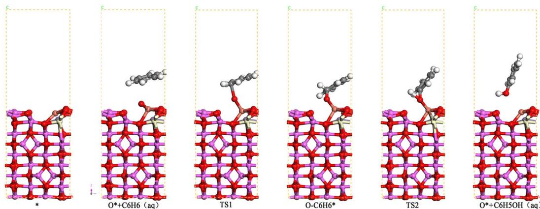
Fig. 14 Reaction configuration of benzene catalyzed oxidation by  $\gamma$ -Al<sub>2</sub>O<sub>3</sub> modified by Cu/Mn/Ce doping.
