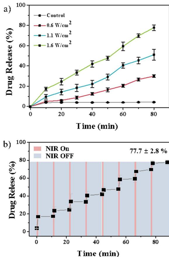
Fig. 3 Drug release profile of PPFA-Nr-GNR with (a) different light power (0.6, 1.1, 1.6 W cm<sup>-2</sup>) and (b) the on-off of the NIR light irradiation.
