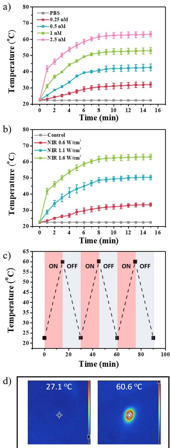
Fig. 2 Temperature change graph of PPFA-GNR with different (a) concentration (0.25, 0.5, 1, 2.5 nM) under the light irradiation (1.6 W cm<sup>-2</sup>) and (b) light power (0.6, 1.1, 1.6 W cm<sup>-2</sup>) with predetermined concentration 2.5 nM. (c) Temperature change graph and (d) infrared camera image of the PPFA-GNR solution by the on-off of the NIR light irradiation.
