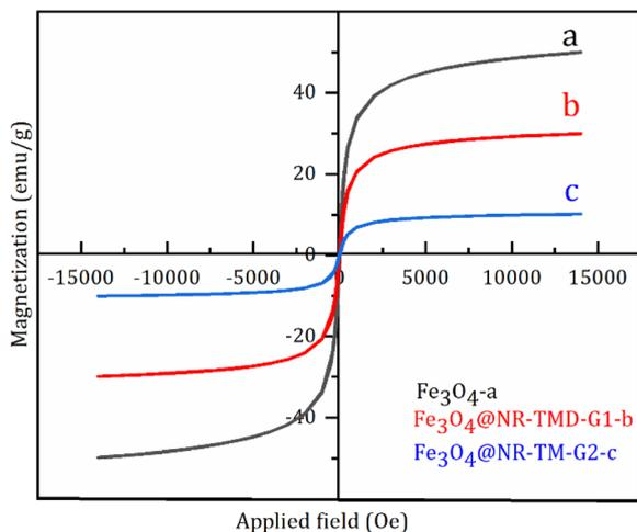
Fig. 4 VSM analyses of  $\text{Fe}_3\text{O}_4$  (a),  $\text{Fe}_3\text{O}_4@NR-TMD-G1$  (b), and  $\text{Fe}_3\text{O}_4@NR-TMD-G2$  (c).
