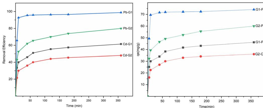
Fig. 8 Effect of contact time on the adsorption of  $\text{Pb(II)}$  and  $\text{Cd(II)}$  by  $\text{Fe}_3\text{O}_4@NR\text{-TMD-G1}$ , and  $\text{Fe}_3\text{O}_4@NR\text{-TMD-G2}$  adsorbents. ( $T = 298\text{ K}$ ,  $\text{pH} = 4.3$ , initial concentration =  $200\text{ mg L}^{-1}$ , adsorbent =  $0.08\text{ g}$ , contact time =  $360\text{ min}$ ).
