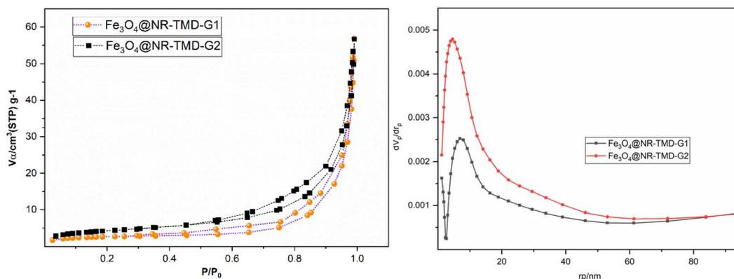
Fig. 5 Adsorption-desorption and pore size distribution plots of  $\text{Fe}_3\text{O}_4@NR-TMD-G1$ , and  $\text{Fe}_3\text{O}_4@NR-TMD-G2$  adsorbents.
