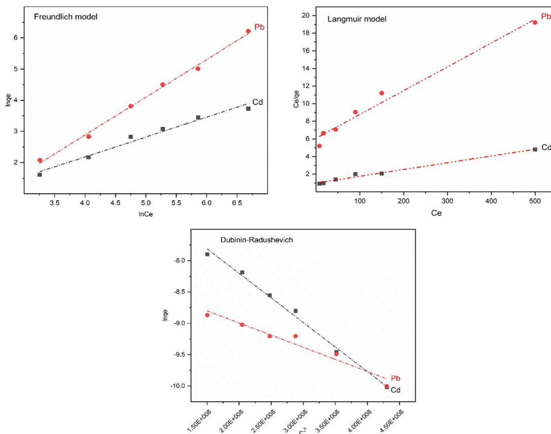
**Fig. 12** Isotherm fitting curves for adsorption of Pb(II) and Cd(II) on Fe<sub>3</sub>O<sub>4</sub>@NR-TMD-G1 nanostructure ( $T = 298$  K).
