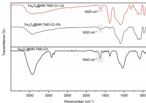
Fig. 17 The FT-IR spectra of Fe<sub>3</sub>O<sub>4</sub>@NR-TMD-G1 nanostructure before and after the adsorption of Pb(II) and Cd(II) ions.
