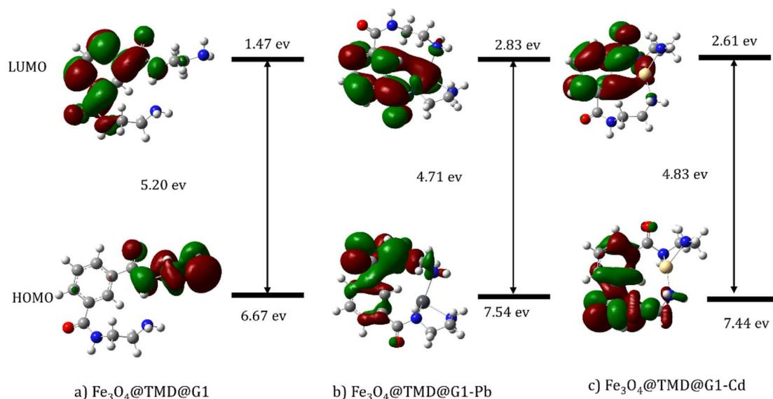
Fig. 14 HOMO and LUMO plots of (a) Fe<sub>3</sub>O<sub>4</sub>@NR-TMD-G1, (b) Fe<sub>3</sub>O<sub>4</sub>@NR-TMD-G1-Pb and (c) Fe<sub>3</sub>O<sub>4</sub>@NR-TMD-G1-Cd structures.
