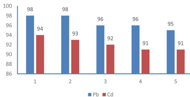
Fig. 15 Reusability of Fe<sub>3</sub>O<sub>4</sub>@NR-TMD-G1 nanostructure for adsorption of Pb(II) and Cd(II) ions from aqueous solutions.
