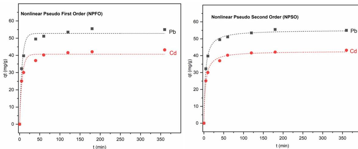
Fig. 11 The fitting curves: non-linear pseudo-first-order and pseudo-second-order models for  $\text{Pb(II)}$  and  $\text{Cd(II)}$  adsorption by  $\text{Fe}_3\text{O}_4\text{@NR-TMD-G1}$ .
