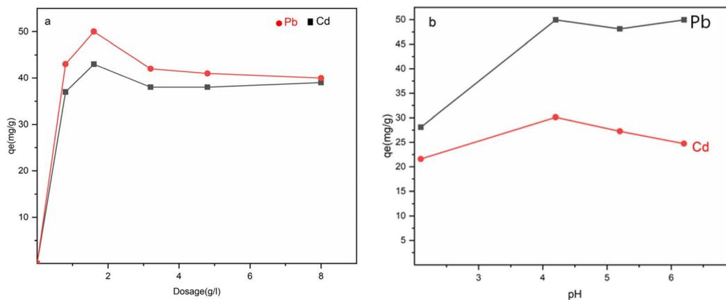
Fig. 9 (a) Effect of adsorbent dosage of  $\text{Fe}_3\text{O}_4\text{@NR-TMD-G1}$  ( $T = 298$  K,  $\text{pH} = 4.3$ , initial concentration =  $200$  mg  $\text{L}^{-1}$ , contact time = 30 min) and (b) effect of pH on the adsorption of  $\text{Pb(II)}$  and  $\text{Cd(II)}$  ions ( $T = 298$  K, initial concentration =  $200$  mg  $\text{L}^{-1}$ , adsorbent =  $0.08$  g, contact time = 30 min).
