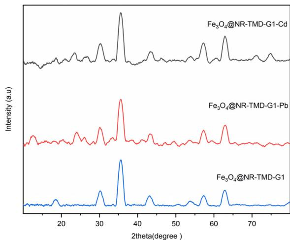
Fig. 16 The XRD patterns of Fe<sub>3</sub>O<sub>4</sub>@NR-TMD-G1 nanostructure before and after the adsorption of Pb(II) and Cd(II) ions.
