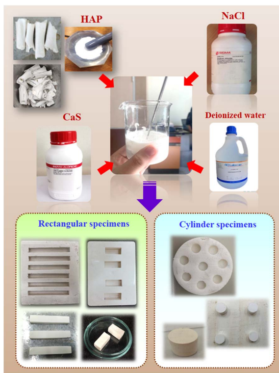
Fig. 1 Schematic of methods to prepare the (0.70CaS–0.30HAP)/xNaCl composite bone cements with different shape.
