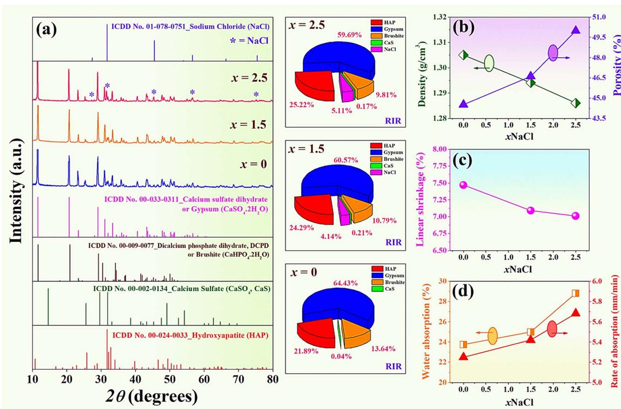
Fig. 3 (a) X-ray diffraction patterns of the (0.70CaS–0.30HAP)/ $x$ NaCl composite bone cements, where  $2\theta = 10\text{--}80^\circ$ , and phase composition (%) analyzed by the Reference Intensity Ratio (RIR) method using SmartLab Studio II program, (b) density and porosity as a function of NaCl content, (c) linear shrinkage as a function of NaCl content, and (d) water absorption and rate of absorption as a function of NaCl content.
