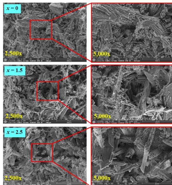
Fig. 6 SEM micrographs with fracture surface mode (2500 $\times$  and 5000 $\times$ ) of the (0.70CaS–0.30HAP)/ $x$ NaCl composite bone cements, where  $x = 0$ –2.5 wt%.
