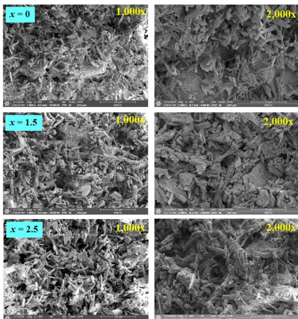
Fig. 5 SEM micrographs with fracture surface mode (1000 $\times$  and 2000 $\times$ ) of the (0.70CaS–0.30HAP)/ $x$ NaCl composite bone cements, where  $x = 0$ –2.5 wt%.
