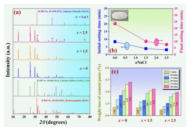
Fig. 2 (a) X-ray diffraction patterns of the (0.70CaS-0.30HAP)/xNaCl mixed powder, where  $2\theta = 10-80^\circ$ , (b) initial setting time and final setting time as a function of NaCl content, and (c) the weight loss of cement paste (%) after immersion in the Ringer's solution as a function of the immersion time.
