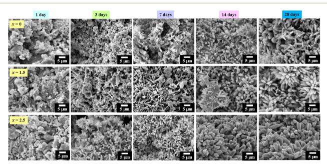
Fig. 8 SEM micrographs of the (0.70CaS-0.30HAP)/xNaCl composite bone cements after being soaked in SBF solution for 1, 3, 7, 14, and 28 days, where x = 0-2.5 wt%.
