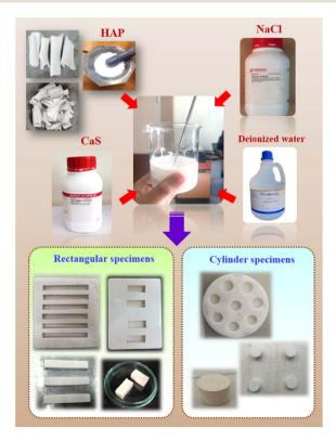
Fig. 1 Schematic of methods to prepare the (0.70CaS-0.30HAP)/xNaCl composite bone cements with different shape.
