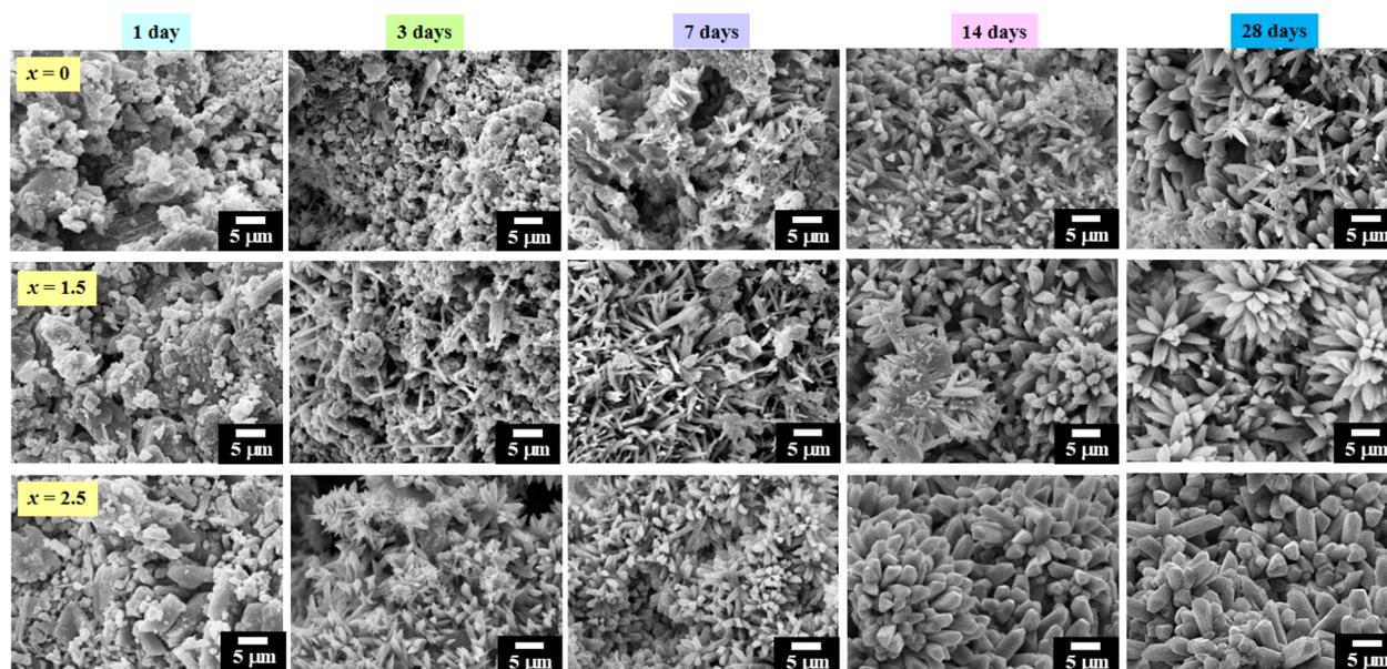
Fig. 8 SEM micrographs of the (0.70CaS–0.30HAP)/*x*NaCl composite bone cements after being soaked in SBF solution for 1, 3, 7, 14, and 28 days, where *x* = 0–2.5 wt%.
