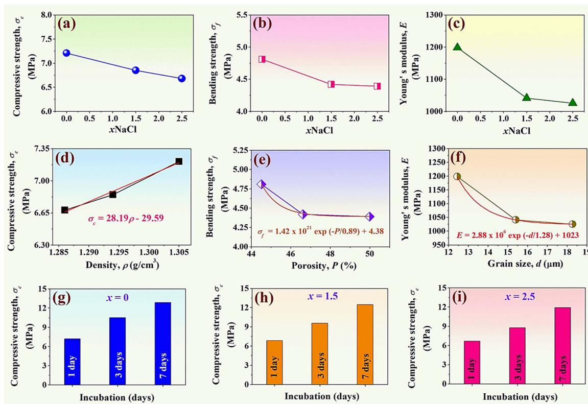
Fig. 7 Plots of (a)  $\sigma_c$  as a function of NaCl content, (b)  $\sigma_f$  as a function of NaCl content, (c)  $E$  as a function of NaCl content, (d)  $\sigma_c$  as a function of  $\rho$ , (e)  $\sigma_f$  as a function of  $P$ , (f)  $E$  as a function of  $d$ , (g)  $\sigma_c$  as a function of incubation of the  $x = 0$  sample, (h)  $\sigma_c$  as a function of incubation of the  $x = 1.5$  sample, and (i)  $\sigma_c$  as a function of incubation of the  $x = 2.5$  sample.
