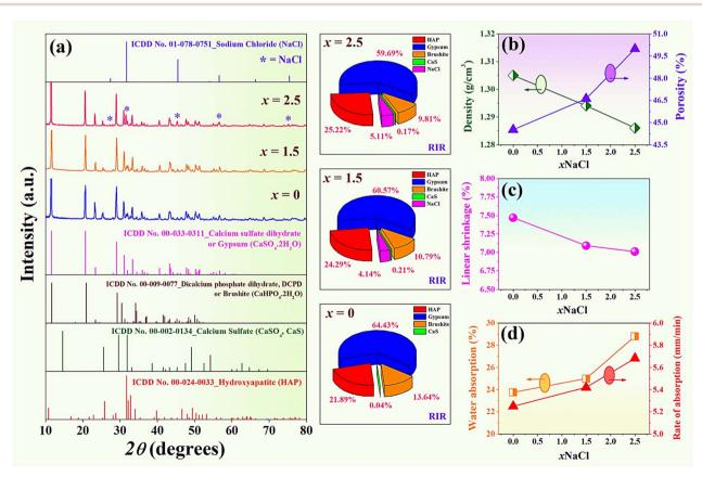
Fig. 3 (a) X-ray diffraction patterns of the (0.70CaS-0.30HAP)/xNaCl composite bone cements, where  $2\theta = 10-80^\circ$ , and phase composition (%) analyzed by the Reference Intensity Ratio (RIR) method using SmartLab Studio II program, (b) density and porosity as a function of NaCl content, (c) linear shrinkage as a function of NaCl content, and (d) water absorption and rate of absorption as a function of NaCl content.
