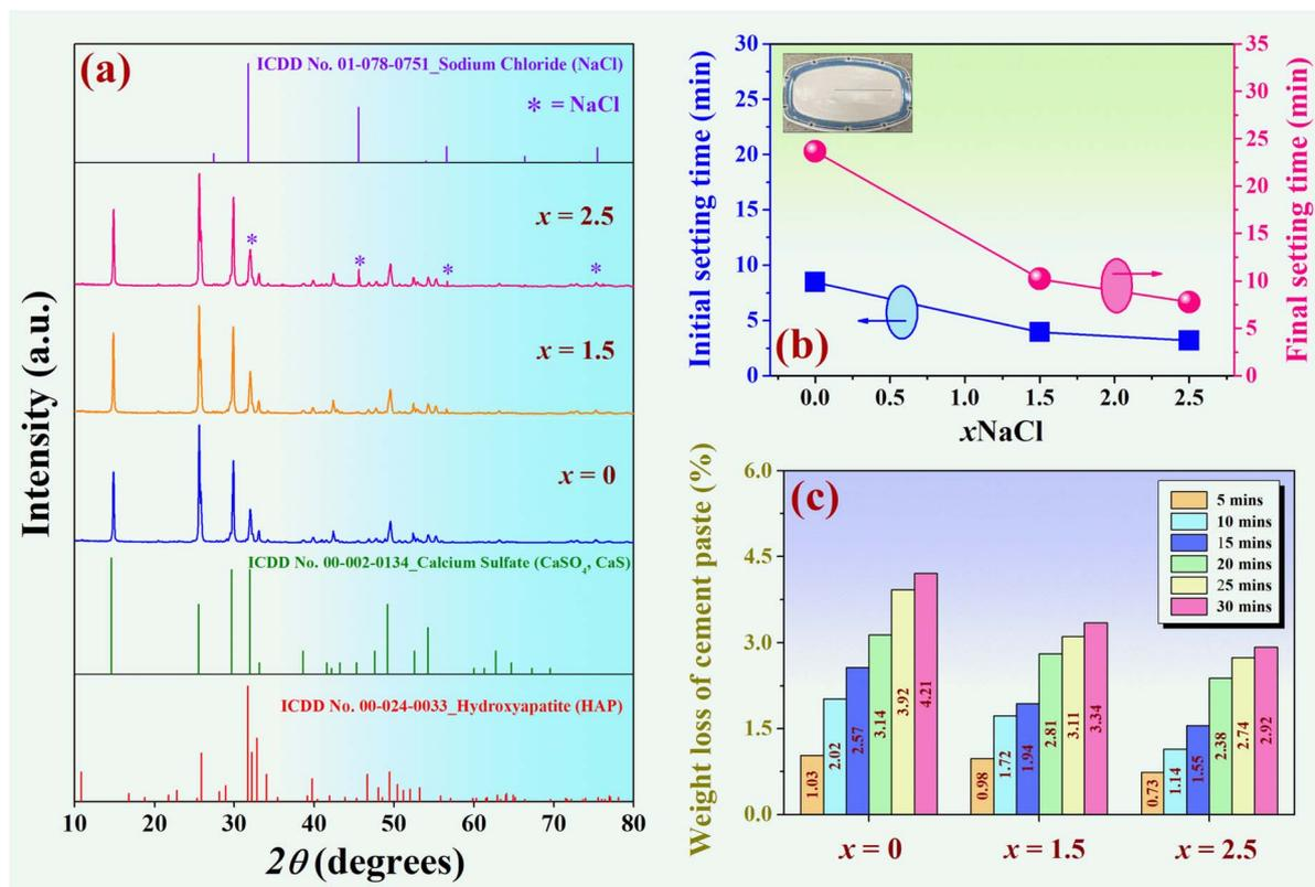
Fig. 2 (a) X-ray diffraction patterns of the (0.70CaS–0.30HAP)/ $x$ NaCl mixed powder, where  $2\theta = 10\text{--}80^\circ$ , (b) initial setting time and final setting time as a function of NaCl content, and (c) the weight loss of cement paste (%) after immersion in the Ringer's solution as a function of the immersion time.
