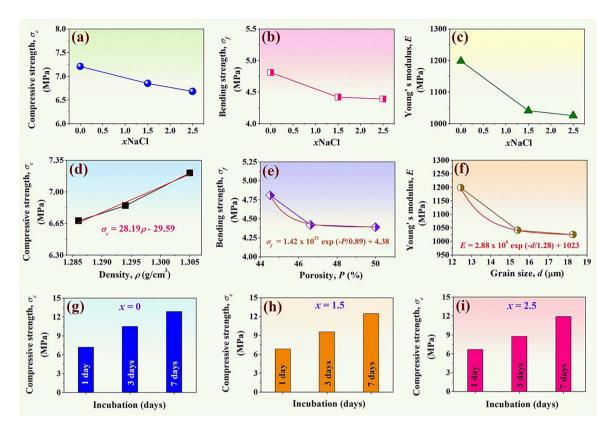
Fig. 7 Plots of (a)  $\sigma_c$  as a function of NaCl content, (b)  $\sigma_f$  as a function of NaCl content, (c) E as a function of NaCl content, (d)  $\sigma_c$  as a function of  $\rho$ , (e)  $\sigma_f$  as a function of P, (f) E as a function of  $\sigma_c$  as a function of incubation of the  $\sigma_c$  and  $\sigma_c$  are  $\sigma_c$  are  $\sigma_c$  and  $\sigma_c$  are  $\sigma_c$  and
