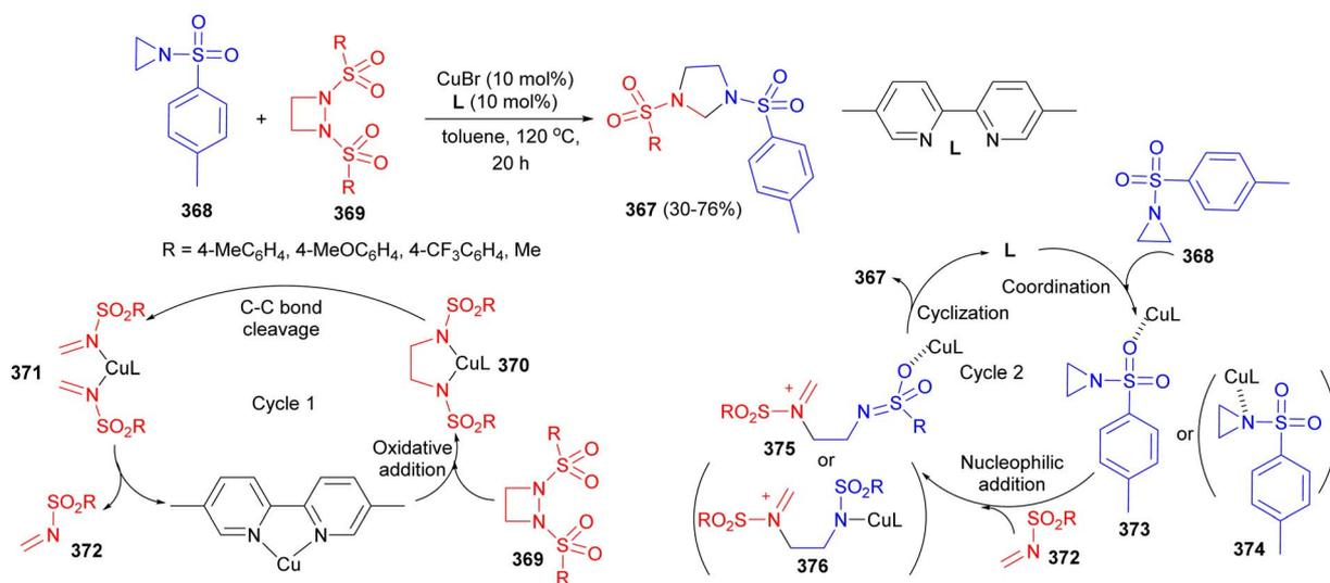
Scheme 102 Cu-catalyzed synthesis of imidazolidines **367**.
