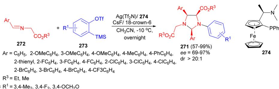
Scheme 80 Synthesis of functionalized imidazolidine derivatives **271** in the presence of Ag(Tf<sub>2</sub>N).
