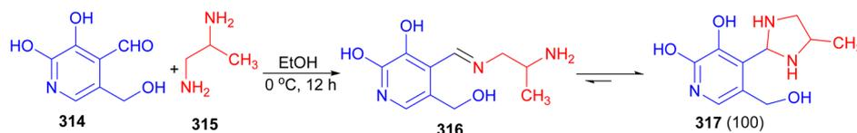
Scheme 89 Synthesis of cyclic 5-(hydroxymethyl)-2-methyl-4-(4-methylimidazolidin-2-yl)pyridin-3-ol tautomer 317.
