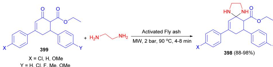
Scheme 108 Synthesis of spiro-imidazolidine derivatives **398** using catalytic amount of fly ash under microwave irradiation.
