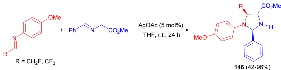
Scheme 49 AgOAc catalyzed synthesis of highly substituted tetrahydroimidazole derivatives 146 .
