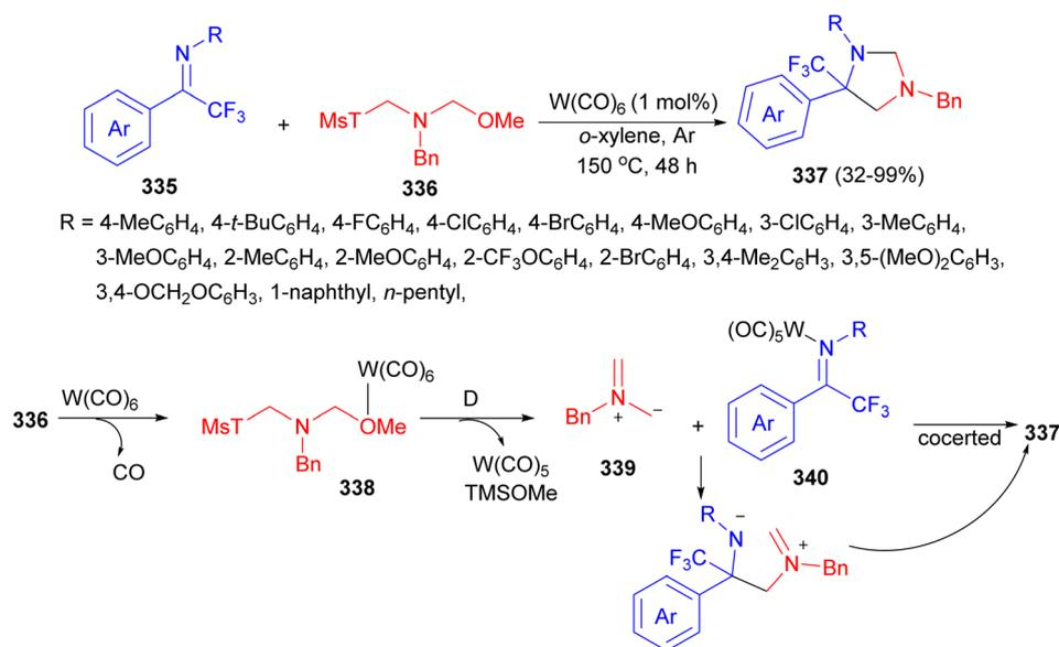
Scheme 94 Tungsten catalyzed synthesis of imidazolidines 337.
