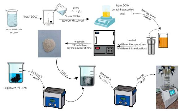
Fig. 1 Schematic preparation scheme of TiO<sub>2-x</sub>/Fe<sub>3</sub>O<sub>4</sub>@g-C
