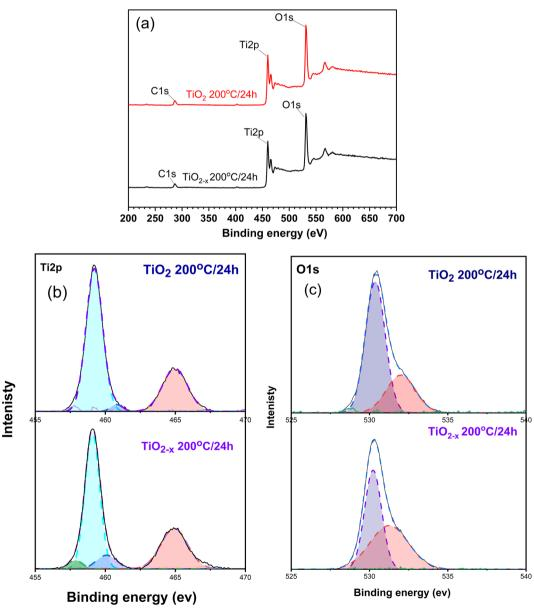
Fig. 7 XPS spectra of the prepared samples; (a) full scan and (b and c) deconvoluted spectra of Ti and O elements.
