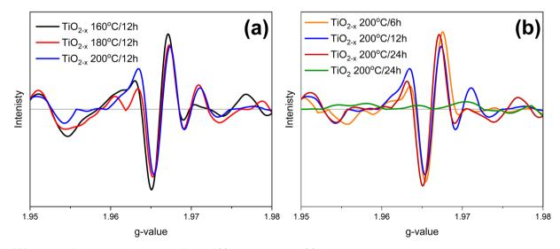
Fig. 6 EPR spectra of the prepared samples; effects of (a) temperature and (b) time.
