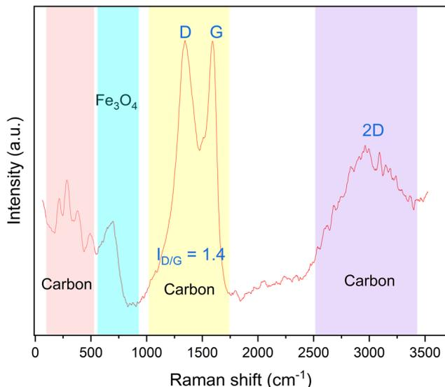
Fig. 9 Raman spectra of the prepared magnetic component.
