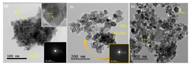
Fig. 10 TEM images of (a) Fe<sub>3</sub>O<sub>4</sub>@g-C and (b) TiO<sub>2-x</sub>/Fe<sub>3</sub>O<sub>4</sub>@g-C 200 °C/24 h 1:1 and (c) TiO<sub>2-x</sub>/Fe<sub>3</sub>O<sub>4</sub>@g-C 200 °C/24 h 4:1.
