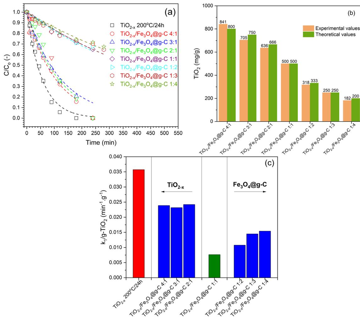
Fig. 13 (a) Experimental data of phenol photocatalytic degradation with 1st order kinetics fitting, (b) ICP analysis of  $\text{TiO}_2$  content in the prepared samples, (c) corrected rate constants based on the  $\text{TiO}_2$  content.
