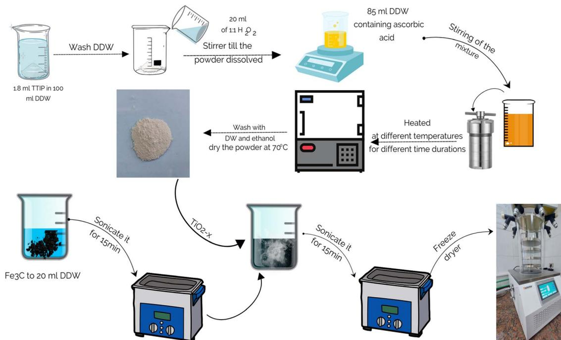
Fig. 1 Schematic preparation scheme of  $\text{TiO}_{2-x}/\text{Fe}_3\text{O}_4@\text{G-C}$ .
