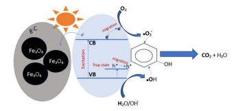
Fig. 14 Photocatalytic mechanism
