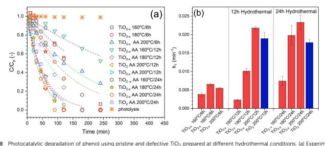
Fig. 8 Photocatalytic degradation of phenol using pristine and defective TiO<sub>2</sub> prepared at different hydrothermal conditions. (a) Experimental data with 1st order kinetics fitting, and (b) comparison of the calculated rate constants [100 mg per L catalyst, 10 mg per L phenol, and natural pH].
