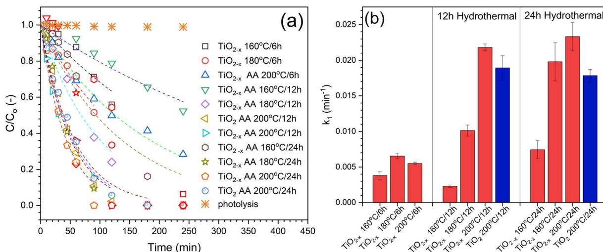
Fig. 8 Photocatalytic degradation of phenol using pristine and defective TiO<sub>2</sub> prepared at different hydrothermal conditions. (a) Experimental data with 1st order kinetics fitting, and (b) comparison of the calculated rate constants [100 mg per L catalyst, 10 mg per L phenol, and natural pH].
