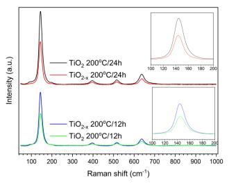
Fig. 4 Raman spectra of  ${\rm TiO_2}$  and  ${\rm TiO_{2-x}}$  prepared at 200 °C in 12 h and 24 h.
