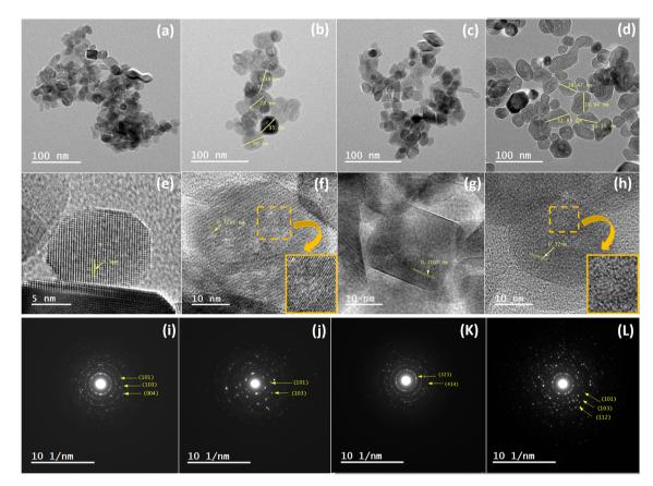
Fig. 5 TEM images of TiO<sub>2</sub> and TiO<sub>2-x</sub> samples: (a, e and i) TiO<sub>2</sub> 200 °C/12 h, (b, f and j) TiO<sub>2-x</sub> 200 °C/12 h, (c, g and k) TiO<sub>2</sub> 200 °C/24 h and (d, h and I) TiO<sub>2-x</sub> 200 °C/24 h.
