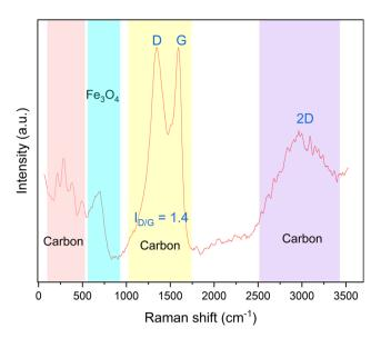
Fig. 9 Raman spectra of the prepared magnetic component.
