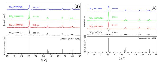
Fig. 2 XRD patterns of pure and defective TiO<sub>2</sub> samples prepared at different (a) temperatures and (b) times.
