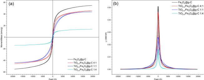
Fig. 11 (a) VSM hysteresis loops and (b) magnetic susceptibility of the pure  $Fe_3O_4@g-C$  and  $TiO_{2-x}/Fe_3O_4@g-C$  composite of different ratios.
