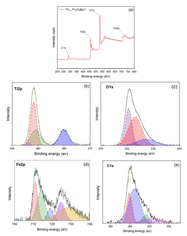
Fig. 12 XPS spectra of the  $TiO_{2-x}/Fe_3O_4@g-C$  1:1 composite; (a) full scan spectrum, (b) Ti 2p, (c) O 1s, (d) Fe 2p and (e) C 1s spectra.
