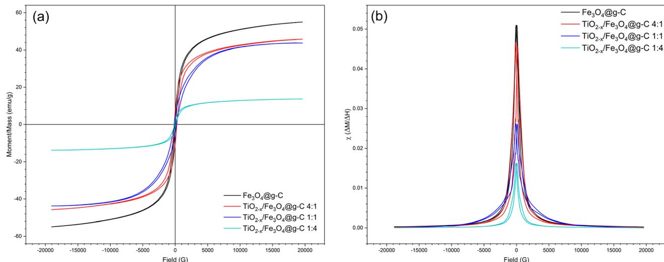
Fig. 11 (a) VSM hysteresis loops and (b) magnetic susceptibility of the pure  $\text{Fe}_3\text{O}_4$ @g-C and  $\text{TiO}_{2-x}/\text{Fe}_3\text{O}_4$ @g-C composite of different ratios.
