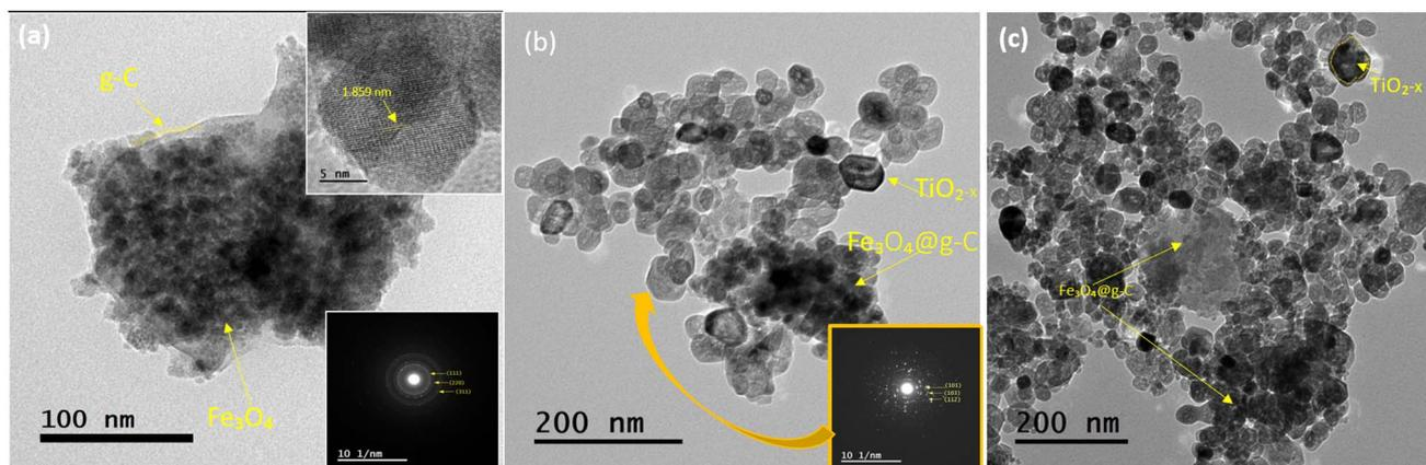
Fig. 10 TEM images of (a)  $\text{Fe}_3\text{O}_4@g\text{-C}$  and (b)  $\text{TiO}_{2-x}/\text{Fe}_3\text{O}_4@g\text{-C}$   $200\text{ }^\circ\text{C}/24\text{ h}$  1 : 1 and (c)  $\text{TiO}_{2-x}/\text{Fe}_3\text{O}_4@g\text{-C}$   $200\text{ }^\circ\text{C}/24\text{ h}$  4 : 1.
