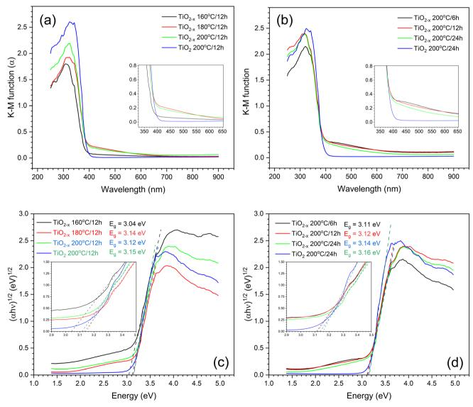
Fig. 3 (a and b) Transformations of the UV-vis DRS spectra, and (c and d) Tauc plot of TiO<sub>2</sub> prepared under different hydrothermal conditions.
