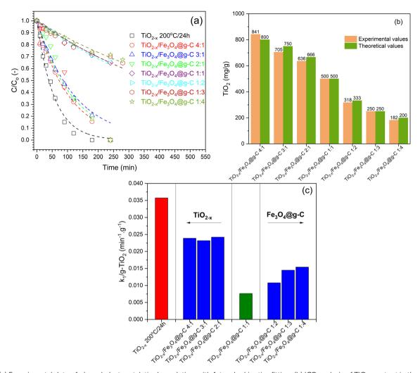
Fig. 13 (a) Experimental data of phenol photocatalytic degradation with 1st order kinetics fitting, (b) ICP analysis of TiO<sub>2</sub> content in the prepared samples, (c) corrected rate constants based on the TiO<sub>2</sub> content.
