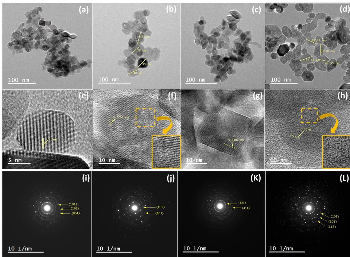
Fig. 5 TEM images of  $\text{TiO}_2$  and  $\text{TiO}_{2-x}$  samples: (a, e and i)  $\text{TiO}_2$  200 °C/12 h, (b, f and j)  $\text{TiO}_{2-x}$  200 °C/12 h, (c, g and k)  $\text{TiO}_2$  200 °C/24 h and (d, h and l)  $\text{TiO}_{2-x}$  200 °C/24 h.
