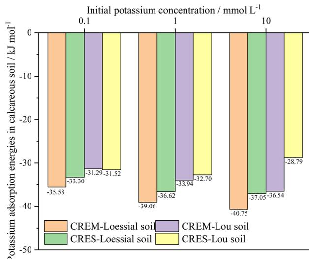
Fig. 5 Adsorption energies of K<sup>+</sup> in calcareous soil at different treatments.
