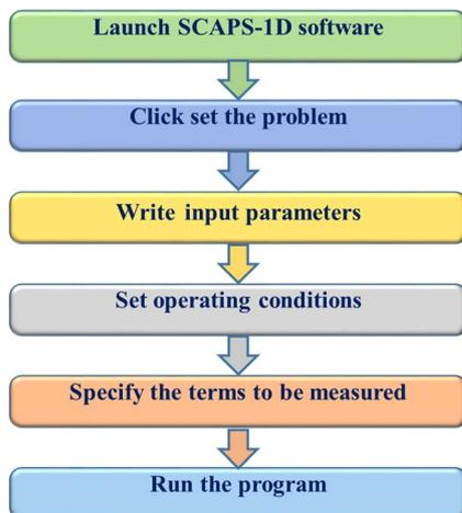
Fig. 1 Schematic of the working approach of the SCAPS-1D simulator.<sup>23</sup>
