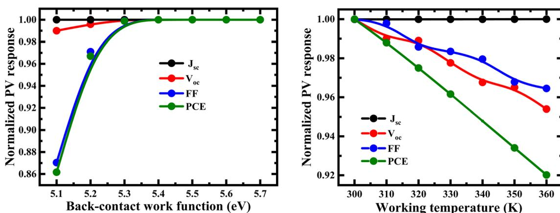
Fig. 10 Key performance parameter responses of the N-doped Cu<sub>2</sub>O/MoTe<sub>2</sub>/ZnO PVSC in relation to (a) work function of the back-contact metal and (b) operating temperature.
