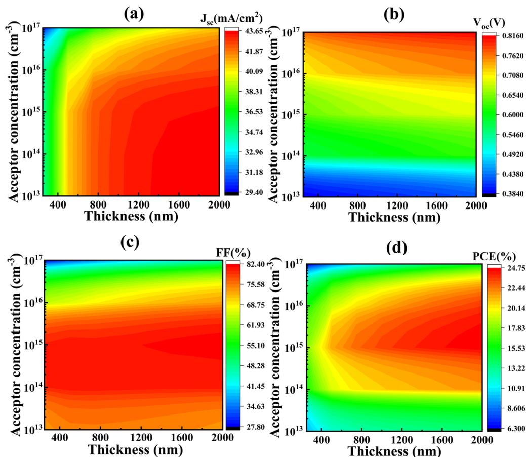
Fig. 3 Contour representations of the variation of (a)  $J_{sc}$ , (b)  $V_{oc}$ , (c) FF, and (d) PCE depending on the width and doping concentration of the MoTe<sub>2</sub> absorber layer. The low to high values of each parameter are indicated by the blue-to-red color coding.
