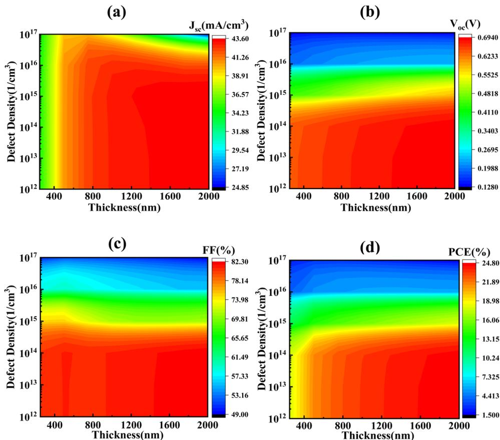
Fig. 4 Contour representations of the variation of (a)  $J_{sc}$ , (b)  $V_{oc}$ , (c) FF, and (d) PCE of the  $\text{MoTe}_2/\text{ZnO}$  device as a function of thickness and defects of the  $\text{MoTe}_2$  layer. The low to high values of each parameter are indicated by the blue-to-red color coding.
