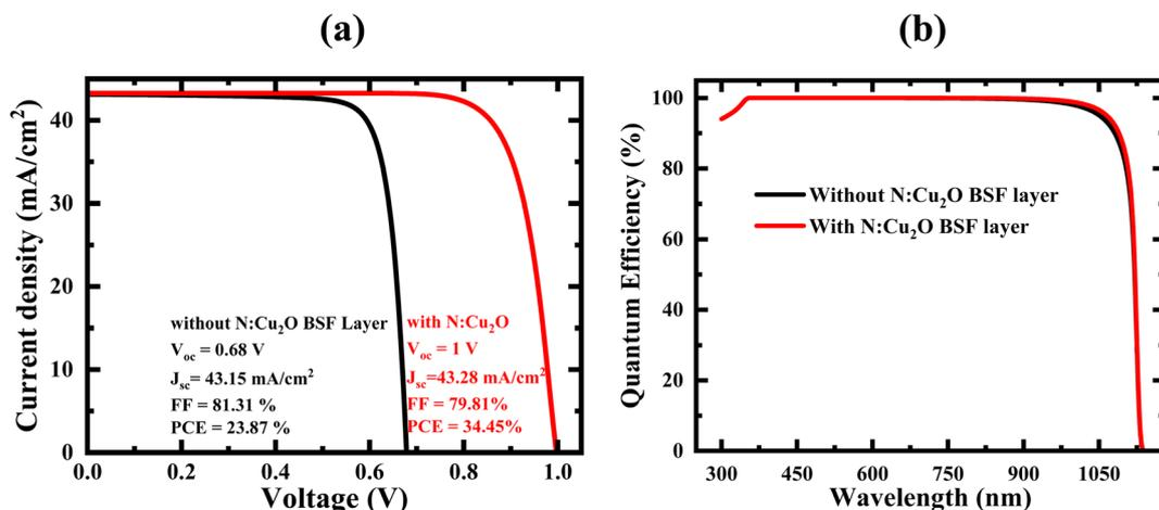
Fig. 9 (a) Light-dependent output characteristic and (b) quantum efficiency curves for the proposed MoTe<sub>2</sub>/ZnO PVSC in the presence and absence of an N-doped Cu<sub>2</sub>O-BSF layer.
