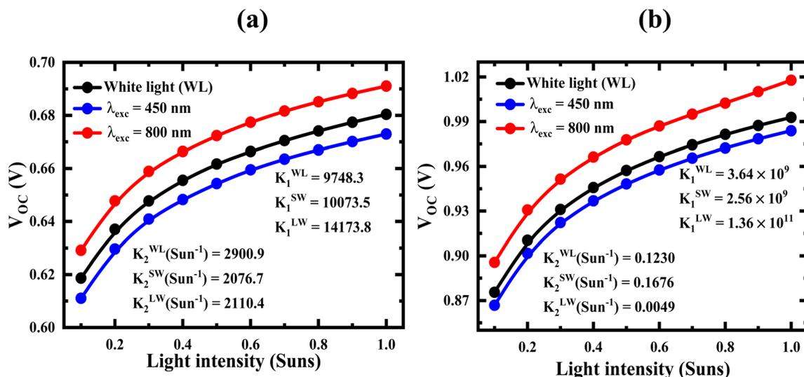
Fig. 8 Light intensity-dependent  $V_{OC}$  for (a) ZnO/MoTe<sub>2</sub> (b) ZnO/MoTe<sub>2</sub>/N-doped Cu<sub>2</sub>O device with different excitation wavelengths of white light (WL),  $\lambda_{exc} = 450$  nm, and  $\lambda_{exc} = 800$  nm at a constant temperature of 300 K.
