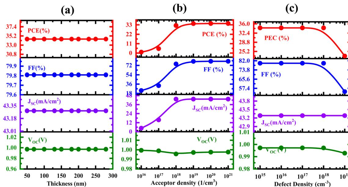
Fig. 6 Dependency of MoTe<sub>2</sub>/ZnO-based PVSC performance on the (a) thickness, (b) donor concentration, and (c) bulk defect density of the N-doped Cu<sub>2</sub>O BSF layer.
