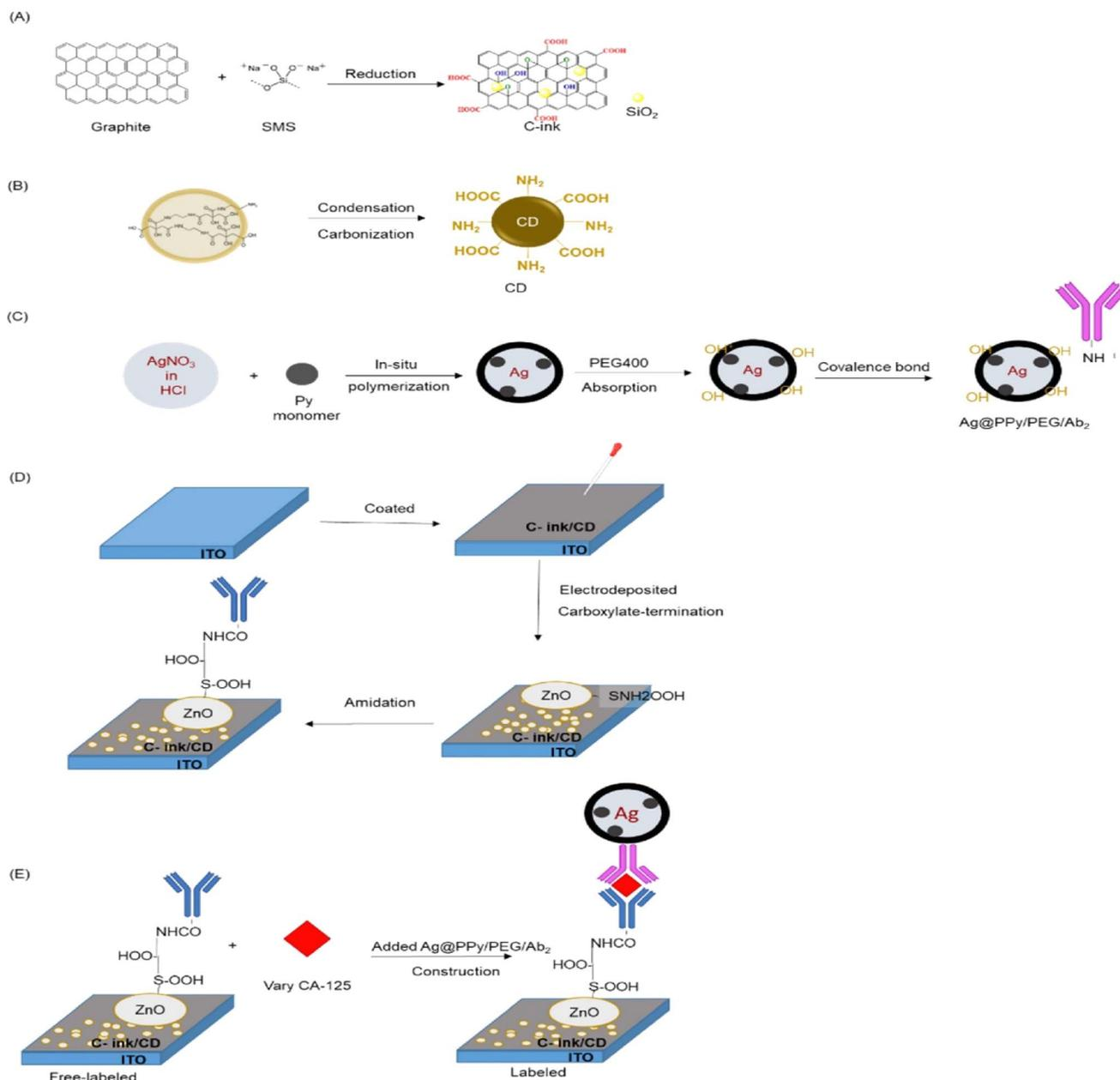
Fig. 8 Preparation steps of materials for CA-125 immunosensor. (A) Synthesis of C-ink and (B) CD. (C) Combined of Ag@PPy/PEG and Ab<sub>2</sub> with covalence bond. (D) Electrode of ITO/C-ink/CD/ZnO/Ab<sub>1</sub> as free-labeled. (E) Construction of ITO/C-ink/CD/ZnO/CA-125 labeled with Ag@PPy/PEG/Ab<sub>2</sub>. "This figure has been adapted from ref. 91 with permission from Elsevier, copyright 2023".
