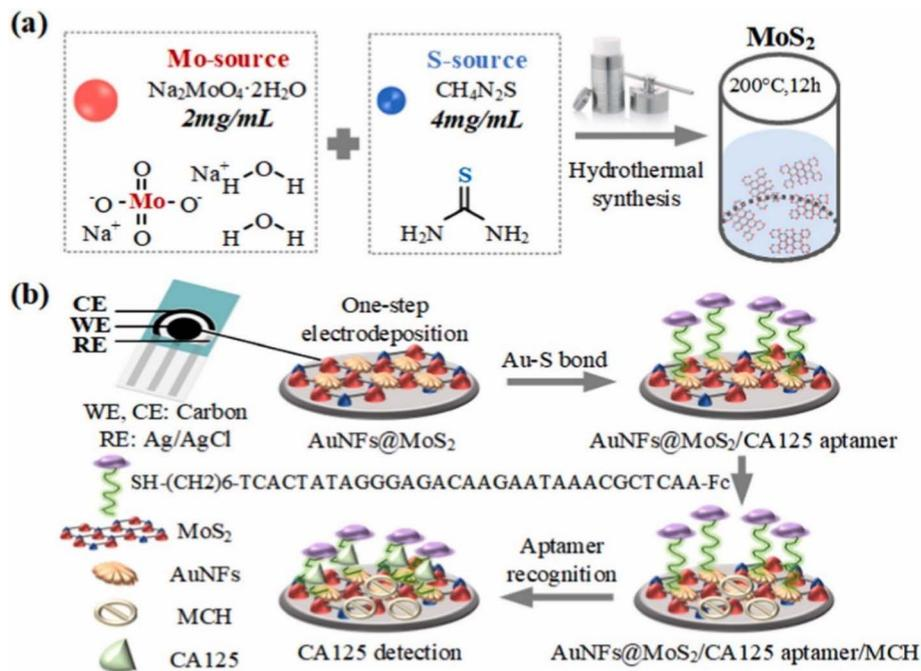
Fig. 7 Schematic diagrams of the sensing platform. (a) Synthesis of MoS<sub>2</sub>. (b) Modification of AuNFs@MoS<sub>2</sub>/CA125 aptamer/MCH for CA125 detection. "This figure has been adapted from ref. 88 with permission from Elsevier, copyright 2023".
