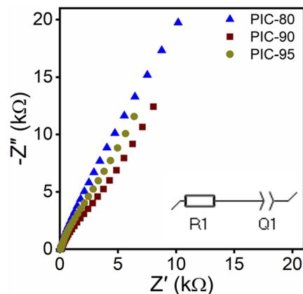
Fig. 5 Nyquist plots of PICs. The inset shows the equivalent circuit model utilized in the extrapolation. R1 and Q1 correspond to the bulk resistance and constant phase element of the composite, respectively.
