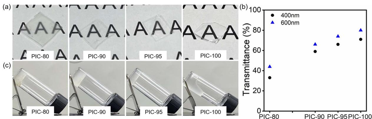
Fig. 1 (a) Photographs of polymer-IL composite (PIC) films (thickness = 0.3 mm). (b) Transmittance of PICs at a wavelength of 400 nm (black dot) and 600 nm (blue triangle). (c) Vial tilt test results after thermal annealing at 40 °C for 36 h.
