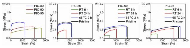
Fig. 3 Stress-strain curves of (a) pristing and (b-d) self-healed PIC samples. Self-healing was conducted at room temperature for 6 h (green), 24 h (red), and at 65 °C for 2 h (blue)
