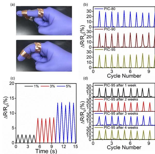
Fig. 6 (a) Photographs of the PIC-95 strain sensor attached to a finger before and after bending. (b) Relative resistance changes for PICs during repeated bending and extension of the finger. (c)  $\Delta R/R_0$  as a function of the imposed tensile strains for PIC-95. (d) Operation of the PIC-95 strain sensor over 4 weeks.
