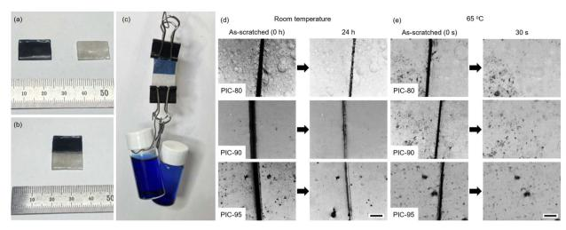
Fig. 4 Dyed and non-dyed PIC-95 specimens (a) before and (b) after self-healing (RT, 24 h). (c) Self-healed PIC-95 withstood a weight of 50 g. (d and e) Optical microscope images of scratched PIC-80, PIC-90, and PIC-95 monitored after (d) 24 h at RT and (e) 30 s at 65 °C. The scale bars correspond to 100  $\mu$ m.
