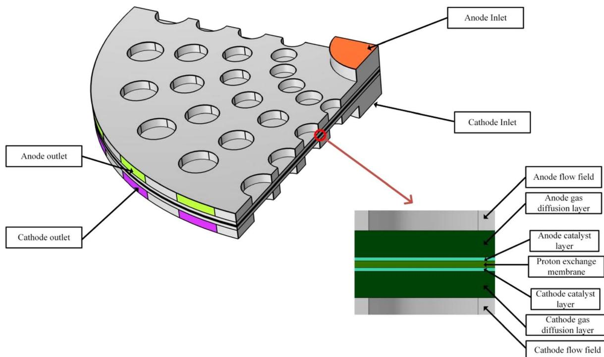
Fig. 1 Three-dimensional geometric model of the lattice-type radial flow field.
