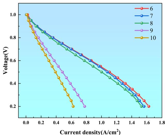
Fig. 11 Polarization curves for Case 6 to Case 10.
