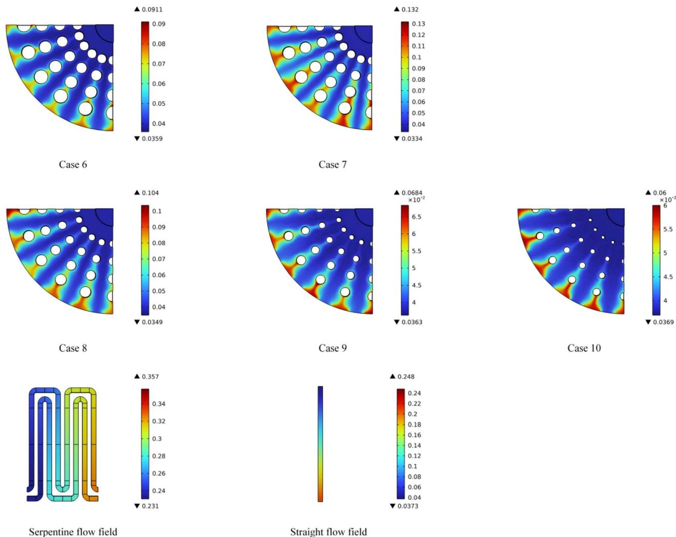
Fig. 14 The water distribution in the flow field cross-section for Case 6 to Case 10 and two types of conventional flow fields.
