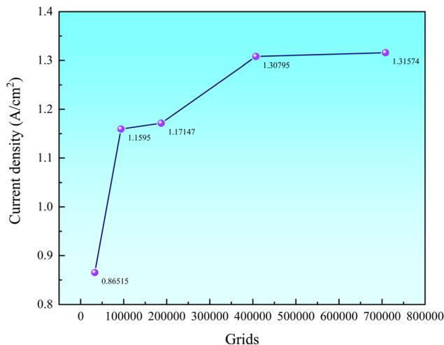
Fig. 2 Verification of grid independence at 0.4 V voltage.
