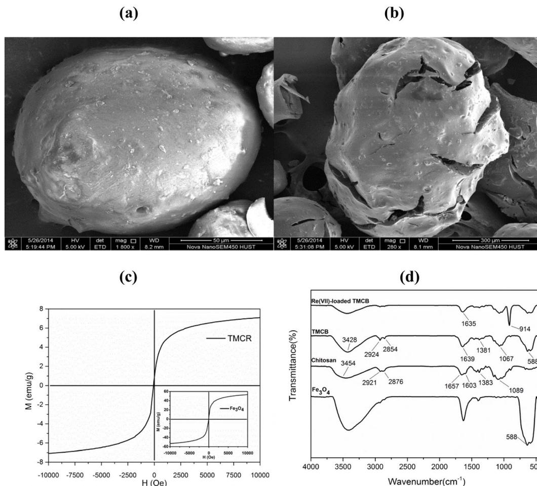
Fig. 1 SEM images of MCB (1800 $\times$ ) (a) and TMCB (280 $\times$ ) (b); VSM magnetization curves of TMCB and Fe<sub>3</sub>O<sub>4</sub> (c); FTIR spectra of Fe<sub>3</sub>O<sub>4</sub>, chitosan, TMCB and Re(vii)-loaded TMCB (d).
