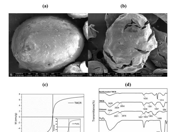
Fig. 1 SEM images of MCB (1800 $\times$ ) (a) and TMCB (280 $\times$ ) (b); VSM magnetization curves of TMCB and Fe<sub>3</sub>O<sub>4</sub> (c); FTIR spectra of Fe<sub>3</sub>O<sub>4</sub>, chitosan, TMCB and Re( $v_1$ )-loaded TMCB (d).
