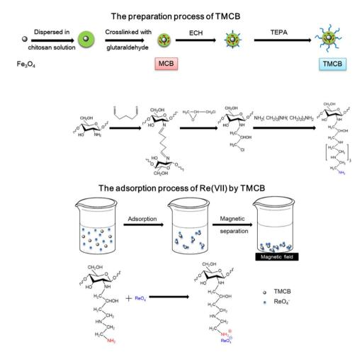
Scheme 1 Schematics of the preparation process of the TMCB and the adsorption process of Re(vii) by the TMCB.
