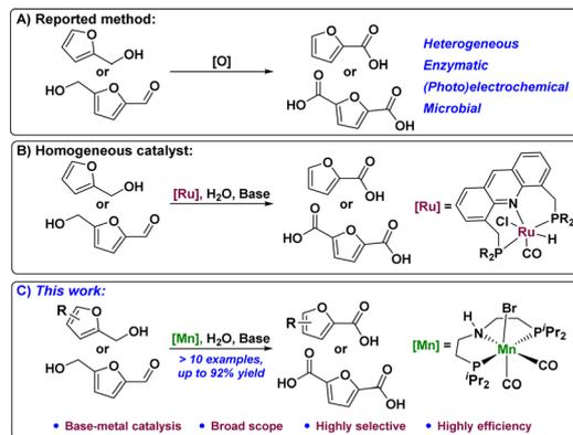
**Fig. 1** (A) The reported method for the oxidation of furfuryl alcohols to furoic acids. (B) Homogeneous catalytic oxidation of furfuryl alcohols to furoic acid. (C) Mn-catalyzed oxidation of furfuryl alcohol to furoic acid.
