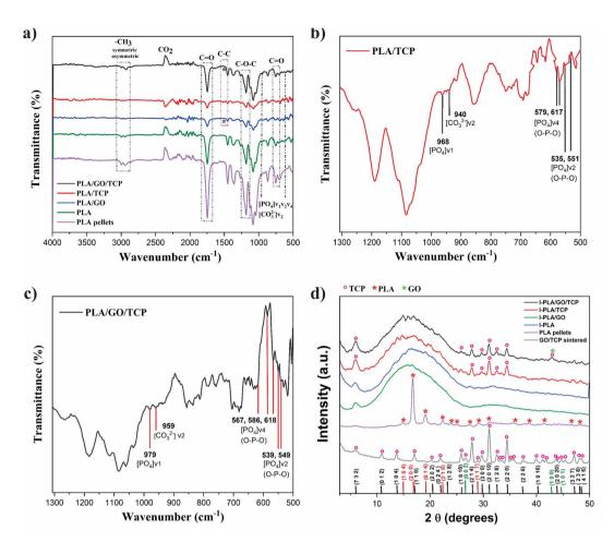
Fig. 2 FTIR spectra for PLA pellets and 3D scaffolds PLA, PLA/GO, PLA/TCP and PLA/GO/TCP (a), TCP characteristic bands are evident in PLA/TCP (b) and PLA/GO/TCP (c); XRD of GO/TCP sintered for one hour, PLA pellets and PLA, PLA/GO, PLA/TCP and PLA/GO/TCP 3D scaffolds (d).
