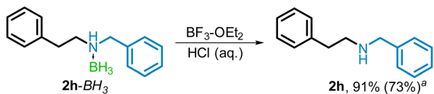
Scheme 6 Conversion of borane-amine to free amine. a Yield of 2h when amidation, reduction and removal of \text{BH}_3 are carried out sequentially in a one-pot reaction.
