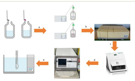
Fig. 1 The measurements diagram including preparation of mixtures and sonication (a), UV-Vis spectrophotometry (b), dynamic light scattering (c), density and speed of sound measurements (d), and viscosity measurement (e).
