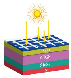
Fig. 1 Proposed CIGS solar cell with Sb<sub>2</sub>S<sub>3</sub> BSF layer.
