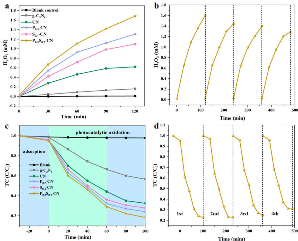
Fig. 5 (a) Photocatalytic production of H<sub>2</sub>O<sub>2</sub> by various photocatalysts, (b) 50 mg photocatalyst for 4 consecutive cycles of H<sub>2</sub>O<sub>2</sub> production, (c) photocatalytic oxidative degradation of TC (20 mg L<sup>-1</sup>) by multifarious catalysts (30 mg), and (d) 30 mg photocatalyst employed for 4 consecutive cycles of TC degradation.
