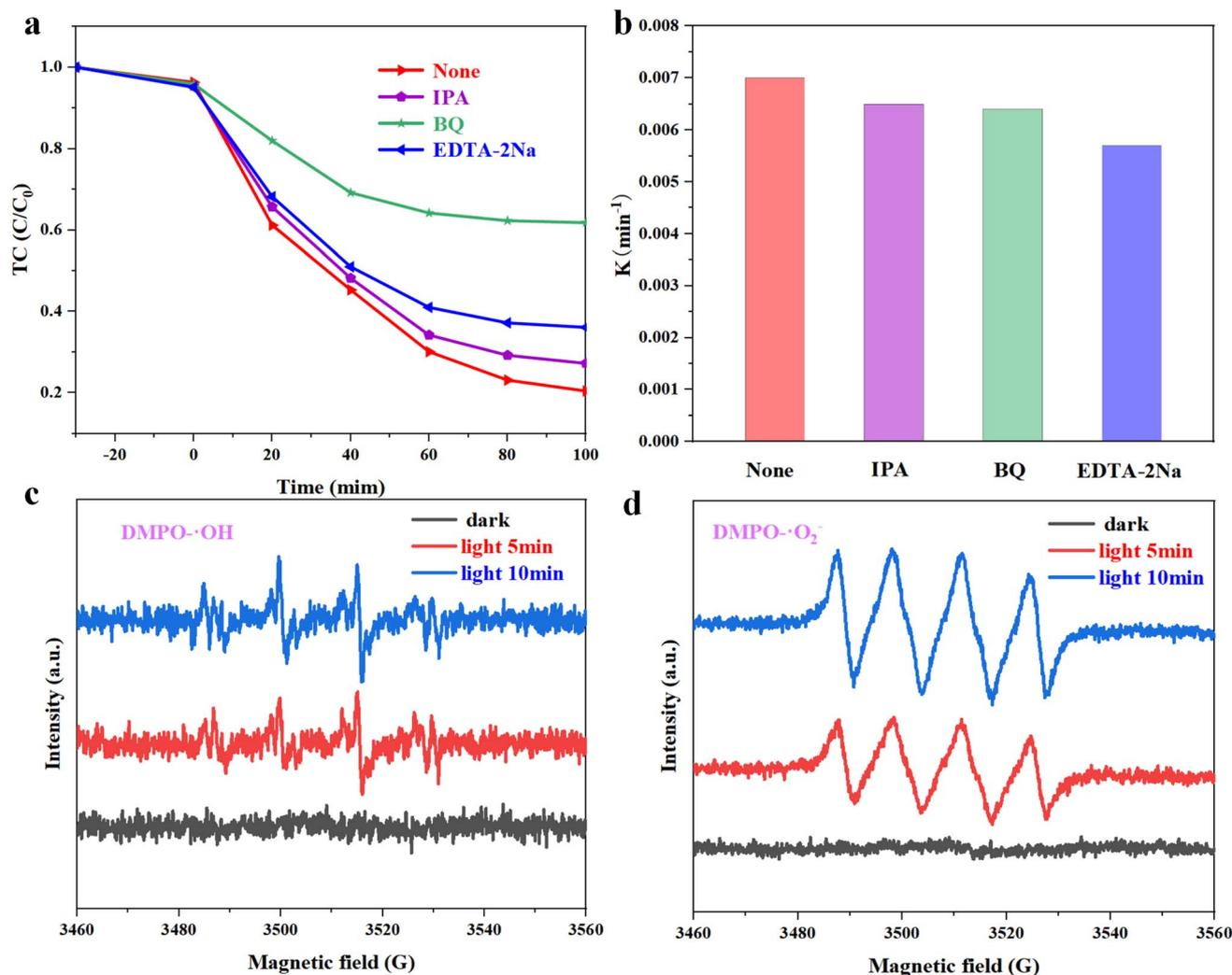
Fig. 9 Under visible light irradiation and added scavenger conditions, (a) TC and (b) corresponding kinetic constants of  $P_{0.3}S_{0.2}$ -CN degradation and EPR spectra of  $P_{0.3}S_{0.2}$ -CN in the dark and under visible light irradiation with (c)  $DMPO\cdot OH$  and (d)  $DMPO\cdot O_2^-$ .
