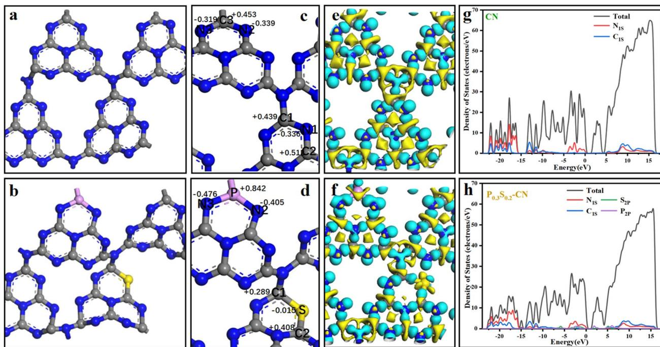
Fig. 7 The optimized structures of the (a) CN and (b)  $P_{0.3}S_{0.2}$ -CN; the DFT-computed atomic charges at the (c) CN and (d)  $P_{0.3}S_{0.2}$ -CN doping sites are provided near each atom. The differential charge density plots of (e) CN and (f)  $P_{0.3}S_{0.2}$ -CN. DOS plots of (g) CN and (h)  $P_{0.3}S_{0.2}$ -CN.
