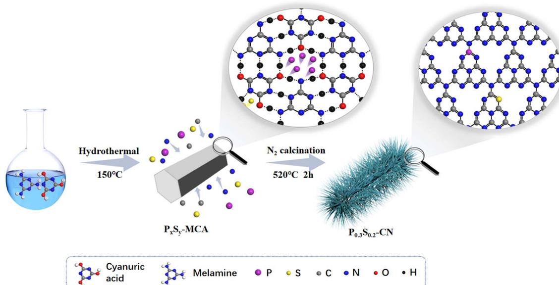
Fig. 1 Schematic depiction of the fabrication process of P<sub>x</sub>S<sub>y</sub>-CN.
