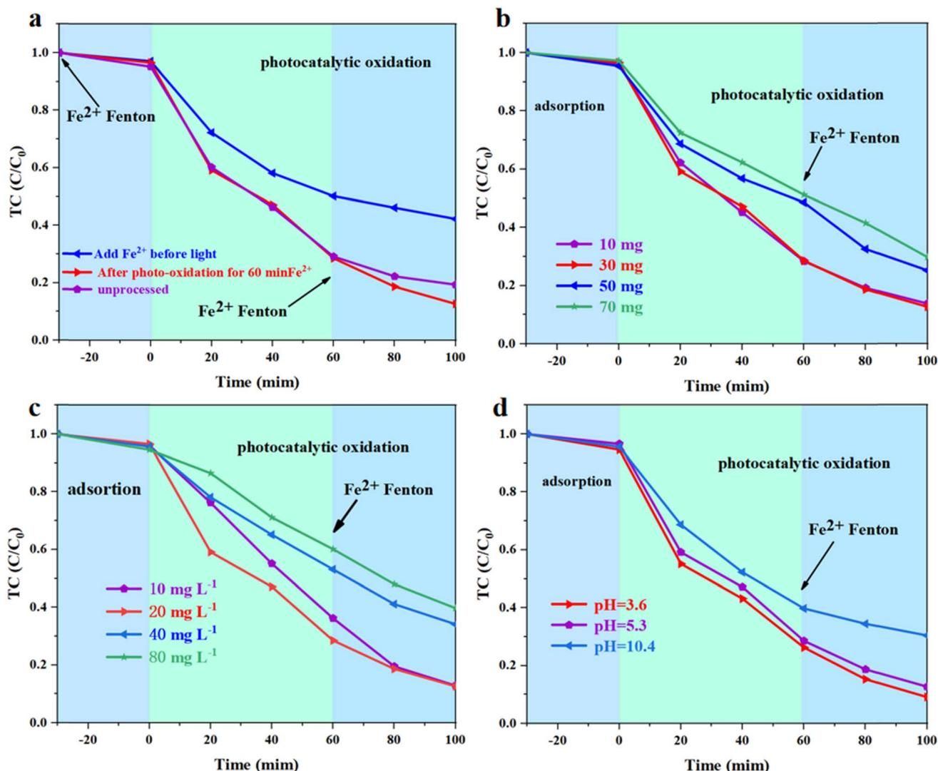
Fig. 6 Under visible light irradiation, effect of (a) Fe<sup>2+</sup> addition on the photocatalytic degradation of TC by P<sub>0.3</sub>S<sub>0.2</sub>-CN, (b) dosage of the P<sub>0.3</sub>S<sub>0.2</sub>-CN catalyst, (c) initial concentration of TC, (d) different pH values on photocatalytic oxidation-Fenton oxidative degradation.
