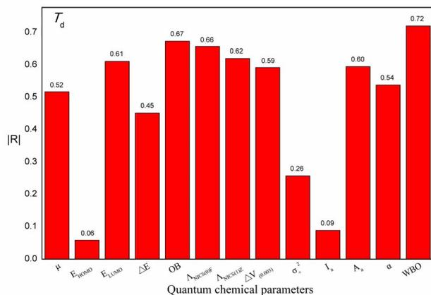
Fig. 4 Absolute values of the correlation coefficients ( $|R|$ ) between chemical parameters and experimental thermal decomposition temperature ( $T_d$ ).
