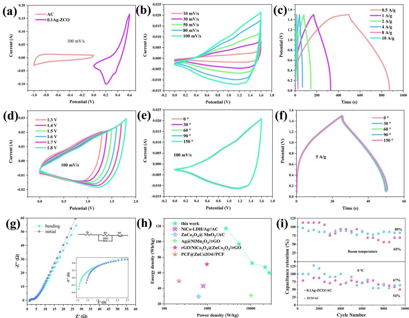
Fig. 4 Electrochemical performance of the ASC device. (a) CV curves of the electrodes at  $100$   $\text{mV s}^{-1}$ , (b) CV curves at various scan rates, (c) GCD curves at various current densities, (d) CV curves in different potential windows at  $100$   $\text{mV s}^{-1}$ , and CV (e) and GCD (f) curves at various bending angles, (g) Nyquist plots, (h) Ragone plots, and (i) cycling performance at  $5$   $\text{A g}^{-1}$ .
