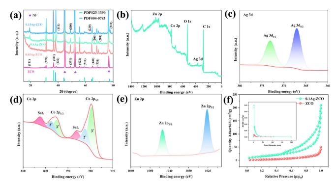
Fig. 1 Structure characterization of the as-prepared materials. (a) XRD patterns of the electrode materials, (b) XPS full spectrum of ZCSN-2, (c-e) XPS spectra of Ag 3d Co 2p and 2 Zn p and (f)  $N_2$  adsorption-desorption isotherms and corresponding pore-size distribution curves (inset) of ZCO and 0.01Ag-ZCO.
