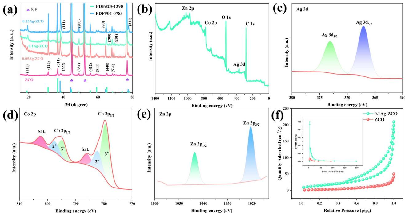
Fig. 1 Structure characterization of the as-prepared materials. (a) XRD patterns of the electrode materials, (b) XPS full spectrum of ZCSN-2, (c–e) XPS spectra of Ag 3d, Co 2p and 2 Zn p and (f)  $N_2$  adsorption–desorption isotherms and corresponding pore-size distribution curves (inset) of ZCO and 0.01Ag-ZCO.
