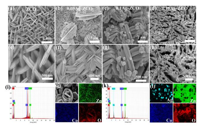
Fig. 2 Morphology of the samples. SEM images of (a and e) ZCO, (b and f) 0.05Ag-ZCO, (c and g) 0.05Ag-ZCO, (d and h) 0.05Ag-ZCO. (i-I) EDS pattern and elemental mapping images of the ZCO and 0.05Ag-ZCO samples.
