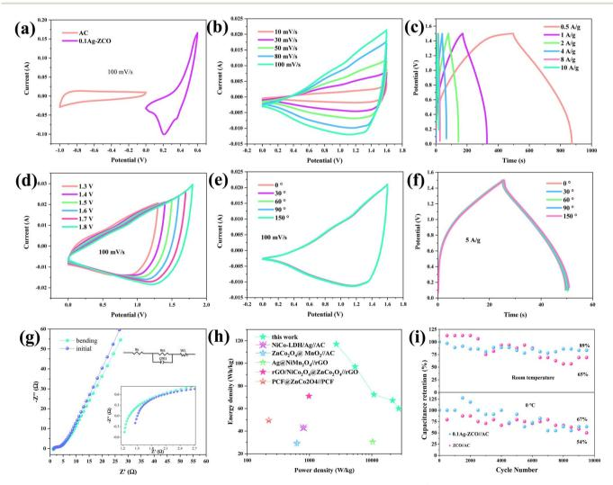
Fig. 4 Electrochemical performance of the ASC device. (a) CV curves of the electrodes at 100 mV s<sup>-1</sup>, (b) CV curves at various scan rates, (c) GCD curves at various current densities, (d) CV curves in different potential windows at 100 mV s<sup>-1</sup>, and CV (e) and GCD (f) curves at various bending angles, (g) Nyquist plots, (h) Ragone plots, and (i) cycling performance at 5 A  $g^{-1}$ .
