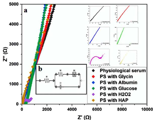
Fig. 7 (a) EIS of  $\alpha$ -titanium in different solutions: saline solution, amino acid medium (glycin  $0.09 \text{ g L}^{-1}$ ), protein medium (albumin  $40 \text{ g L}^{-1}$ ) and glucose ( $0.85 \text{ g L}^{-1}$ ),  $\text{H}_2\text{O}_2$  ( $35 \text{ }\mu\text{M}$ ) hydroxyapatite ( $0.1 \text{ g L}^{-1}$ ) at  $37^\circ \text{C}$ , and EIS at high frequency of the six media, (b) equivalent circuit used to fit the experimental data.
