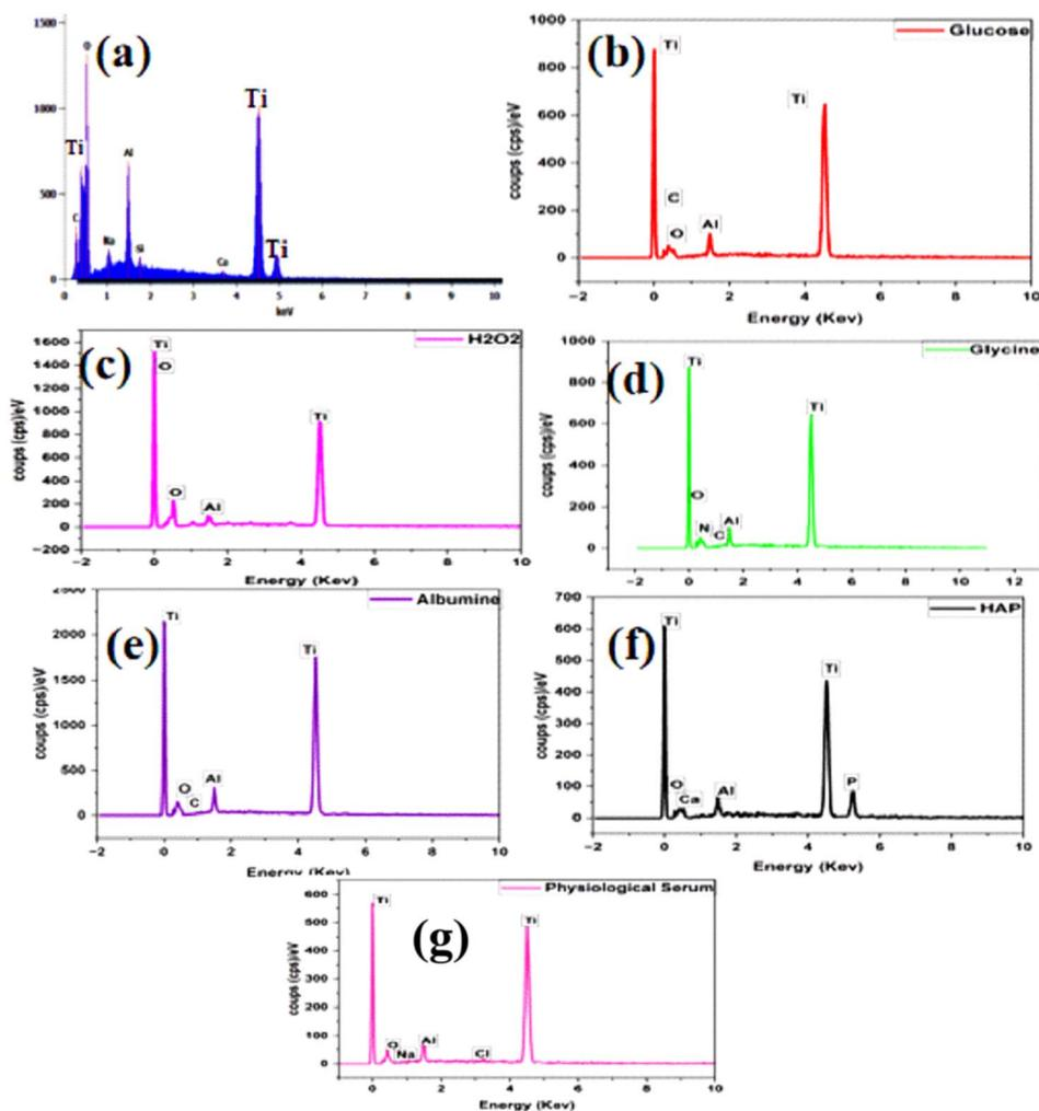
Fig. 9 EDS analysis of titanium alloy after immersion in solutions for 168 h: (a) titanium alloy before immersion and (b) titanium alloy immersed in SP with glucose, (c) titanium alloy immersed in SP with H<sub>2</sub>O<sub>2</sub> and (d) Titanium alloy immersed in SP with glycine (e) titanium alloy immersed in SP with albumin and (f) titanium alloy immersed in SP with hydroxyapatite, (g) titanium alloy immersed in SP.
