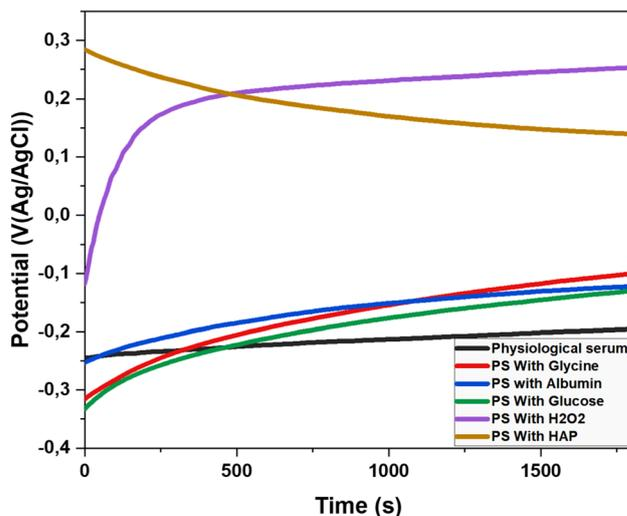
Fig. 5 Open-circuit potential curves for Titanium alloy in different solutions: saline solution, amino acid medium (glycine 0.09 g L<sup>-1</sup>), protein medium (Albumin 40 g L<sup>-1</sup>) and glucose (0.85 g L<sup>-1</sup>), H<sub>2</sub>O<sub>2</sub> (35 μM) hydroxyapatite (0.1 g L<sup>-1</sup>) at 37 °C.
