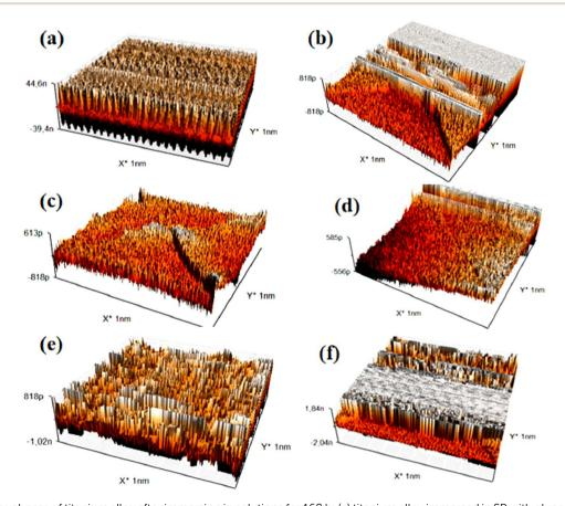
Fig. 10 Surface roughness of titanium alloy after immersion in solutions for 168 h: (a) titanium alloy immersed in SP with glucose and (b) titanium alloy immersed in SP with  $H_2O_2$ , (c) titanium alloy immersed in SP with glycine and (d) titanium alloy immersed in SP with albumin (e) titanium alloy immersed in SP with hydroxyapatite and (f) titanium alloy immersed in SP.
