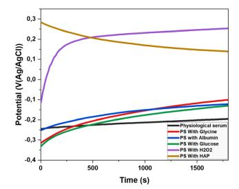
Fig. 5 Open-circuit potential curves for Titanium alloy in different solutions: saline solution, amino acid medium (glycine  $0.09 \text{ g L}^{-1}$ ), protein medium (Albumin 40 g L<sup>-1</sup>)and glucose (0.85 g L<sup>-1</sup>), H<sub>2</sub>O<sub>2</sub> (35  $\mu$ M) hydroxyapatite (0.1 g L<sup>-1</sup>) at 37 °C.
