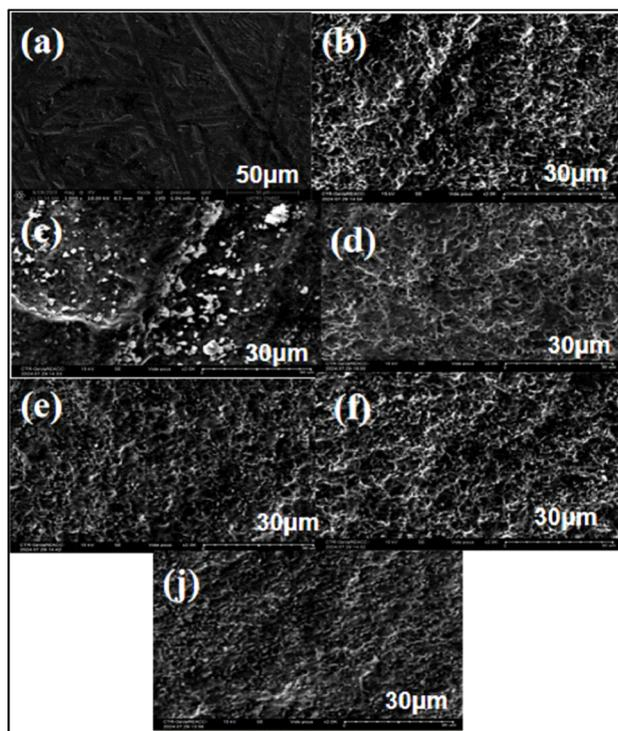
Fig. 8 Surface morphology following corrosion of titanium alloy after immersion in solutions for 168 h: (a) titanium alloy before immersion and (b) titanium alloy immersed in SP with glucose, (c) titanium alloy immersed in SP with  $\text{H}_2\text{O}_2$  and (d) titanium alloy immersed in SP with glycine (e) titanium alloy immersed in SP with albumin and (f) titanium alloy immersed in SP with hydroxyapatite, (g) titanium alloy immersed in SP.
