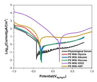
Fig. 6 Potentiodynamic polarization curves for Titanium alloy in different media solutions: Saline solution, amino acid medium (glycine 0.09 g L $^{-1}$ ), protein medium (albumin 40 g L $^{-1}$ ) and glucose (0.85 g L $^{-1}$ ), H<sub>2</sub>O<sub>2</sub> (35  $\mu$ M) hydroxyapatite (0.1 g L $^{-1}$ ) at 37 °C.
