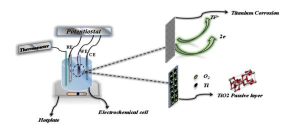
Fig. 3 Electrochemical experimental set-up.
