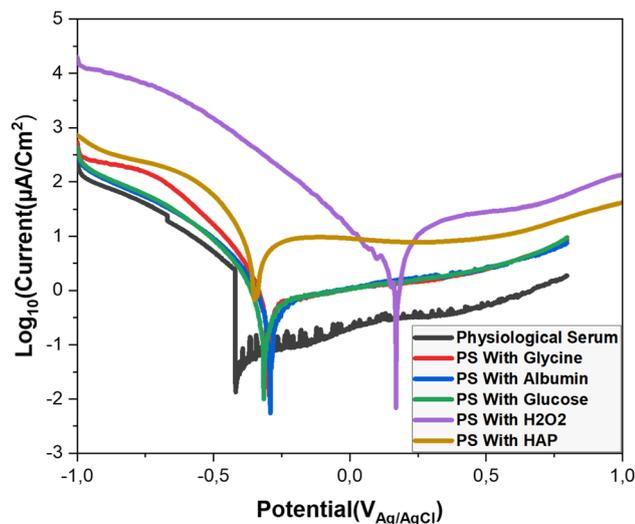
Fig. 6 Potentiodynamic polarization curves for Titanium alloy in different media solutions: Saline solution, amino acid medium (glycine  $0.09 \text{ g L}^{-1}$ ), protein medium (albumin  $40 \text{ g L}^{-1}$ ) and glucose ( $0.85 \text{ g L}^{-1}$ ),  $\text{H}_2\text{O}_2$  ( $35 \text{ }\mu\text{M}$ ) hydroxyapatite ( $0.1 \text{ g L}^{-1}$ ) at  $37 \text{ }^\circ\text{C}$ .
