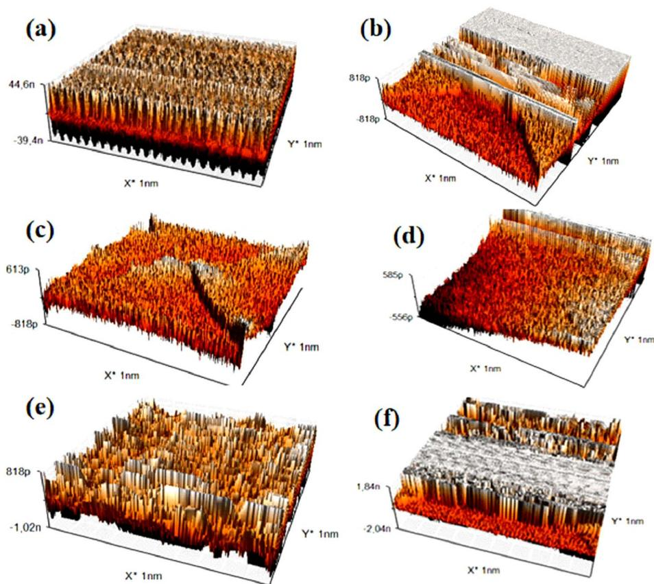
Fig. 10 Surface roughness of titanium alloy after immersion in solutions for 168 h: (a) titanium alloy immersed in SP with glucose and (b) titanium alloy immersed in SP with H<sub>2</sub>O<sub>2</sub>, (c) titanium alloy immersed in SP with glycine and (d) titanium alloy immersed in SP with albumin (e) titanium alloy immersed in SP with hydroxyapatite and (f) titanium alloy immersed in SP.
