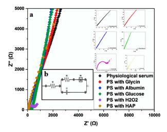
Fig. 7 (a) EIS of  $\alpha$ -titanium in different solutions: saline solution, amino acid medium (glycin 0.09 g L $^{-1}$ ), protein medium (albumin 40 g L $^{-1}$ ) and glucose (0.85 g L $^{-1}$ ), H $_2$ O $_2$  (35  $_\mu$ M) hydroxyapatite (0.1 g L $^{-1}$ ) at 37 °C, and EIS a high frequency of the six media, (b) equivalent circuit used to fit the experimental data.
