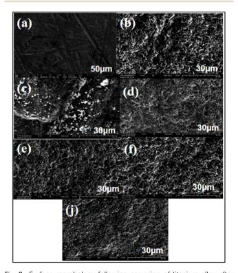
Fig. 8 Surface morphology following corrosion of titanium alloy after immersion in solutions for 168 h: (a) titanium alloy before immersion and (b) titanium alloy immersed in SP with glucose, (c) titanium alloy immersed in SP with  $H_2O_2$  and (d) titanium alloy immersed in SP with glycine (e) titanium alloy immersed in SP with albumin and (f) titanium alloy immersed in SP.
