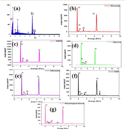
Fig. 9 EDS analysis of titanium alloy after immersion in solutions for 168 h: (a) titanium alloy before immersion and (b) titanium alloy immersed in SP with glucose, (c) titanium alloy immersed in SP with  $H_2O_2$  and (d) Titanium alloy immersed in SP with glycine (e) titanium alloy immersed in SP with albumin and (f) titanium alloy immersed in SP with hydroxyapatite, (g) titanium alloy immersed in SP.
