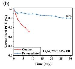
Fig. 7 Stability tests of unsealed control and Pyr-mediated FPSCs (a) in humid ambient air in dark condition and (b) in ambient air under simulated light irradiance.
