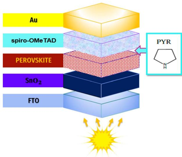
Fig. 1 Proposed perovskite solar cell structure.
