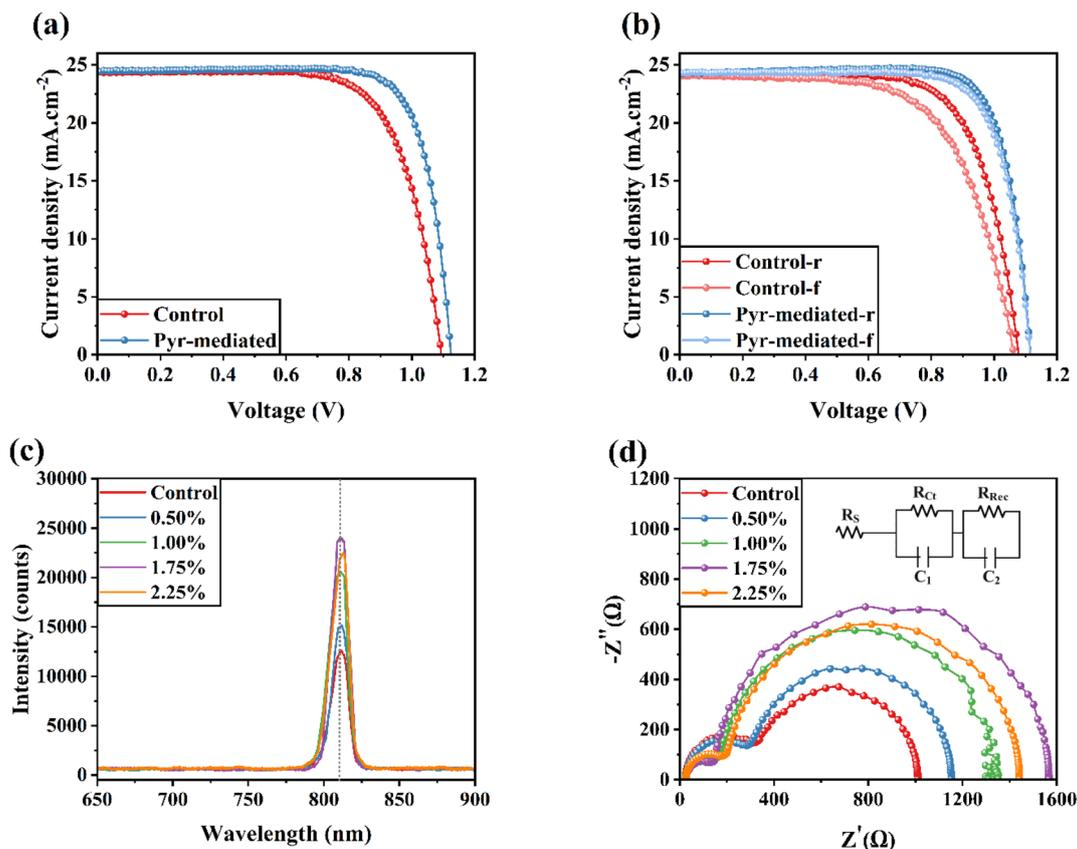
Fig. 2 (a)  $J$ - $V$  curves of the optimized FSCs based on control and Pyr-mediated perovskite layers. (b)  $J$ - $V$  curves of typical FSCs in reverse and forward directions in each group. (c) PL spectra of different perovskite layers fabricated on glass substrates. (d) EIS responses of different FSCs measured at open-circuit voltage in dark conditions. Inset of (d) shows equivalent electrical circuit to fit Nyquist plots.
