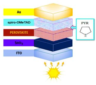
Fig. 1 Proposed perovskite solar cell structure.
