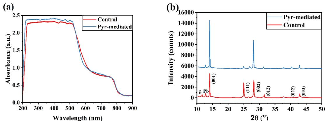
Fig. 5 (a) Absorbance spectra and (b) XRD patterns of control and Pyr-mediated perovskite layers.
