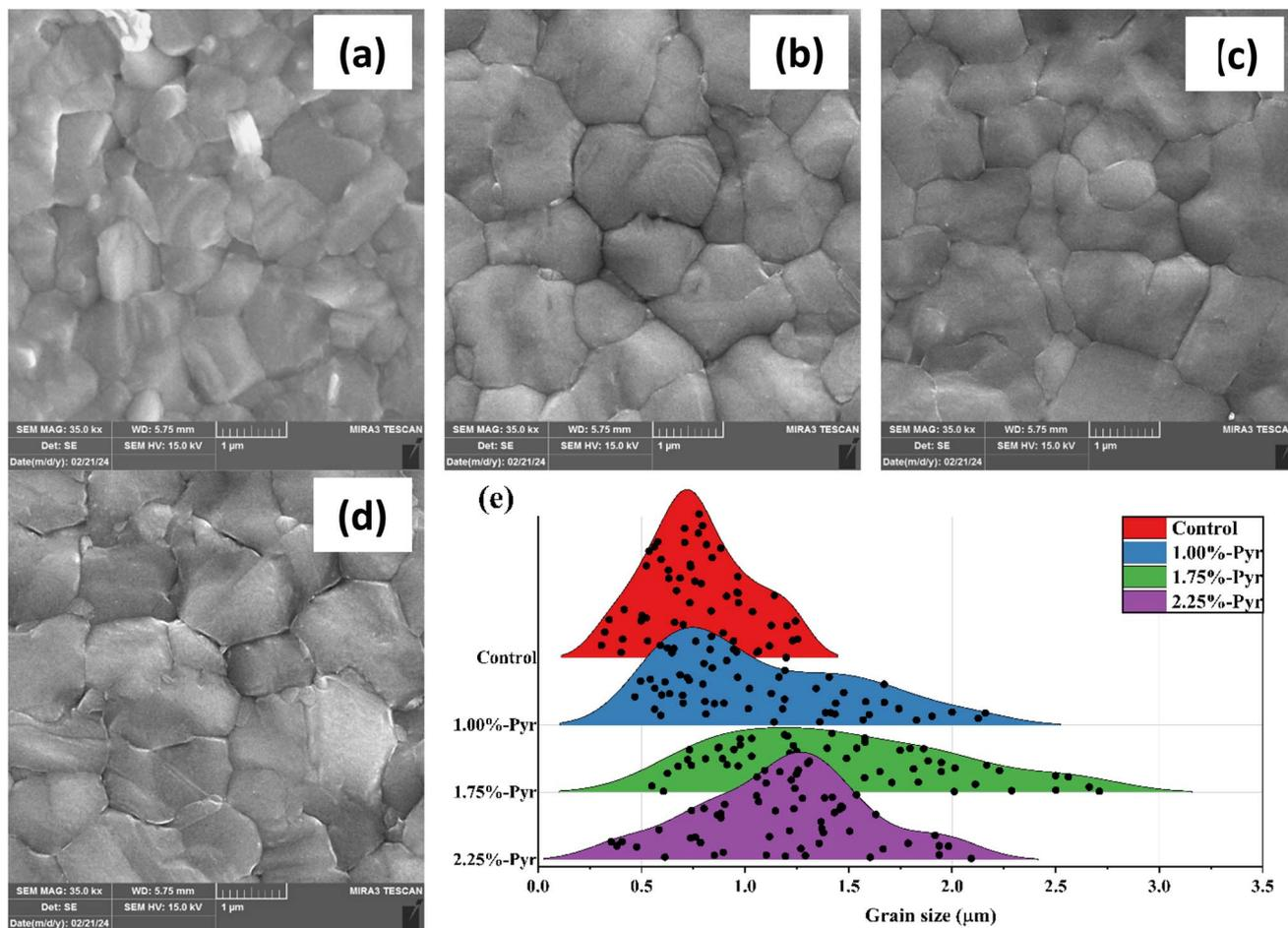
Fig. 3 FESEM images of (a) control, (b) 1.00%-, (c) 1.75%-, and (d) 2.25%-Pyr based perovskite layers. (e) Grain size distributions of different perovskite layers.
