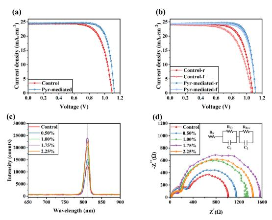
Fig. 2 (a) J-V curves of the optimized FSCs based on control and Pyr-mediated perovskite layers. (b) J-V curves of typical FSCs in reverse and forward directions in each group. (c) PL spectra of different perovskite layers fabricated on glass substrates. (d) EIS responses of different FSCs measured at open-circuit voltage in dark conditions. Inset of (d) shows equivalent electrical circuit to fit Nyquist plots.
