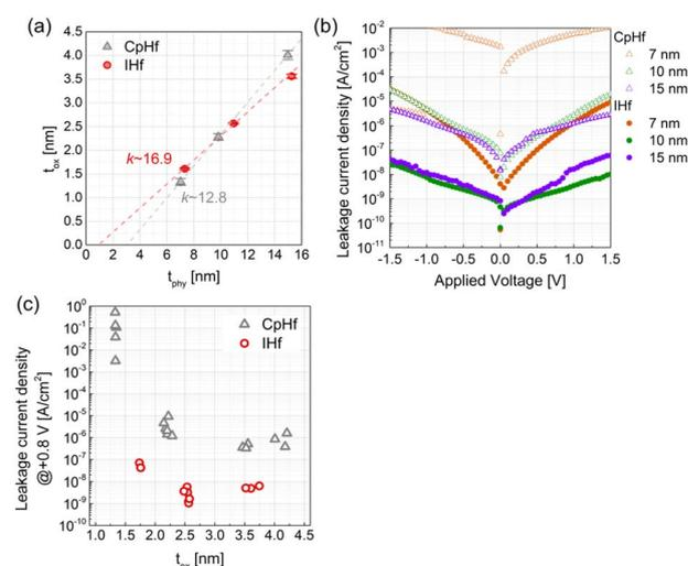
Fig. 4 (a)  $t_{\text{phy}}-t_{\text{ox}}$  plot, (b)  $J-V$  curves, and (c)  $J-t_{\text{ox}}$  plot of HfO<sub>2</sub> thin films varied thicknesses using CpHf and IHf precursors.
