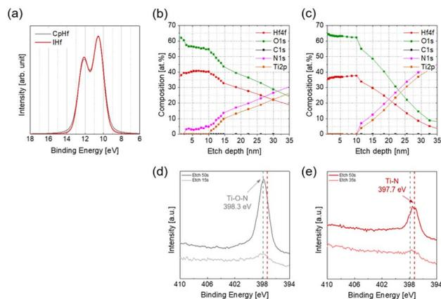
Fig. 3 (a) Hf 4f spectra of  $10 \text{ nm}$ -thick  $\text{HfO}_2$  thin films deposited using CpHf and IHf precursors. (b and c) Depth profile of  $10 \text{ nm}$ -thick  $\text{HfO}_2$  thin films deposited using (b) CpHf, and (c) IHf. (d and e) N 1s spectra obtained at each etch time from  $\text{HfO}_2$  thin films deposited using (d) CpHf, and (e) IHf.
