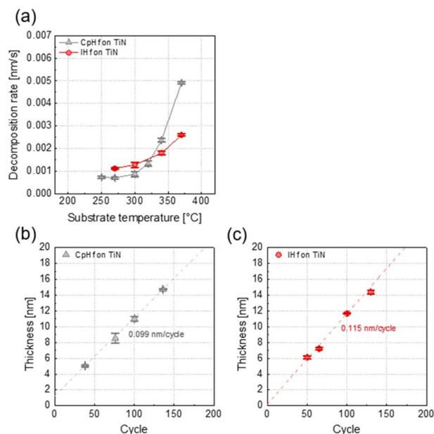
Fig. 1 (a) Thermal decomposition of CpHf and IHf precursors. Linear growth behavior of HfO<sub>2</sub> thin film deposition processes using (b) CpHf + O<sub>3</sub> and (c) IHf + O<sub>3</sub>.
