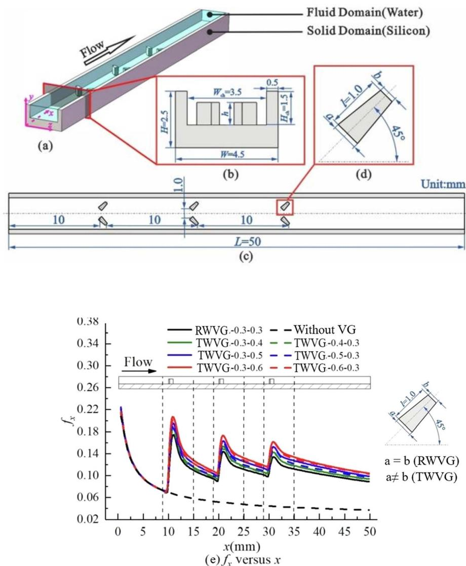
Fig. 9 Schematic diagrams of (a) the computational domain of mini-channel, (b) sectional side-view, (c) top-view and (d) TWVG.<sup>62</sup> (e) The deviations in local fanning friction factor along the flow direction for MCW with trapezoidal VG and smooth micro channel. Reproduced with permission<sup>62</sup> copyright © 2022 Elsevier.
