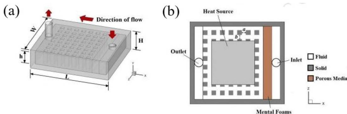
Fig. 10 Structure diagram of micro square pin-fin heat sinks (a) external view. (b) Bottom view. Reproduced with permission<sup>137</sup> copyright © 2015 Elsevier.
