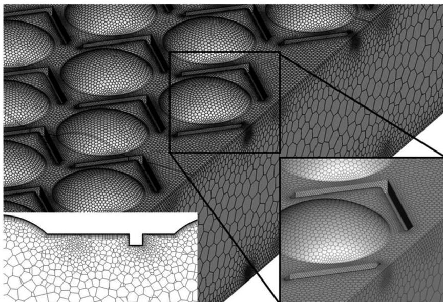
Fig. 13 The geometry of deep dimple tube. Reproduced with permission<sup>166</sup> copyright © 2023 Elsevier Masson SAS.
