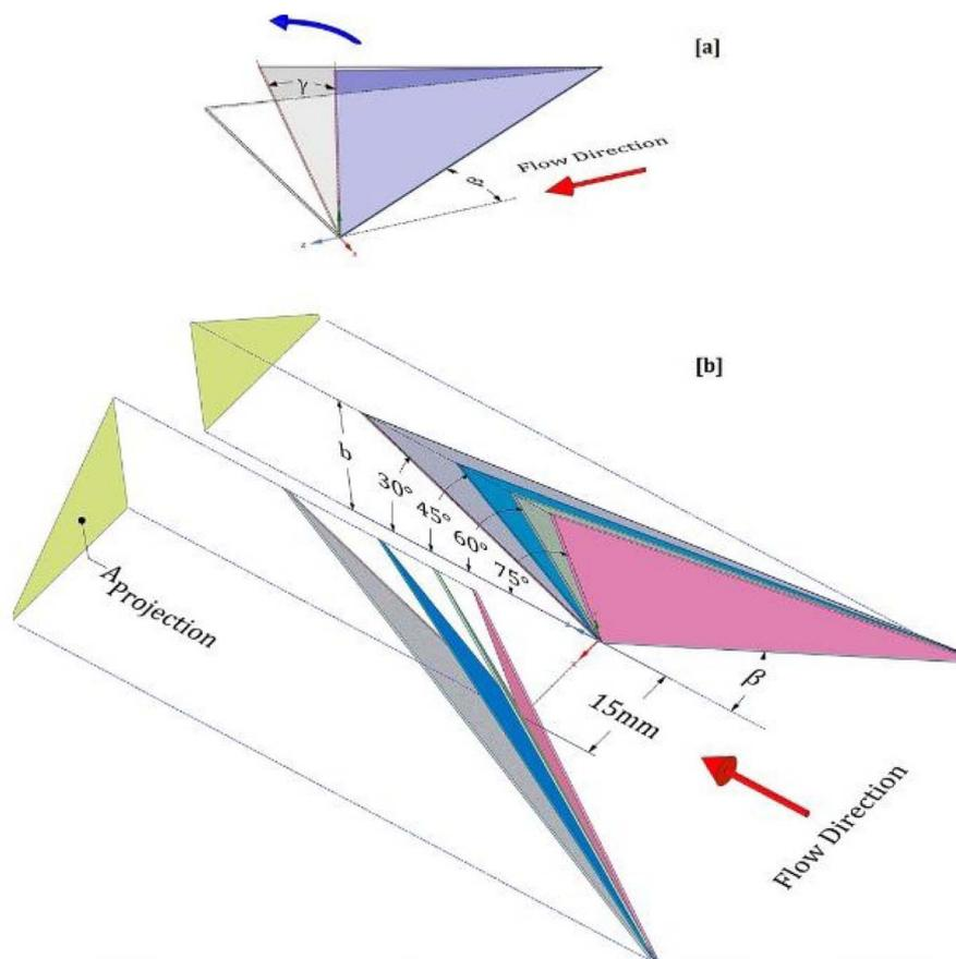
Fig. 12 Schematic of inclined DW. (a) Conventional approach. (b) Innovative approach. Reproduced with permission<sup>144</sup> copyright © 2024 Elsevier.
