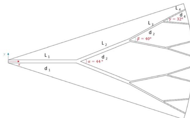
Fig. 3 The schematic geometry of the studied fractal microchannel. Reproduced with permission<sup>52</sup> copyright © 2020, Scientific Reports.
