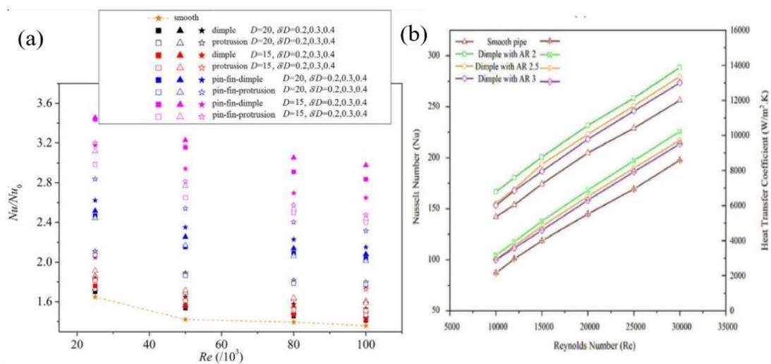
Fig. 14 Variation of Nusselt number and convective heat transfer coefficient with Reynolds number. (a) Summary of average  $Nu/Nu_0$  in each channel. Reproduced with permission<sup>167</sup> copyright © 2016 Elsevier. (b) Using 1%  $Al_2O_3$ /water nanofluid for different geometries. Reproduced with permission<sup>168</sup> copyright © 2023 Elsevier.
