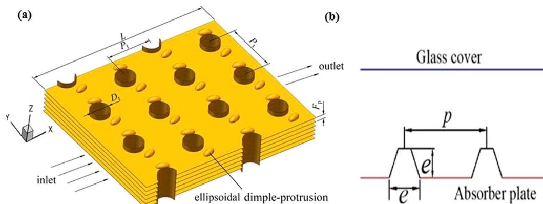
Fig. 16 Protrusion used in HX. (a) Elliptical dimple.<sup>180</sup> (b) Frustum-shaped. Reproduced with permission<sup>178</sup> copyright © 2023 International Solar Energy Society.
