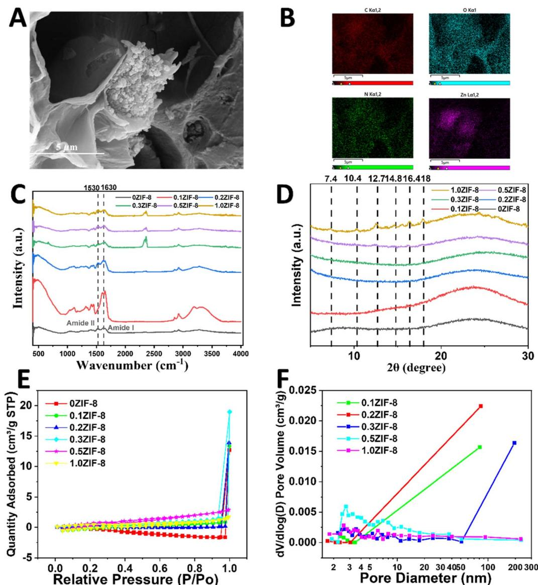
Fig. 3 (A) SEM photo of 0.3ZIF-8. (B) EDS mapping photos of 0.3ZIF-8 with four elements (C, O, N, Zn). (C) FTIR curves of HPHG. (D) XRD curves of HPHG. (E)  $\text{N}_2$  adsorption–desorption isotherm curves. (F) DFT pore size distribution of HPHG.
