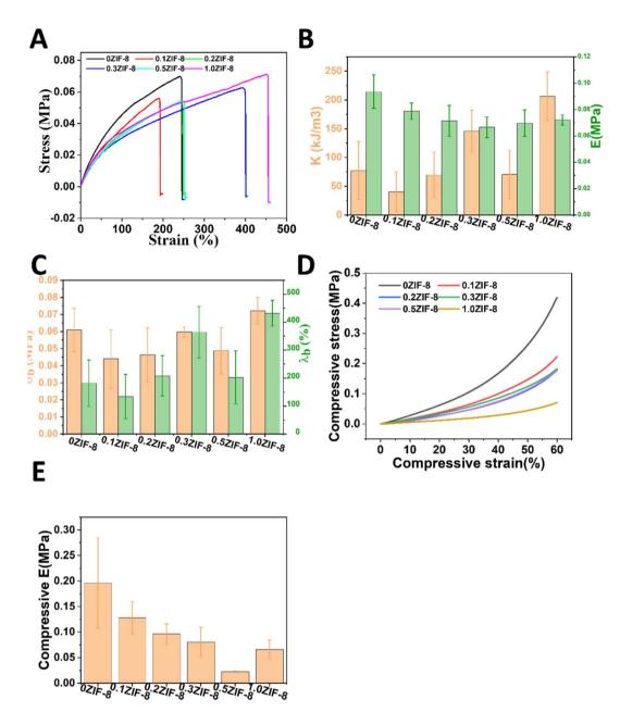
Fig. 5 (A) Typical tensile curves of HPHG. (B) Tensile strength ( $\sigma_b$ ) and elongation at break ( $\lambda_b$ ) of HPHA. (C) Toughness (K), (D) fracture energy ( $\Gamma$ ) of HPHG, and (E) compressive moduli.
