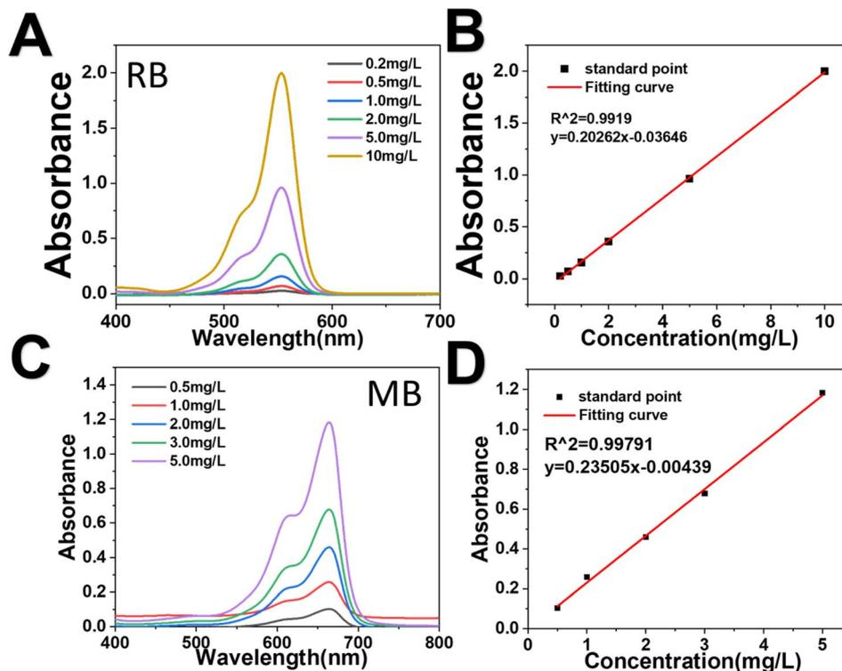
Fig. 6 Adsorption kinetics of RB and MB adsorbed by HPHG. (A and B) Standard concentration curve of RB. (C and D) Standard concentration curve of MB.
