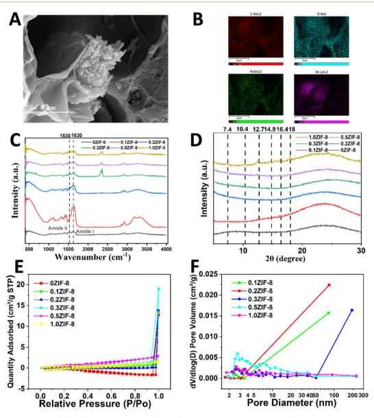
Fig. 3 (A) SEM photo of 0.3ZIF-8. (B) EDS mapping photos of 0.3ZIF-8 with four elements (C, O, N, Zn). (C) FTIR curves of HPHA. (D) XRD curves of HPHA. (E) N<sub>2</sub> adsorption-desorption isotherm curves. (F) DFT pore size distribution of HPHG.
