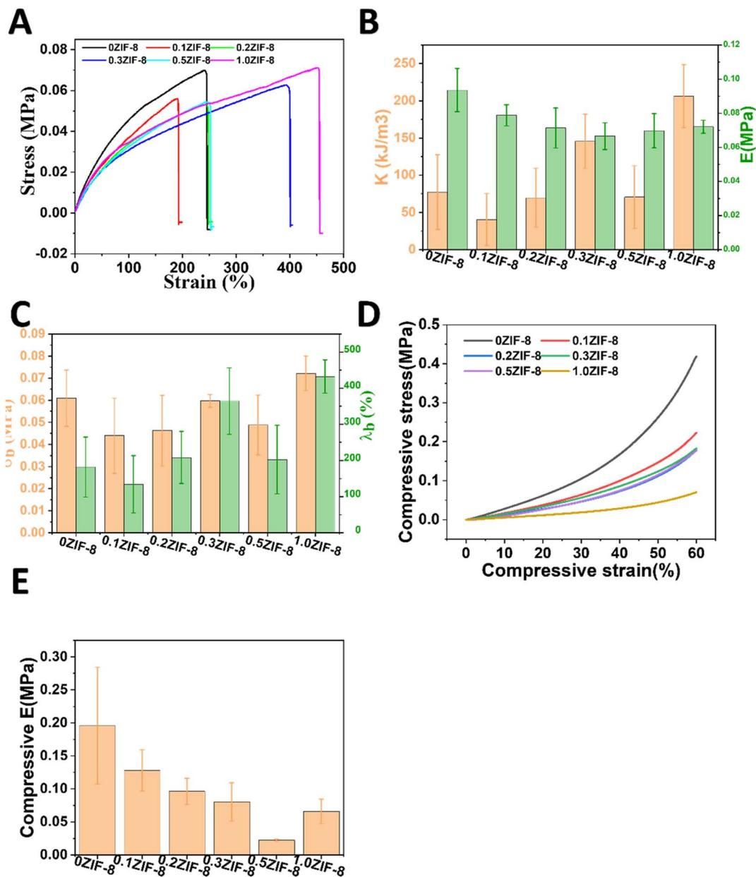
Fig. 5 (A) Typical tensile curves of HPHG. (B) Tensile strength ( $\sigma_b$ ) and elongation at break ( $\lambda_b$ ) of HPHA. (C) Toughness ( $K$ ), (D) fracture energy ( $I'$ ) of HPHG, and (E) compressive moduli.
