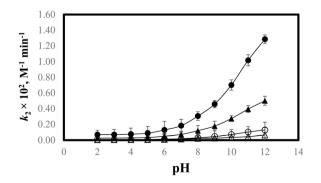
Fig. 9  $k_2$ -pH profile for the photodegradation of PD in the presence of RF in aerobic and anaerobic conditions using UV and visible irradiation sources: aerobic visible ( $\bullet$ ) and UV ( $\Delta$ ), anaerobic visible ( $\bigcirc$ ) and UV ( $\Delta$ ).
