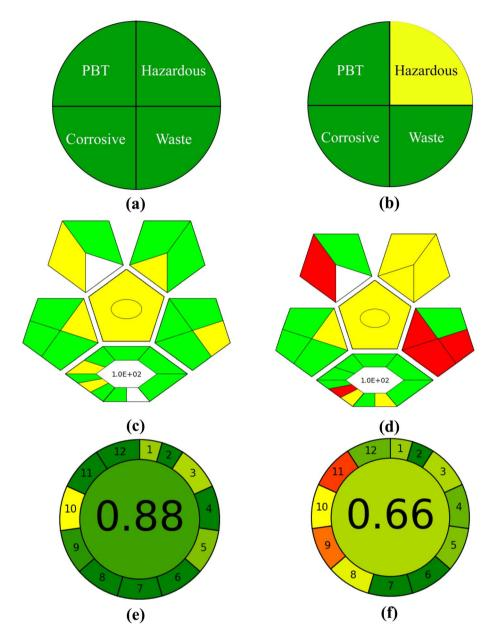
Fig. 6 NEMI (a and b), GAPI (c and d), and AGREE (e and f) analysis for the estimation of the developed UV-vis spectroscopic and HPLC methods.
