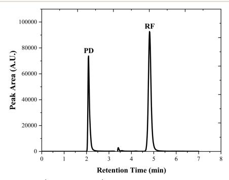
Fig. 5 Chromatograms of PD ( $1.00 \times 10^{-4}$  M) and RF ( $0.50 \times 10^{-4}$  M) in an aqueous solution (pH 3.50) at room temperature ( $25 \pm 2$  °C) and the retention time are 2.10 and 4.8 min for PD and RF, respectively.
