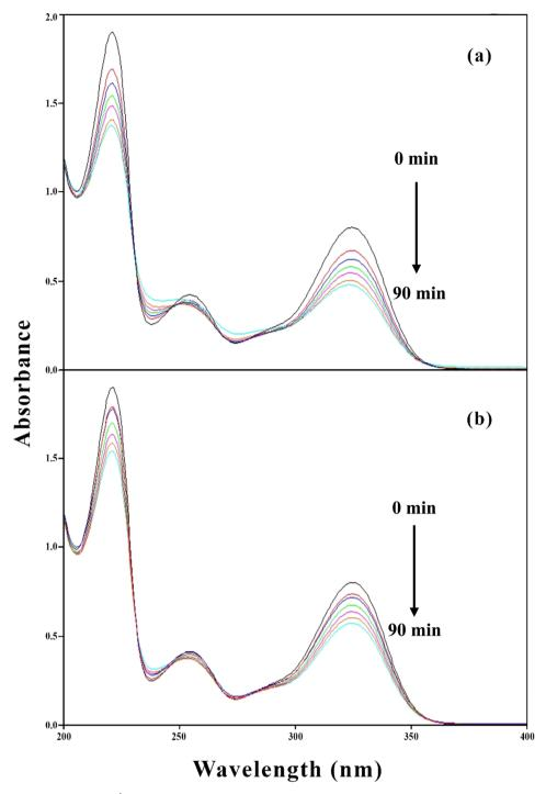
Fig. 7 Overlay spectra of PD ( $1.00 \times 10^{-4}$  M) on photolysis at pH 7.0 using UV (a) and visible irradiation (b) sources.
