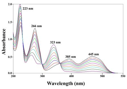
Fig. 4 Overlay absorption spectra of PD  $(0.10-0.90 \times 10^{-4} \text{ M})$  and RF  $(0.05-0.50 \times 10^{-4} \text{ M})$  at pH 7.0 of the synthetic mixture, where 223, 266, 385, 445 and 323 nm correspond to the absorption maxima of RF and PD, respectively.
