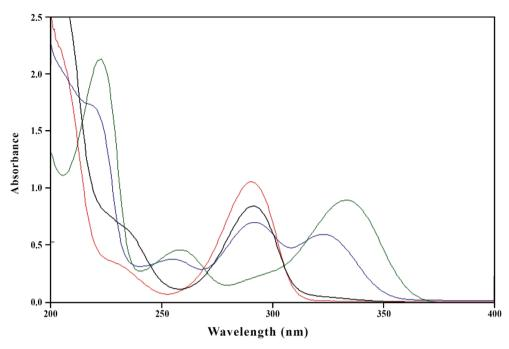
Fig. 3 Absorption spectra of PD (1.00 × 10<sup>-4</sup> M) in aqueous solution at pH 2.0 (red line), 4.5 (blue line), 7.0 (green line) and 9.0 (black line).
