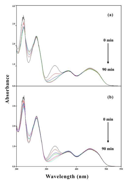
Fig. 8 Overlay spectra of PD ( $1.00 \times 10^{-4}$  M) in the presence of RF ( $5.00 \times 10^{-5}$  M) in visible (a) and UV (b) irradiation sources.
