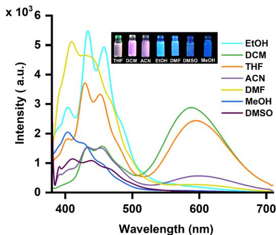
Fig. 1 Fluorimetric responses of HIP-Br (10  $\mu\text{M}$ ) in different organic solvents depicting intense orange emission in THF and DCM and relatively lower emissions in other polar protic and polar aprotic solvents ( $\lambda_{\text{ex}} = 350 \text{ nm}$ ,  $\lambda_{\text{em}} = 598 \text{ nm}$ ) [inset: images of HIP-Br under UV light in different solvents].
